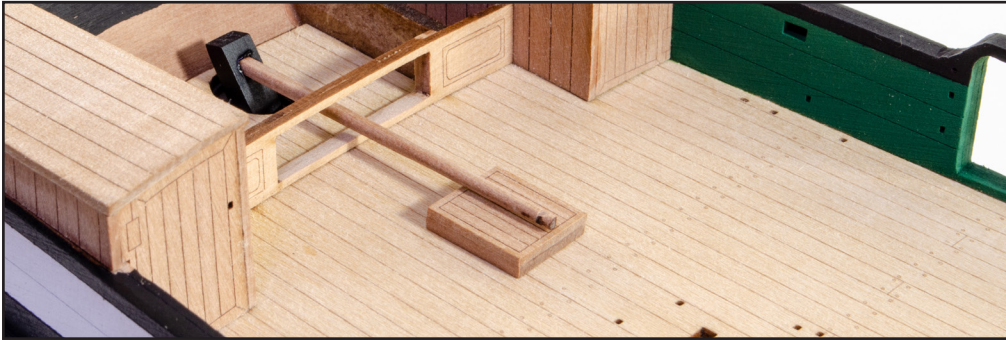
168. From the 1.5mm wood sheet, remove part #147 and sand so it's more rounded. Glue into position in the hole rudder hole, as shown.
