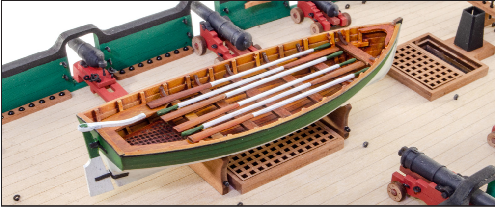
281. The boat will sit atop the cradles. You can glue if you wish but the ropes will hold this in place.
