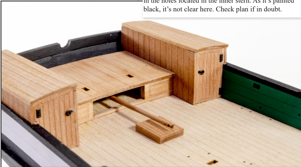
171. Add the 0.2mm hinge parts PE-32 to the cabin doors, as shown. Also add a door handle to each, using two PE-8 parts.
