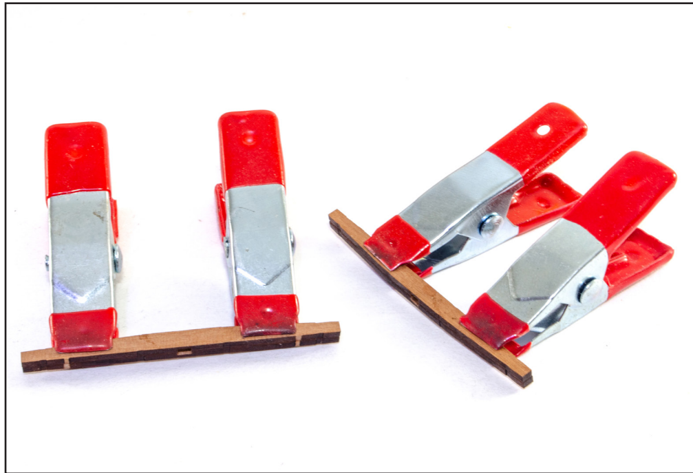
330. Before gluing the halves of the anchor stocks together, test fit the anchor shaft between them and if necessary, deepen the engraved area a little when the anchor sits comfortably within, remove the anchor and glue the stock halves together.
