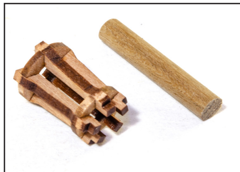
198. Cut a 22mm length of the 4mm diameter dowel. You can assemble the 1.5mm whelp parts and parts #103 and #104 around the dowel if you find it helps you with alignment. Don't glue the dowel into place yet though.
