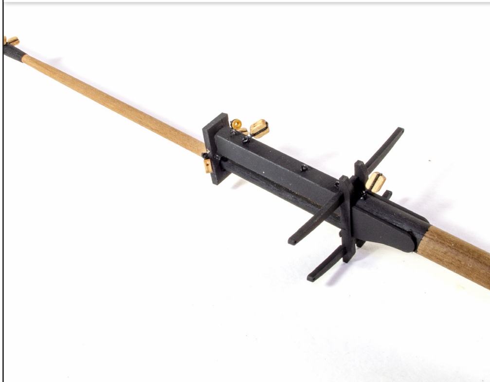
313. Paint this area black (or white) on each mast and add the various blocks as per plan. NOTE: Don't glue the upper two sets of blocks into place yet as you will need to fit a number of rigging lines to the mast before you secure those blocks.
