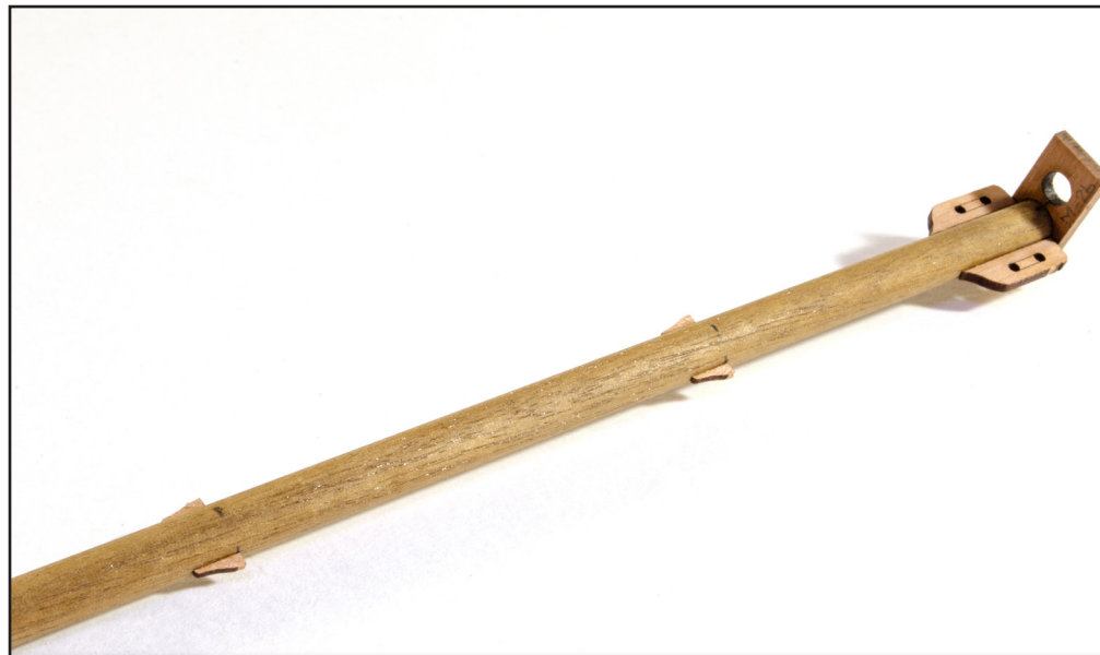
290. Start to fit out the larger dowel as shown. Use your plans to gauge the work needed to fit part M-2b as you can see here. This is angled. Fit the cleats as shown.
