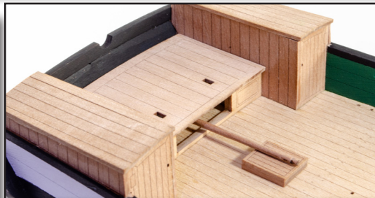
170. Glue into position as shown. You can now also glue part PE-23 into place, from the 0.4mm PE sheet, in the holes located in the inner stern. As it's painted black, it's not clear here. Check plan if in doubt.
