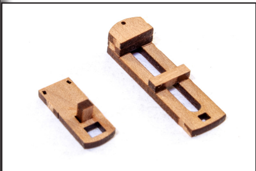
249. Glue part #129 into part #127 as seen on the left-hand side. Glue parts #128 together and then onto the engraved underside of #126. Now glue part #130 across the remaining engraved position.
