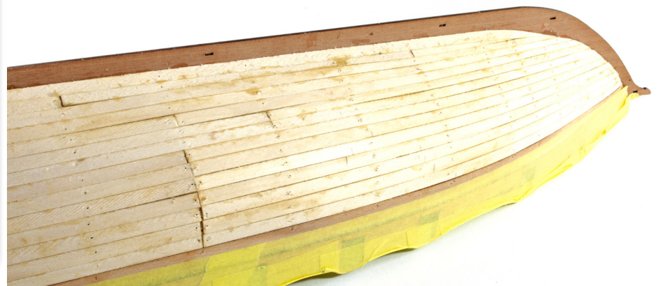
96. Continue to plank the hull, tapering as you go. You will find it beneficial to start tapering the planks from around the double bulkhead point as you progress. No tapering needs to be done at the stern.
