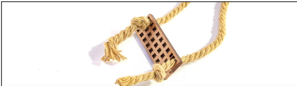
301. The last grate can now be fitted to the model. Use the thick hawse cable and either cut in half and thread from underside as shown or run it continuously from hole to hole. Glue the grate into place in the last frame on the deck.
