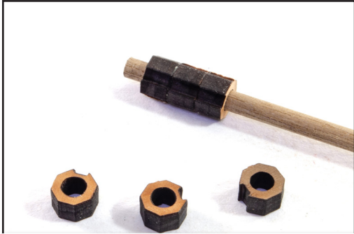
238. We now need to make two hand pumps. From the 4mm wood sheet, remove parts #157. Glue three of these together using a length of 3mm dowel as a guide.
