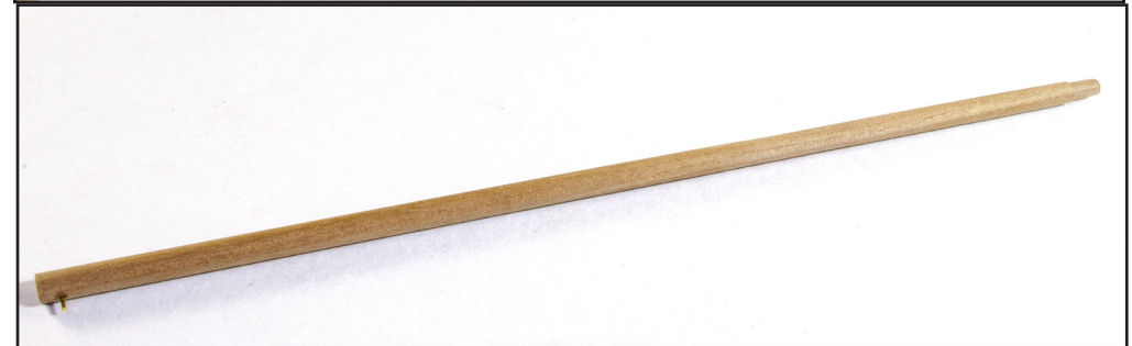
292. Shape the next largest section as shown. Notice I have inserted a small length of 1mm brass wire near the thicker end. This will be used to secure the part to the previous dowel.
