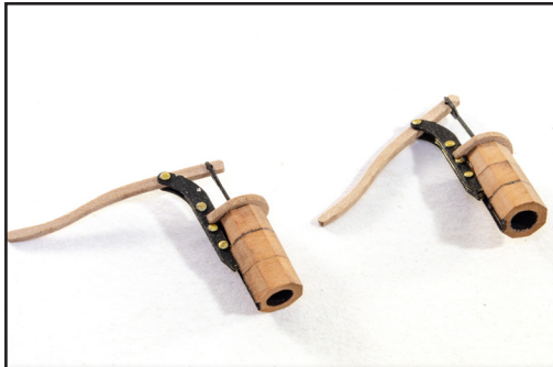
244. Slot the handle assembly into the pump body as shown, with the rod running down the centre of the drum and the handle secured to the metalwork using a brass pin, which can be glued and cut short.
