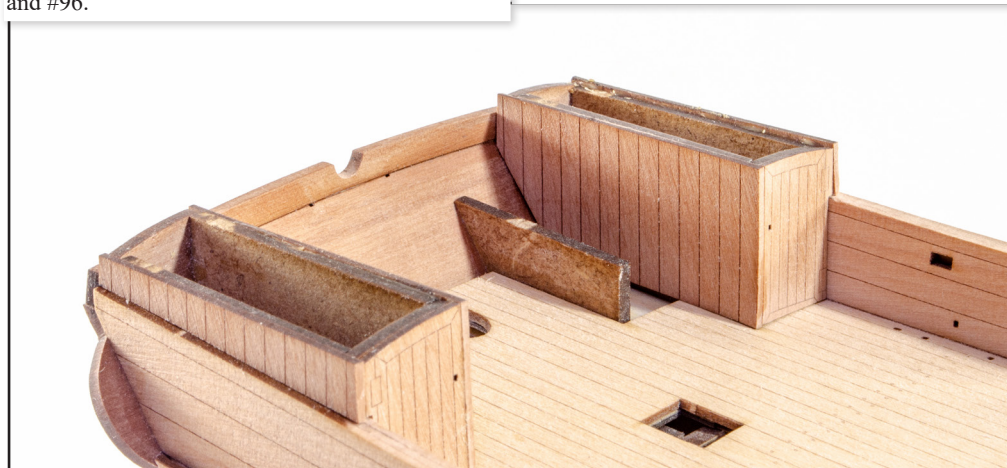
126. These fit on the outside edge of the MDF structure and will lay flush at the front and back. You will need to trim these to suit your own model.
