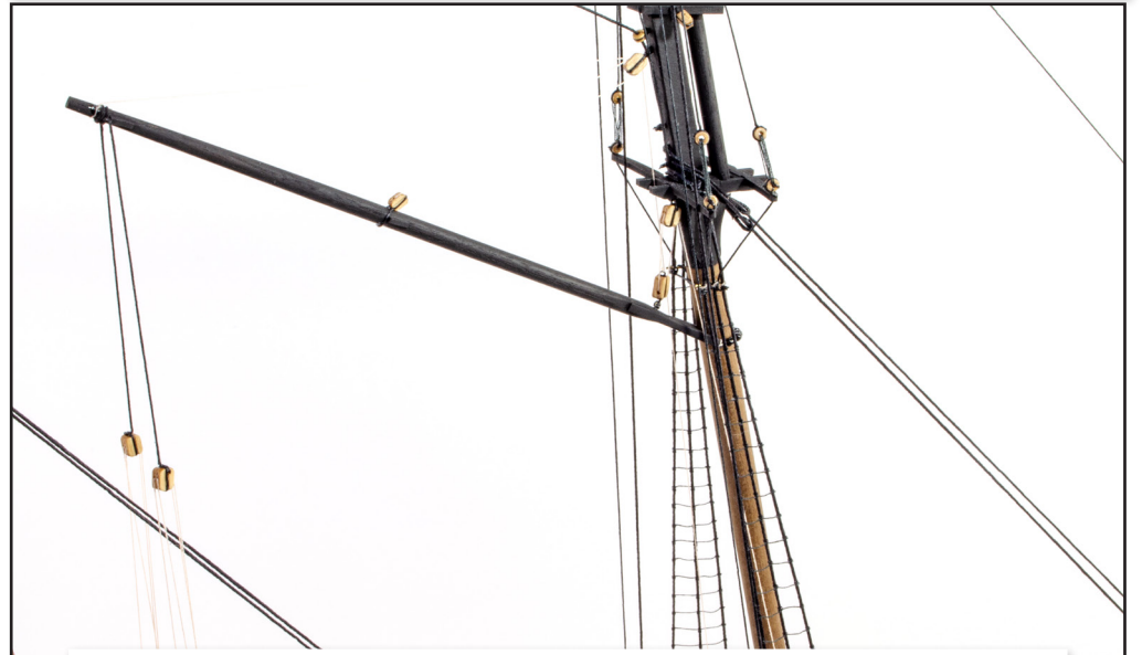
327. And here you see the fore gaff in place. This is rigged exactly the same as the main gaff.
