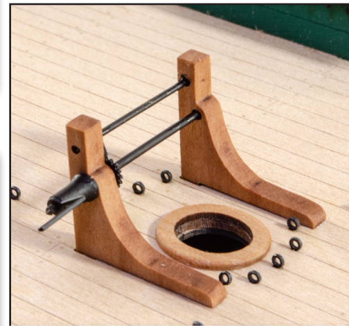
224. Cut the upper brass rod flush with the outside of the assembly. Slide/glue the winch drum to the lower rod and then the handle PE-22 as shown here and on plan. Cut the rod flush with the outside of the handle. Paint all metal/3D parts in black and then glue the winch to the deck.
