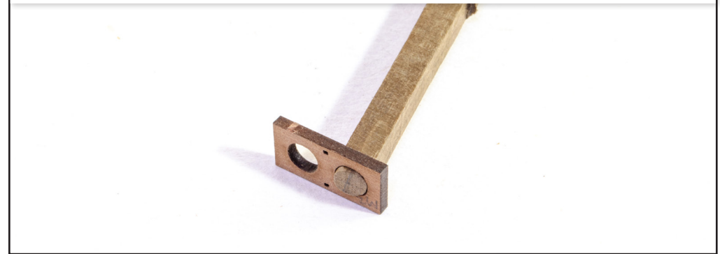
310. Here you can see the cap in situ before the top of the mast is sanded flush to the correct angle.
