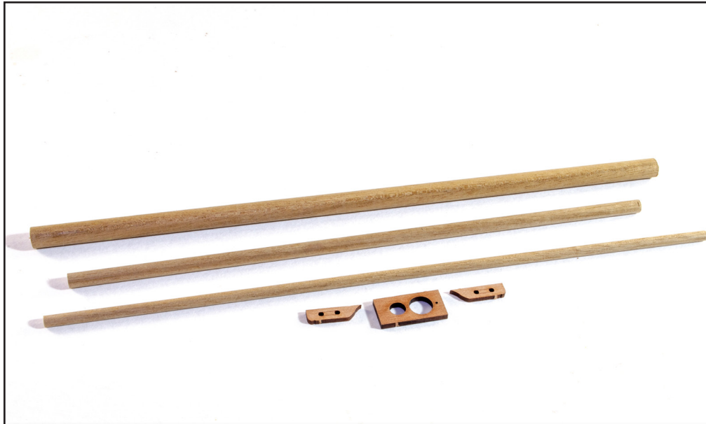
289. We can now build the bowsprit. Check your plans and cut the required dowel sections to length. From the 2mm wood sheet, remove part M-2b. From the 1.5mm wood sheet, remove parts M-13 and M-14.
