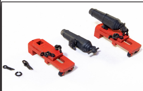
255. Take parts PE-15 and PE-16 from the 0.4mm PE sheet. Add the rings onto the brackets by springing the rings apart slightly and closing them up once in position. These can now be fitted to the carriages. Paint the carronade barrel F-1 in black and then glue to the carriage.
