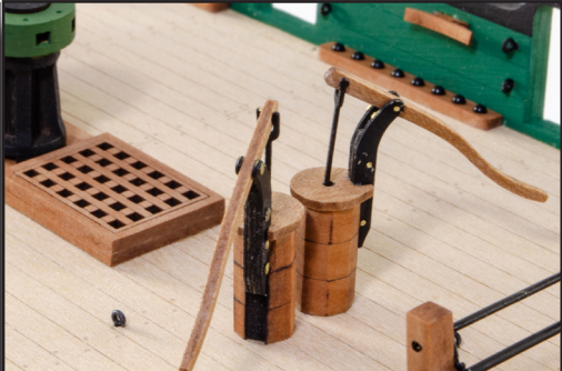
245. Use short lengths of 3mm dowel to mount the pumps to the deck as shown.
