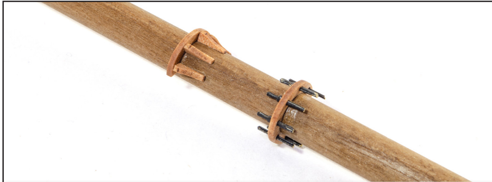
312. You can now fit the parts as shown here to the main mast. NOTE: We supply optional Mast Sail Rings (M-16) that you will need to slide onto the main mast before these are fitted. If you do opt to fit them, then use TEN of them. We supply far more as you could accidentally break them while removing laser char.
