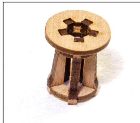
199. Glue part #105 atop the capstan body as shown.
