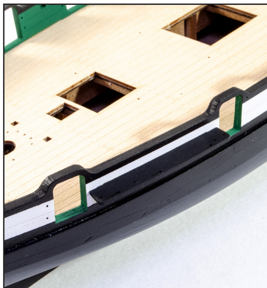
145. Paint these parts in black and glue parts #149 in place towards the bow, as shown.
