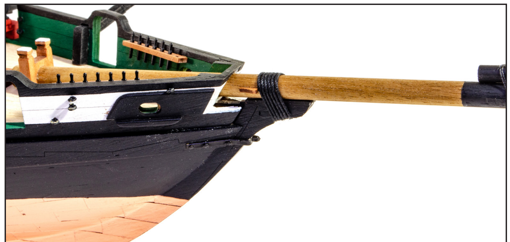
299. The bowsprit can now be fitted to the hull. Add the gammoning to lash the part to the hull, as shown here and plan.
