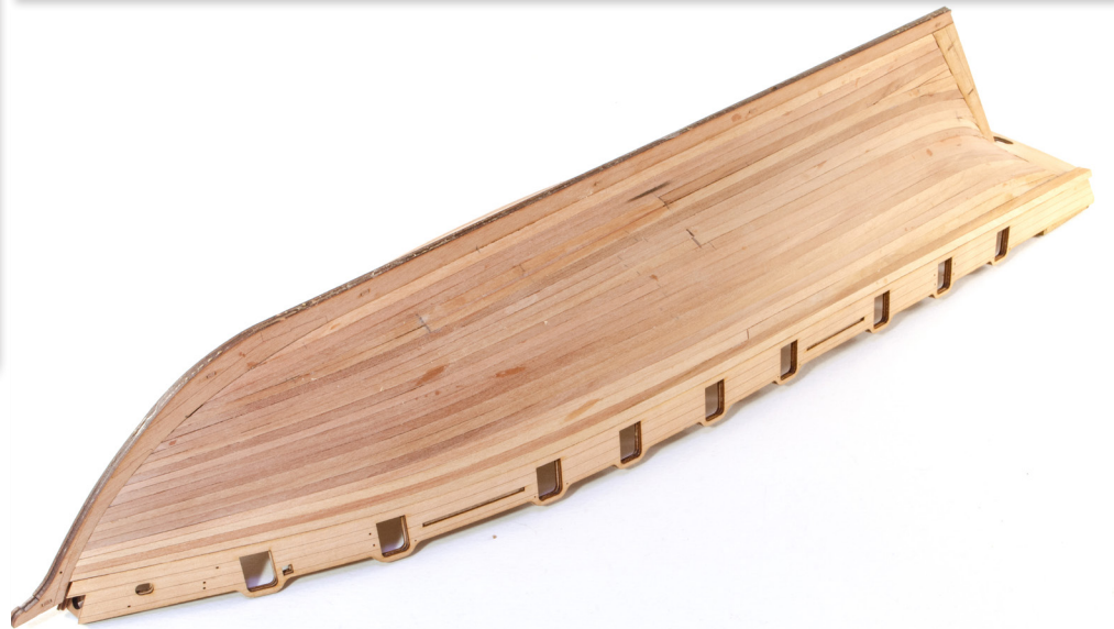
110. Now plank the hull again, using the pear wood strips, in the same manner as before. This photo shows you how the planks terminate at the part you just added, and also how they will look when they transition from the sides to the underside.
