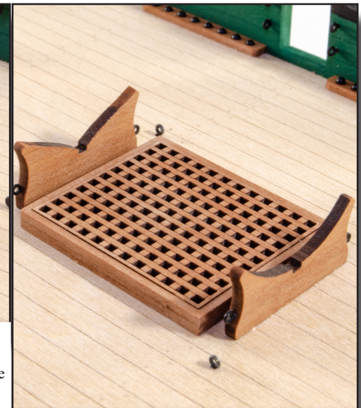
225. Take the boat cradles CT-14 and CT-15 from the 2mm wood sheet and drill/glue eyelets PE-8 into them as shown on the plan. Now glue into place as shown here, using your plan for spacing information.
