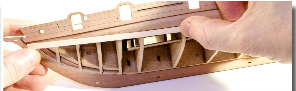
88. Sand the bulwarks flush with the stern of the hull.
