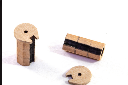
239. Sand off the char and then take part #108 from the 1mm wood sheet and glue as shown with the slot in the 4mm parts lining up with the notch in the new part.
