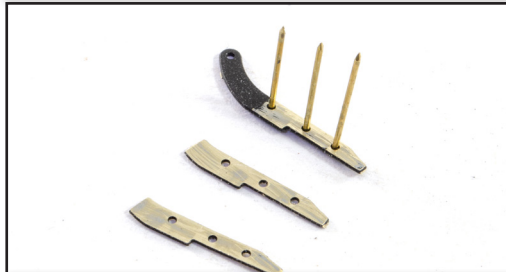
240. From the 0.4mm PE sheet, remove two parts PE-26 and PE-27. You will also need some brass pins. Slide three brass pins through the holes in PE-27.
