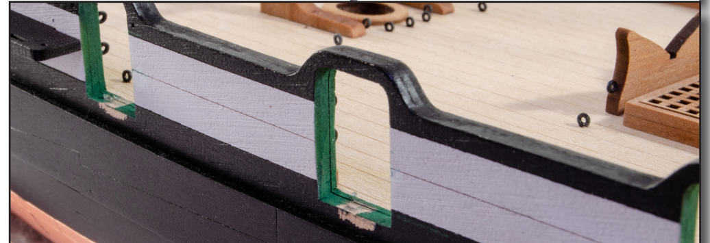
259. Select which gun ports you will install the carronades and remove a little paint from underneath each port and also from the centre lining of each gun port. We have chosen to replicate the gun layout on the plans, but you can choose whatever you wish. However, don't use the very forward port as that wasn't used on the actual ship.
