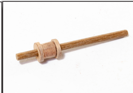
229. Slide the 4mm part onto the dowel, glued and sandwiched in between parts #107. The dowel has been left oversized at this point, to help with assembly.
