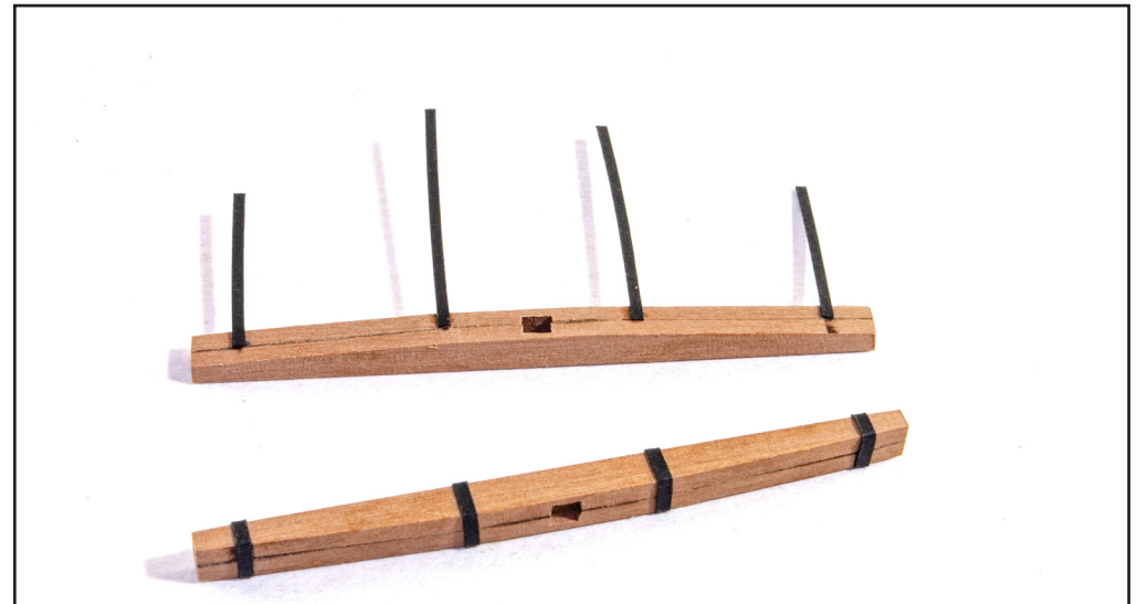
331. Cut thin strips of black cartridge paper and glue into place as shown.
