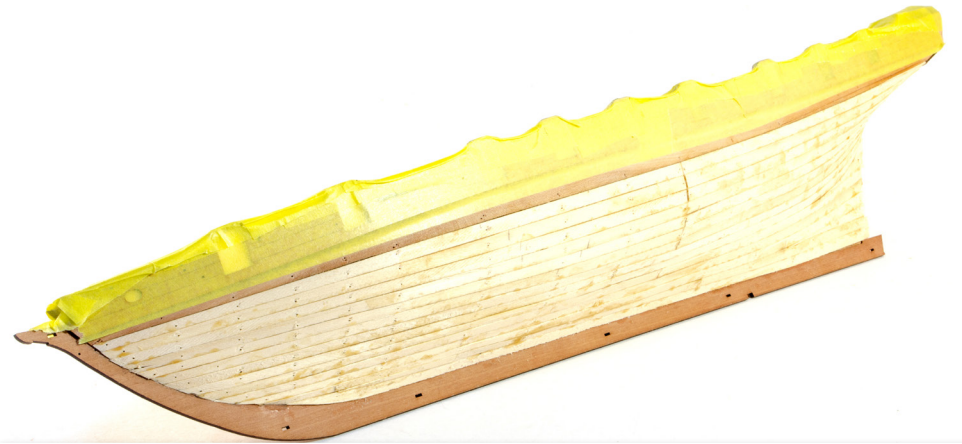
97. The hull is now fully planked. Use scrap planks to fill in any gaps you may have at the stern (or anywhere!).
