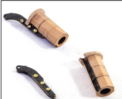
242. Cut the brass pins short and glue the assemblies into place on the wooden drums. You will see the metal part is shaped so it partially sits atop the wooden drums.
