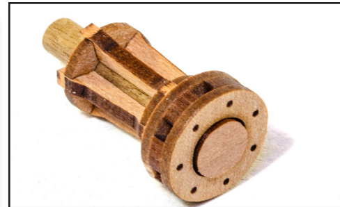
201. ... followed by part #106. Now glue the dowel into place so that the top of it sits about 1mm under the surface of the previous part. When dry, glue part #136 on top of the dowel. This should protrude about 0.5mm above the top of the capstan.
