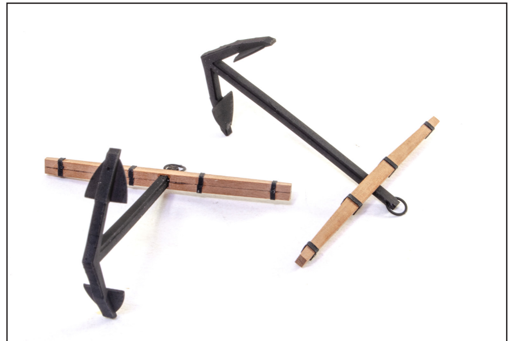
332. Paint the anchor black and then glue it into the stock. Finally, remove the anchor rings PE-7 from the 0.6mm PE sheet. Twist these slightly to open then, then slide into the hole in the anchor before twisting the part closed again.
