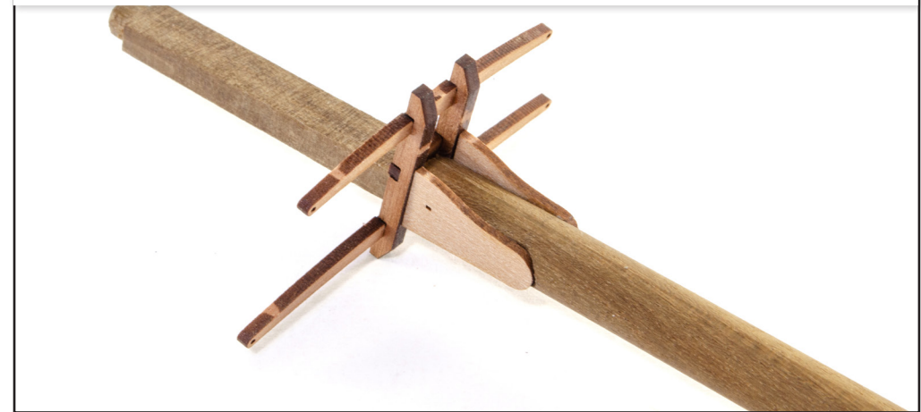
311. Now glue the cross tree into place, taking into account the angle to the mast. ALWAYS check your plans when shaping or fitting anything to do with the masts.
