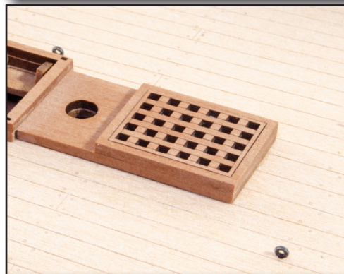
196. Now glue the grate #144c into place.
