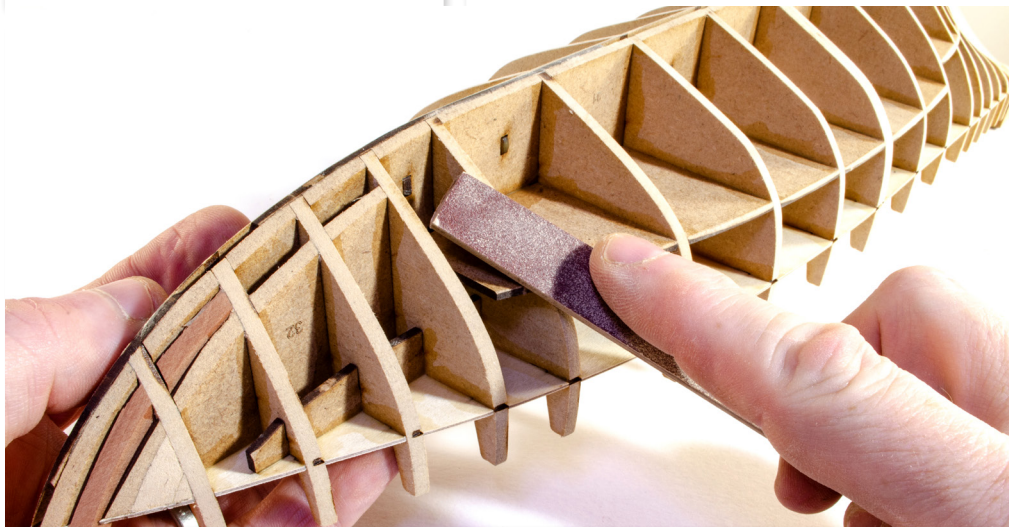
64. Before you can plank the hull, it needs to be prepared. This process of sanding the frames is called 'fairing'. Sand the bulkheads so that the shape of the frames 'flows' and sitting a plank along its length will show a maximum contact area between plank and bulkhead. A good indicator that you are fairing correctly is when most/all of the bulkhead char is gone. Use a sanding stick or similar to fair the hull.
