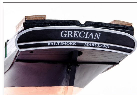
164. This can now be painted white and fitted to the stern as shown. Use the decal sheet to add the details as shown. We have supplied options for you in terms of colour and home port decal. We suggest the decals are added to the surface once it has been glossed. This will provide better adhesion.
