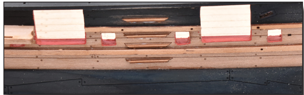
75. The outer hull side steps can now be fitted, These are on the 0.6mm wood sheet, 41 are the lower parts and 42 are the upper parts. The step positions are engraved on the hull sides, so glue in place to these positions using a small amount of PVA wood glue, and tweezers for positioning.
