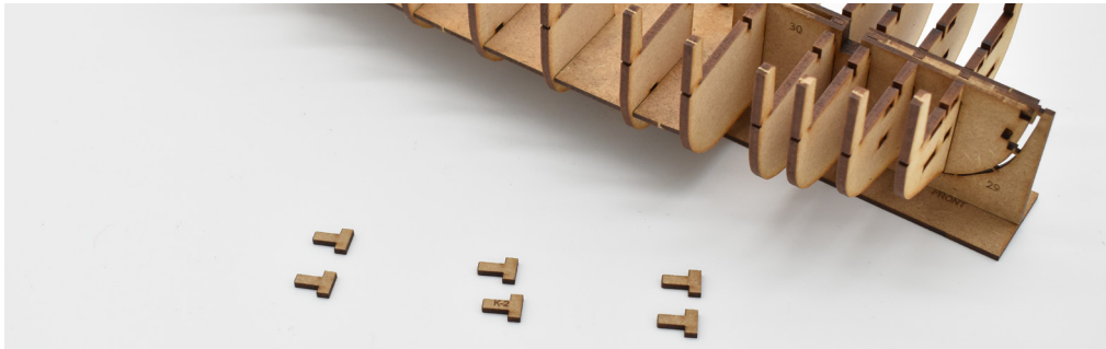
11. Remove the lower deck securing keys (K-2) and slot and glue into place on bulkheads 6, 8, 10 and 12. These will ensure the lower deck is locked into place.
