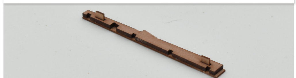
40. Make up the stern/rudder post assembly using part 152 at the core, and parts 94 for the outer rabbet parts. Glue and peg (using 92) the parts together and clamp until set, as shown.
