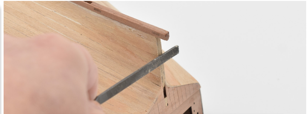
39. File the outer edges of the stern so that the stern/rudder post assembly will fit flush.
