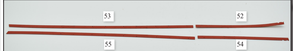
59. Remove the four spirketting patterns (54/55 - left and 52/53 - right) from the 0.8mm wood sheet (Above) Double check the fit, the top edges should be just below or on the lower edges of the gun ports, and the lower edge of the spirketting should touch the deck. Paint the parts red before fixing in place, this avoids the need to mask off the deck edges and ensures a nice clean line.
