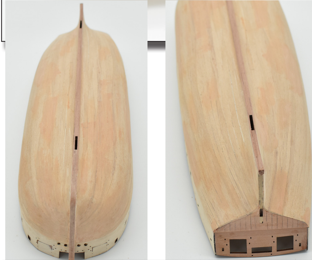
38. Second planking complete, sanded and filled. To get to this stage, several filling and sanding sessions were required. The filler used is a water based type, so it can be diluted and thinned, so it is able to flow into every gap. Before the sanding and filling process started, the engraved upper bulwark patterns were removed and the areas not to be painted white will be masked off.
