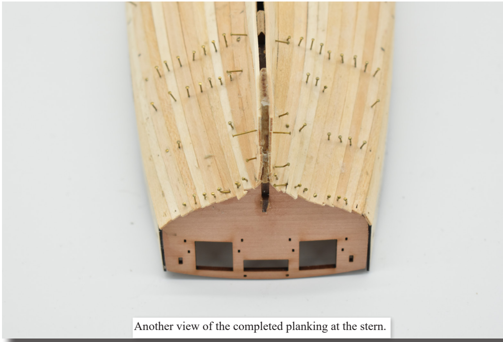
Pins removed and hull sanded and the stern planks trimmed flush with the stern board.
