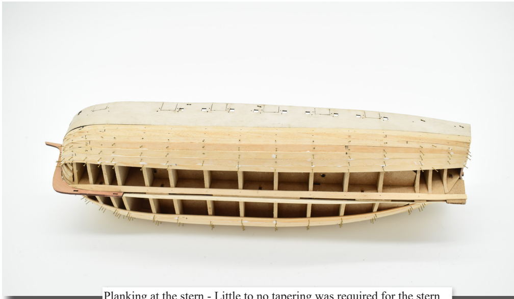
Planking at the stern - Little to no tapering was required for the stern
