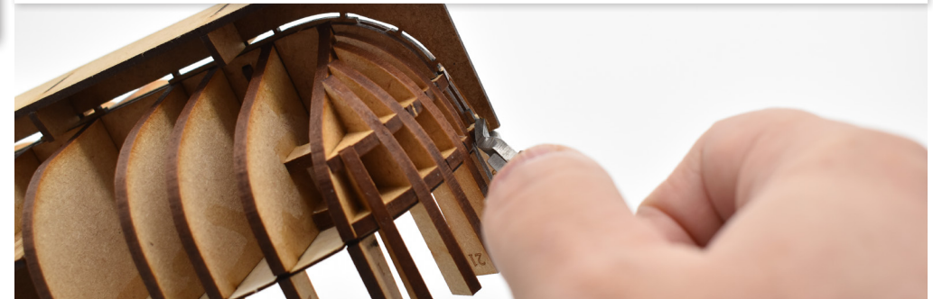
21. The hull assembly will now be very strong. It is now time to remove the keel from its spacing frame. Carefully remove the retaining tabs as shown, followed by filing any remaining bulges from the tabs on the keel flush.
