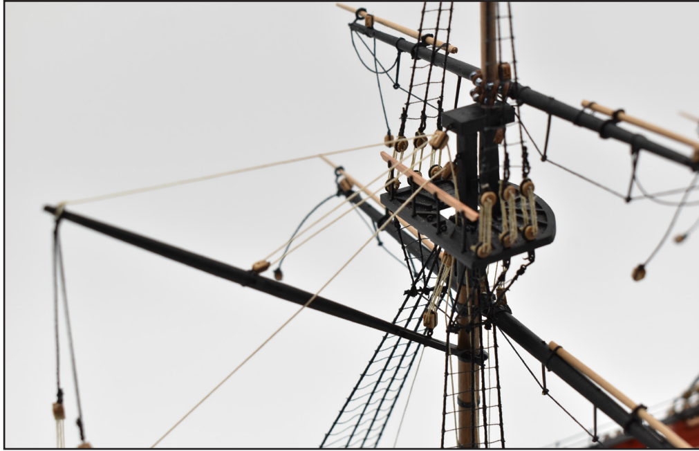
115, The 'Collar and Mouse arrangement as shown on Plan Sheet 10, for the mast stays.
