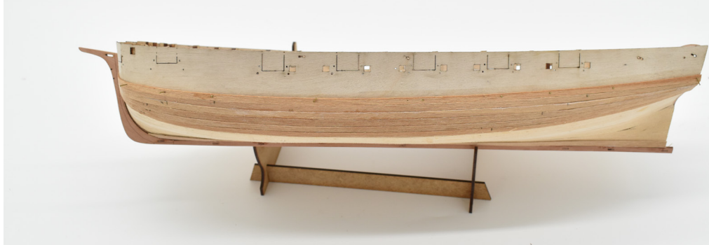
As with the first planking, the planks require tapering at the front (as shown above) Below - The first 4 planks laid.
