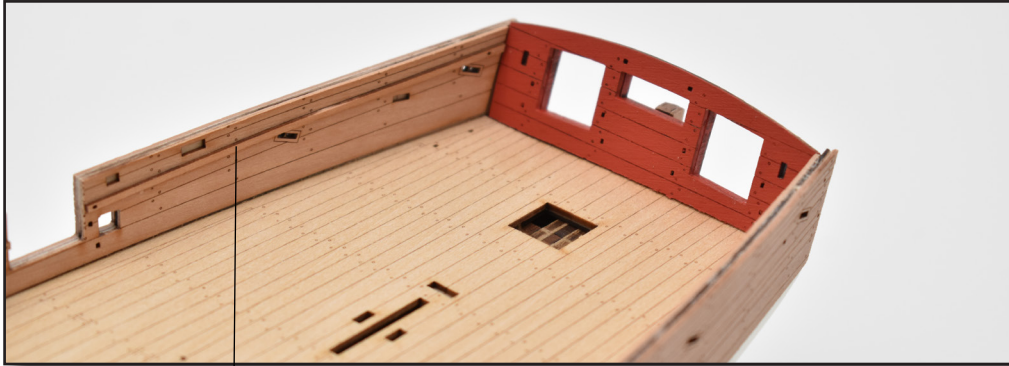
58. The inner bulwarks can be painted red at this point. Cover the outer bulwarks with masking tape, to help stop paint seepage to the outer face. If you are unsure of painting neat, also mask the deck edges. The prototype was brush painted. The paint doesn't need to go all the way to the bottom, as the spirketting will cover this. Make sure all of the inner edges of the oar and gun ports are covered in red. Two to three coats should suffice.
