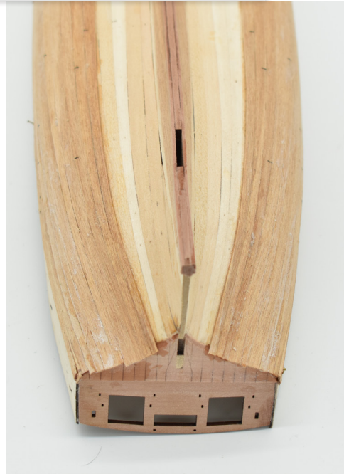
Progress of second planking. The planks at the bow will require severe tapering.
