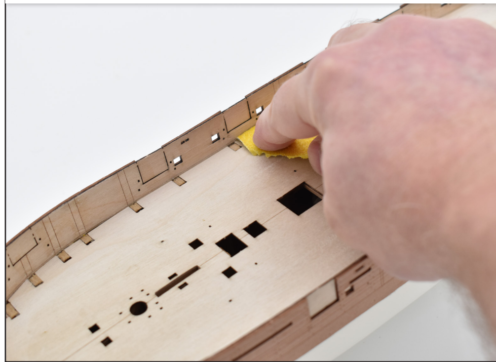
50. Remove all bulkhead tabs above deck level by carefully bending and twisting with a pair of pliers or similar. Once removed, sand any remaining stubs flush with the deck.
