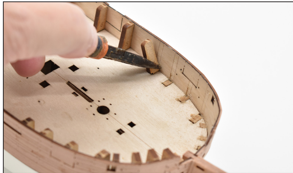
50. Remove all bulkhead tabs above deck level by carefully bending and twisting with a pair of pliers or similar. Once removed, sand any remaining stubs flush with the deck.
