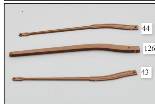
93. Using PVA wood glue (sparingly), glue the two outer parts (43 and 44) to the core tiller arm (126). Insert a brass pin into the holes at each end of the tiller arm to help keep it aligned. When the glue has set, either remove the pins or snip them off flush with the surface. Finally, insert and glue the arm into the rudder.
