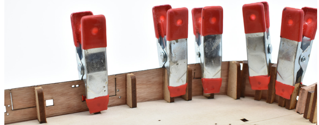
25. The two bulwark 0.8mm ply patterns can now be added (36 - left/port and 37 - right/starboard). The engraved vertical lines should follow quite closely the bulkhead positions, and the lowest horizontal line should be placed at the top edge of the false deck position. We recommend that these parts are dry fitted several times to ensure correct positioning. Each engraved line may not be a perfect match to each bulkhead tab due to slight variations in the sanding of the bulkheads process. However, if they more or less match from front to back, this will be fine. Always watch for the lower deck line along the deck edges.
