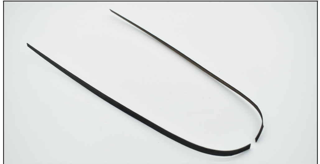
62. The wales can now be painted black before finally fixing into position on the hull.
