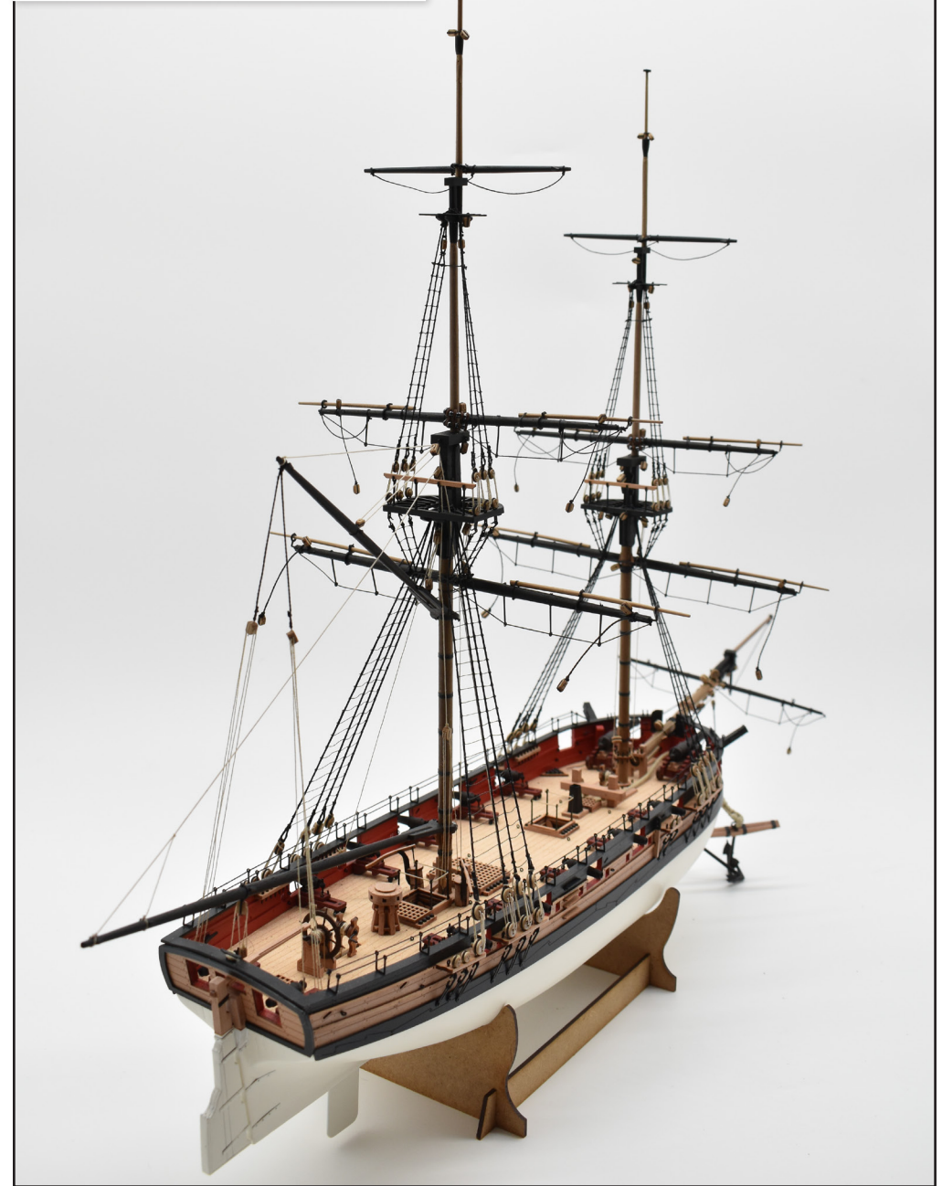
113. Once the shrouds and ratlines have been rigged, add the yards. The gaff and boom can be fully rigged at this time.
