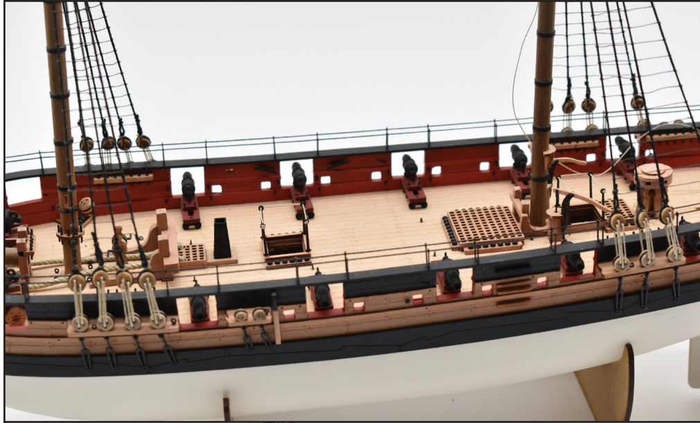
113. Once the shrouds and ratlines have been rigged, add the yards. The gaff and boom can be fully rigged at this time.
