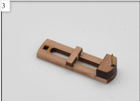
Pin and glue the front chock (178) into position as shown, and then snip off the excess pin.
