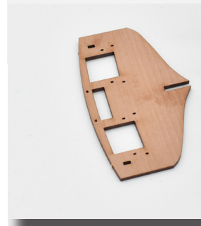
13. Slot and glue bulkhead 153, the rear most bulkhead, in place
