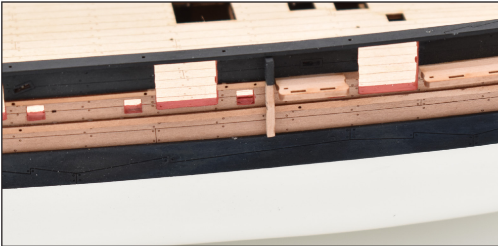
74. The Chess Trees (146 - Right and 147 - Left) can now be painted and added to each side of the hull. The positions are engraved onto the hull sides. Use either cyano gel or PVA wood glue to fix in place.
