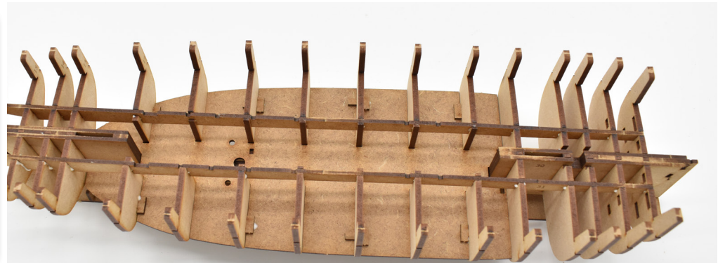
11. Remove the lower deck securing keys (K-2) and slot and glue into place on bulkheads 6, 8, 10 and 12. These will ensure the lower deck is locked into place.
