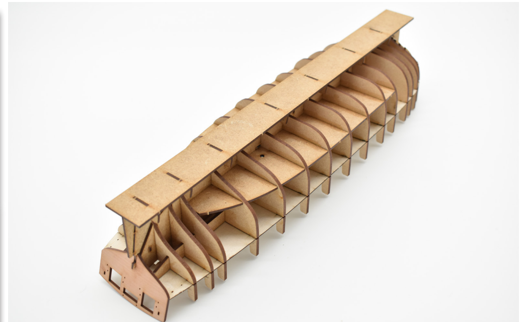
21. The hull assembly will now be very strong. It is now time to remove the keel from its spacing frame. Carefully remove the retaining tabs as shown, followed by filing any remaining bulges from the tabs on the keel flush.
