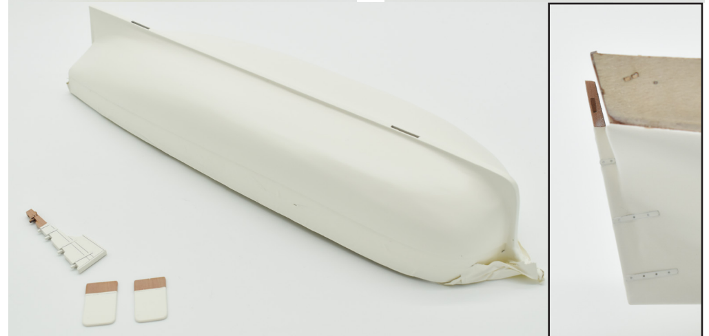
47. The hull will require several coats with filling and sanding in-between most coats. Standard matt white spray paint was used for this model. Before adding the last two or three coats and when final filing/sanding is complete, glue the rudder hinges (PE-6, PE-7 and PE-8) in place as shown on the inset picture.
