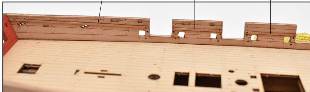
57. Using Plan Sheet 5 for placement, add the inner bulwark rails. For the prototype, PVA wood glue was used, and the rails clamped in place until the glue had cured.
