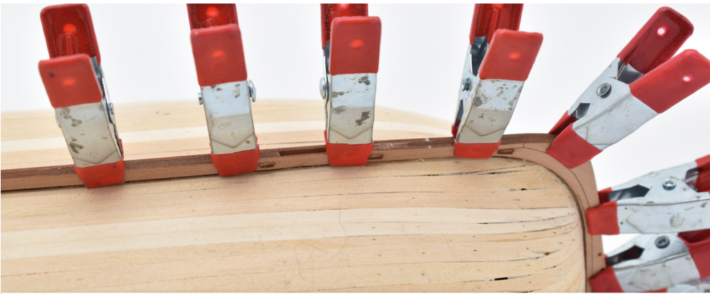
34. Add the lower keel outer facings (93). Use parts 92 to lock the parts in place and PVA wood glue to fix. Clamps are shown, securing the assembly until the glue has cured.
