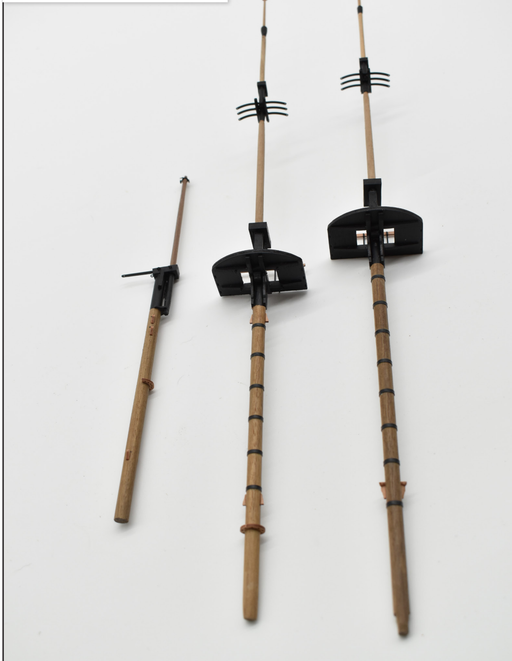
108. Fore and main mast complete, along with the bowsprit, using Plan Sheet 7 for the masts and Plan Sheet 8 for the bowsprit.
