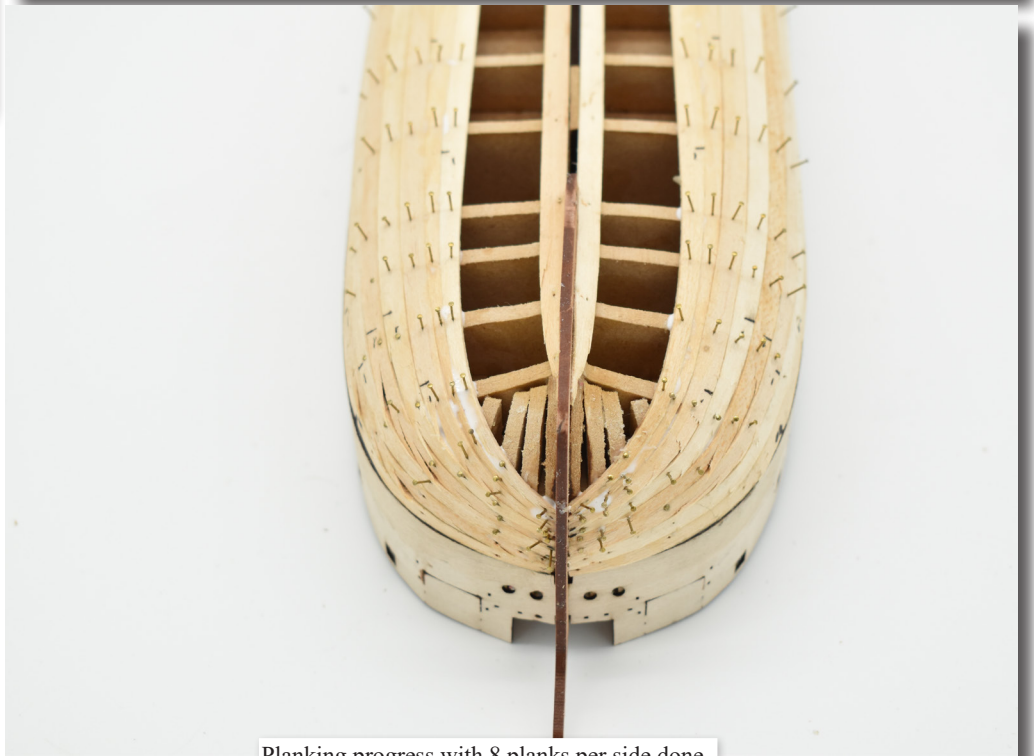
Planking progress with 8 planks per side done
