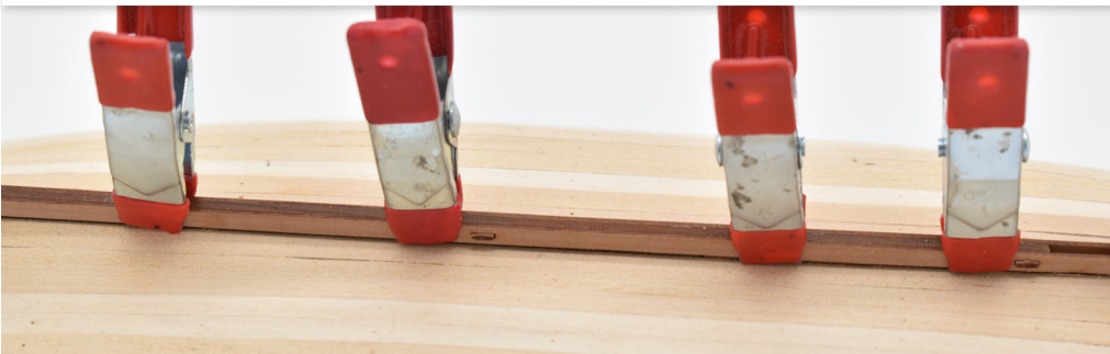
34. Add the lower keel outer facings (93). Use parts 92 to lock the parts in place and PVA wood glue to fix. Clamps are shown, securing the assembly until the glue has cured.
