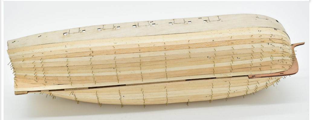
Planking almost complete. There will be a few 'stealers' required (triangular shaped filling planks) for the stern. as seen below with the completed planking.
