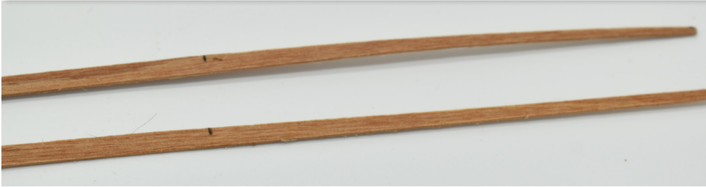
As with the first planking, the planks require tapering at the front (as shown above) Below - The first 4 planks laid.
