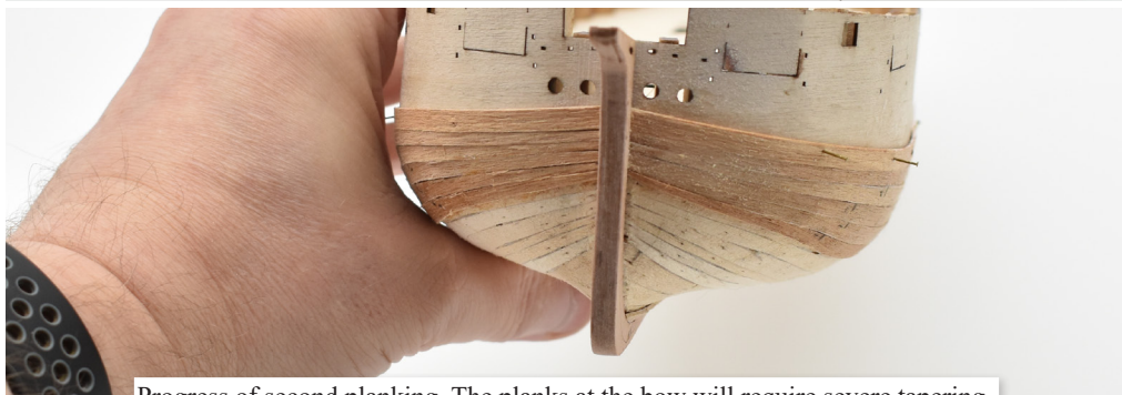
Progress of second planking. The planks at the bow will require severe tapering.
