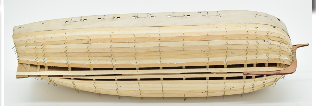
Planking almost complete. There will be a few 'stealers' required (triangular shaped filling planks) for the stern. as seen below with the completed planking.
