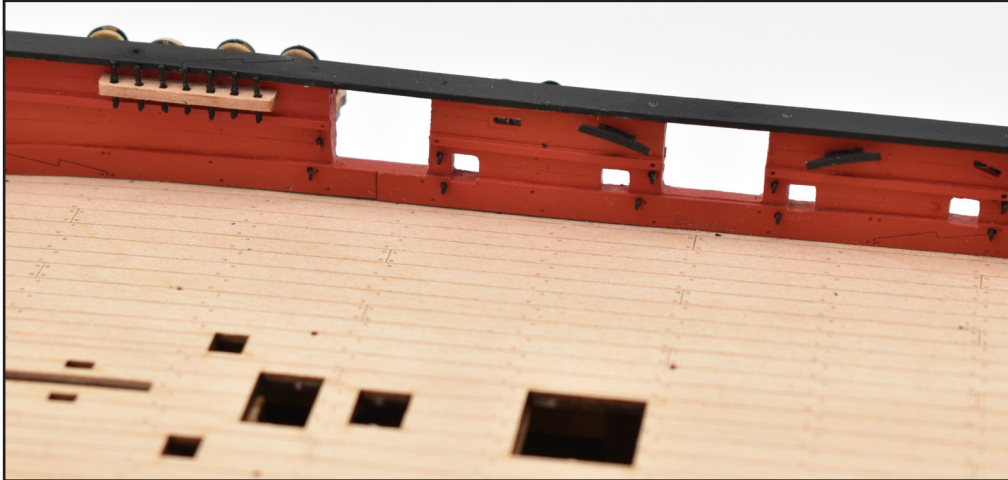
80. Using Plan Sheet 6 as reference, add all of the remaining outer eyebolts (PE-15), again, opening up each hole to ensure each eyebolt pushes all the way in when glued (using cyano gel)
