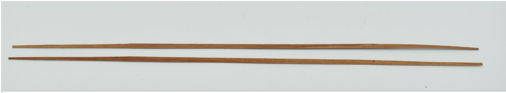
As with the first planking, the planks require tapering at the front (as shown above) Below - The first 4 planks laid.
