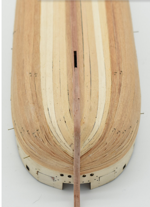
Progress of second planking. The planks at the bow will require severe tapering.
