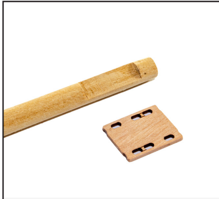
413. Using your plan as reference for dimensions, slightly taper the thickest dowel and then remove a section of the dowel into which this part M11 can be fitted. This part can be located on the 1mm wood sheet.
