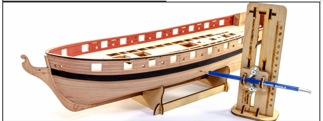
186. We need to now prepare the hull under the waterline before we can copper it. To do this, add a waterline to the hull, and make it a few millimetres below the actual waterline shown on plan. The reason for this is that we don't want any filler appearing above the actual waterline, later in the build.
