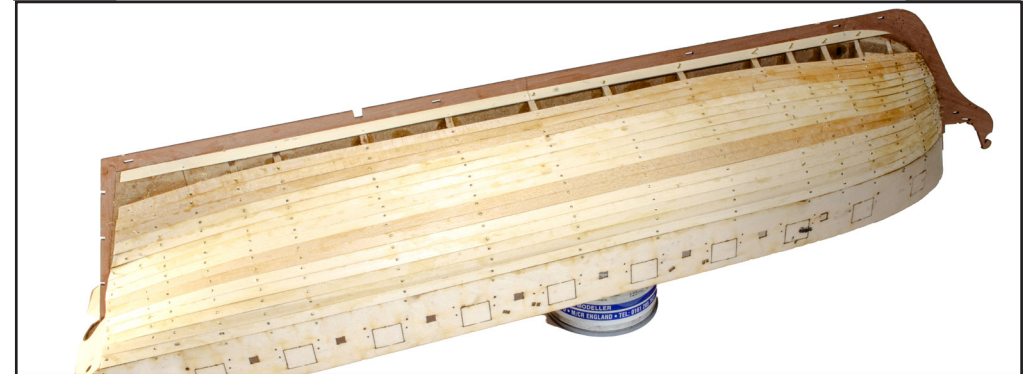
120. You will be able to run many planks down towards the lower keel, in the same way. You may also have your own preferred way of planking. As you approach the keel, you will need to add a plank along that edge. This is called the 'garboard plank'. Feel free to add this in two parts if you feel happier. When fitted, continue to plank down towards the garboard plank. If you have small gaps in your planking, then use scrap limewood to make 'stealers' and fill in those gaps.
