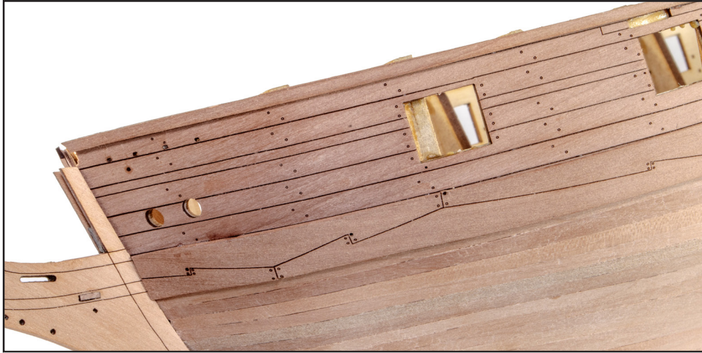
146. Glue these in place along the top side of each bulwark, along the top of the first engraved line down each part.
