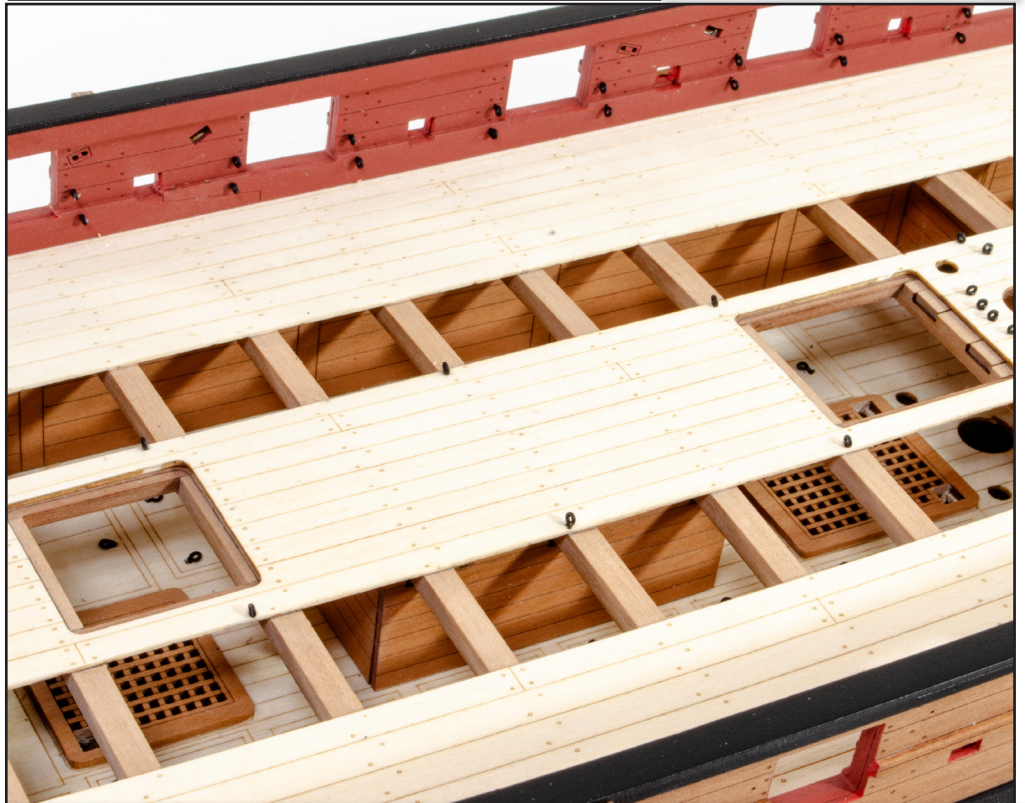
252. Following your plan sheet, you now need to install eyelets PE-14 from the 0.4mm PE sheet. There are four per gun port, including the inner stern ports, and also eyelets to add to the deck. Again, check your plans.
