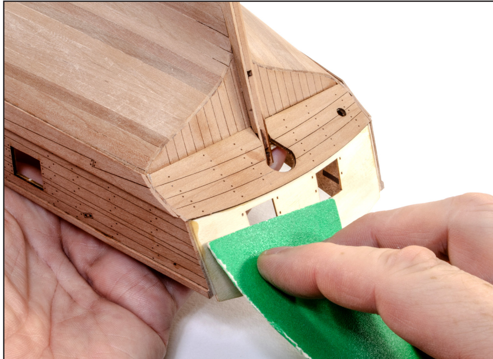
147. Use a piece of sandpaper to sand flush the bulwarks, wales and strips to the stern and stern counter areas.
