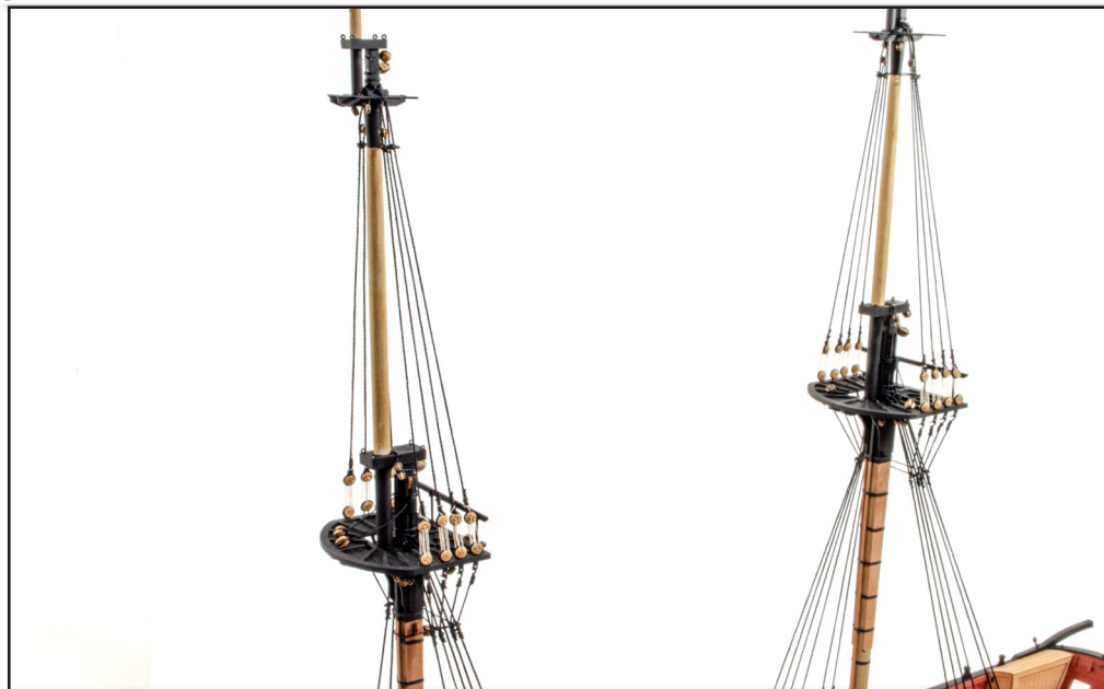
477. The deadeyes can now be rigged by adding the next set of shroud lines, in the same way as before.
