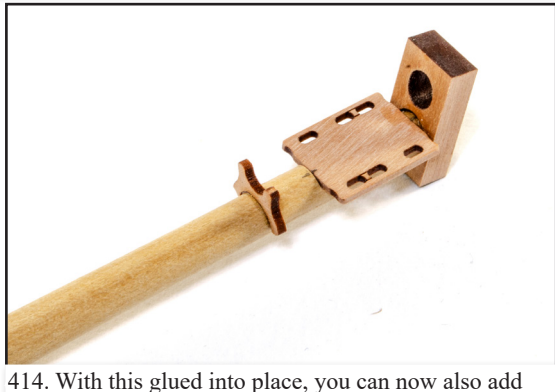
414. With this glued into place, you can now also add part M35. You WILL need to internally chamfer the holes on this part so it can attain the correct angle in relation to the dowel. ALWAYS check against your plans. From the 1mm wood sheet, remove part M12, and glue into place as shown, checking the position.
