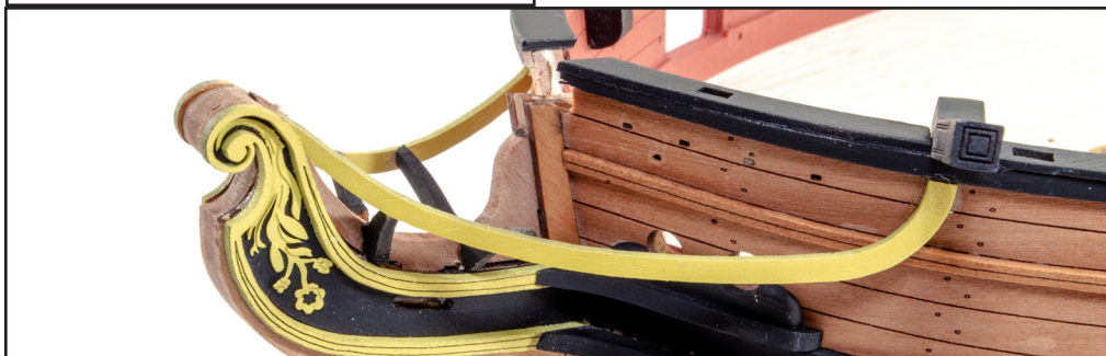
242. After sanding the 'v' parts as shown on plan, paint parts 147 in ochre and glue into place as shown here and on plan. These parts should sit flat against the 'v' parts for maximum contact.
