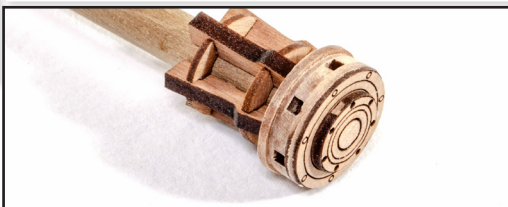
370. Glue the drum to the top of the capstan. Now cut the 6mm dowel so that it's 52mm long. Glue the dowel into the capstan so the top of the dowel is flush with the top of the drum. From the 0.8mm wood sheet, remove part 120. Glue this to the centre top of the capstan.
