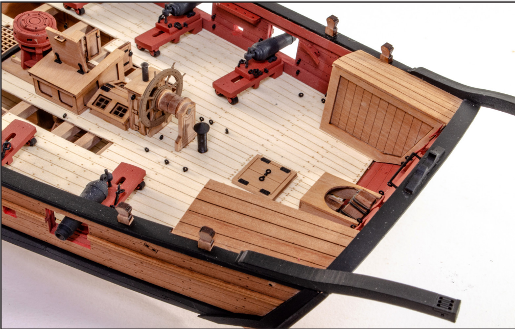
400. Here you see those timberheads installed on the rear gunwales.
