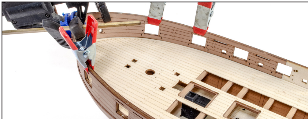
157. There is no need to soak the shorter forward bulwark parts here, but it is a good idea to push them into position and clamp them for 24hrs so the fibres relax, and it will make it easier to fit when gluing the parts.
