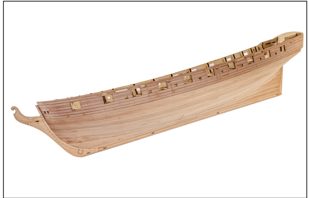
139. In the same manner as with the first layer of planks, use the pearwood planks to create a second layer. We suggest that you DON'T use pins for this layer as it will be seen when finished. For our prototypes, we use Gorilla Glue CA gel for controllability and predictability when applying. We use small dots about 2mm diameter and 2 or 3mm apart down each strip and slowly apply each one, making sure the wood is bonding as you progress.
