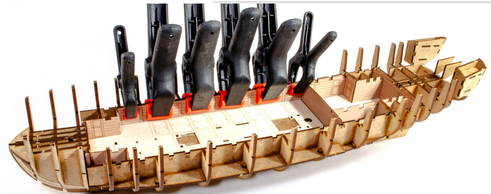
69. Glue them into place and clamp to stop the parts curling after glue is applied. Part 171 is the one you see being clamped in this photo, with part 170 on the opposite side.
