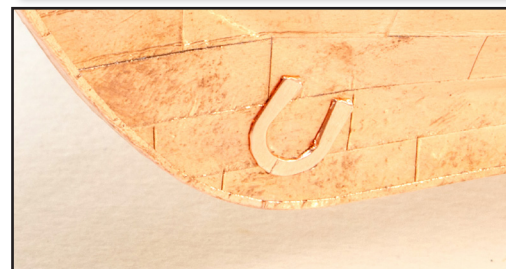
229. Cover these in copper tape (or paint copper) and glue into place as shown here. If you wish, you can use short brass pins to simulate rivets.
