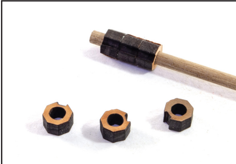
356. From the 3mm wood sheet, remove all parts 268. From these you will make the bodies for TWO pumps. Carefully glue them together whilst aligning them on a 3mm dowel length. Ensure the recessed sides are in alignment.
