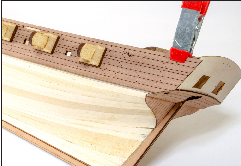
137. Now glue each bulwark onto the hull, pinning if necessary, and also clamping. Use those gunport jigs to ensure correct port alignment, but make sure you don't accidentally glue them in situ! Don't worry about any overhang at the rear. That will shortly be fixed. Leave these parts to thoroughly dry.
