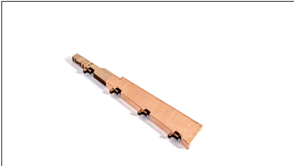
192. Now copper the rudder as you did with the hull. It's always better adding too much as it can be removed later.
