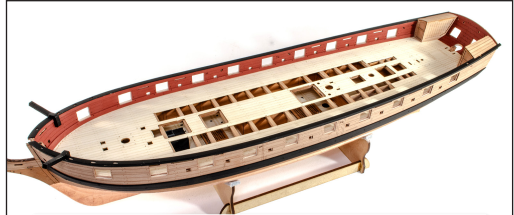
205. Now glue parts 93 to the top edge of the bulwark, so it's flush with the outer black rail.
