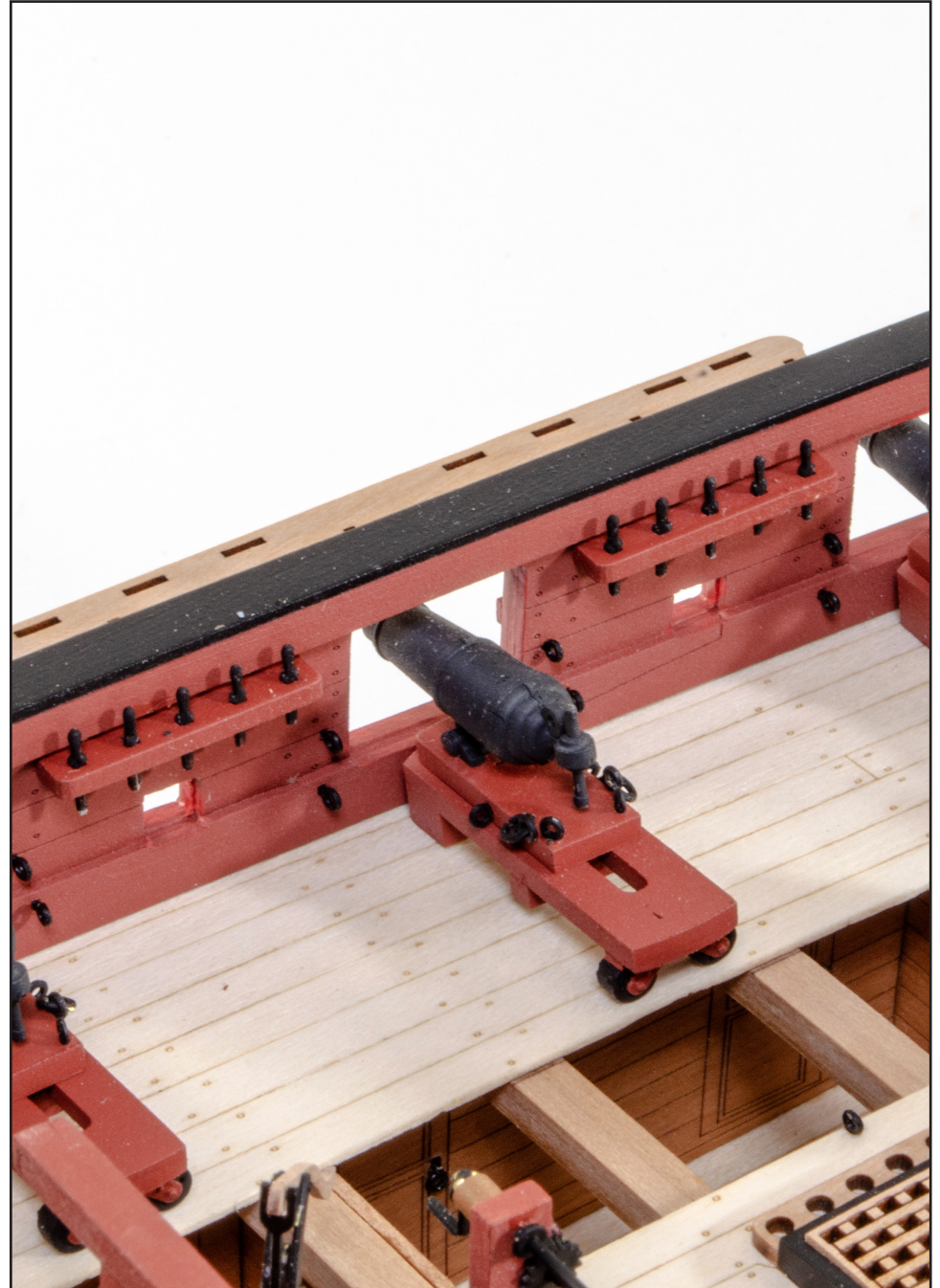
401. From the 0.6mm PE sheet, remove parts PE-54. Install these into all of the belaying pin racks.
