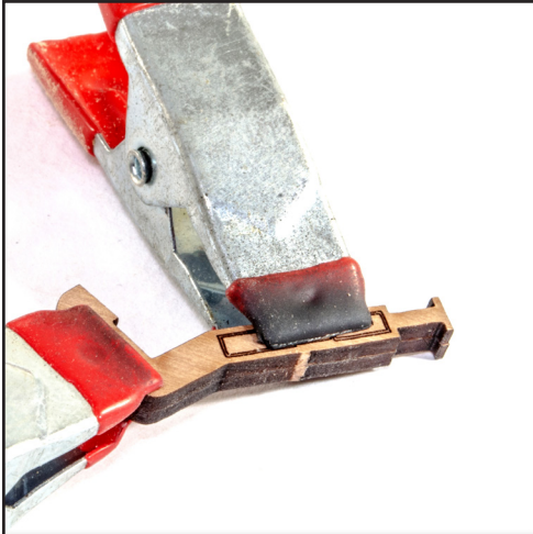
202. Glue the 2mm parts together to create two catheads. NOTE: These parts are paired. Parts 256 and 257 are a pair, and parts 258 and 259 are another pair.
