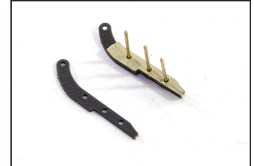
359. Sandwich one part PE-28 between two parts PE-27, using pins to align the parts and superglue to secure the parts.
