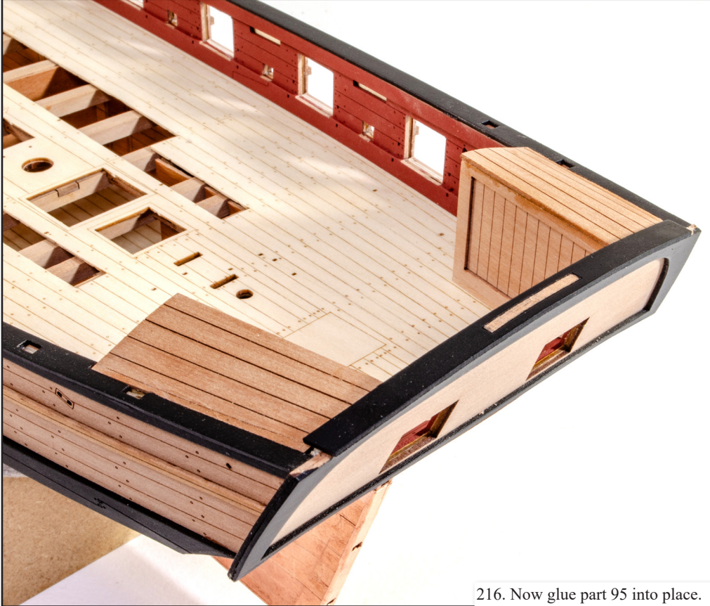
215. Sand the top of the stern so that it's level.
