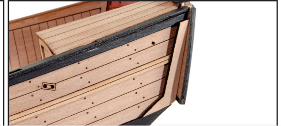
218. Temporarily sit in position on each side of the hull and score the side rails where these parts sit over them.
