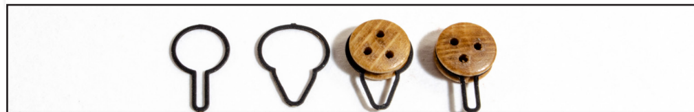
407. We now need to add the deadeyes to the channels, using the PE strips. From the 0.4mm PE sheet, remove all parts PE-16 and PE-22. You will also need your 5mm and 3mm deadeyes. Take the PE parts and splay them with pliers or a suitable tool. Pop the deadeye into the part and then squeeze the PE back together again. We find it best to prime and pre-paint these parts before assembly.
