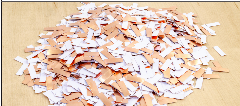
188. Take your copper tape and cut it into lengths that are 18mm long. You can leave a few meters of copper uncut on the roll.
