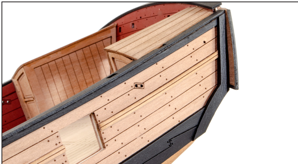
221. From the 0.6mm wood sheet, remove both parts 82, paint black and then glue into place as shown here. You should also paint the small visible area of the inside stern in black too. Now is also a good time to paint the gunport linings in the same red as the interior.
