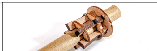
366. Assemble the parts as shown here, using a length of 6mm dowel to align. Do NOT glue the dowel.
