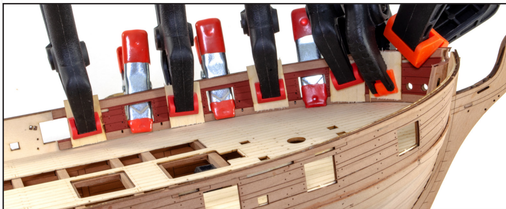
158. So as not to get red paint anywhere near the model, we suggest you mask the upper and lower sections of these parts, and then paint them red before gluing in place. We've also used scrap wood to protect the painted surface from the clamps. Here you see part 90 being clamped into place after glue. Leave to thoroughly set. NOTE: You will need to bevel the inside front end of this part so that it pushes fully into the inner prow. Make sure those gunports are fully aligned. Use the gunport jigs if you feel this will help you.
