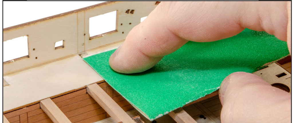
149. Use both a knife and sandpaper to remove any remnants down to deck height.
