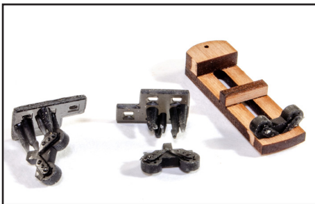
381. Take the 3D-printed carronade wheels and remove them from their blocks. Use superglue to glue them into the underside of the carronade carts.
