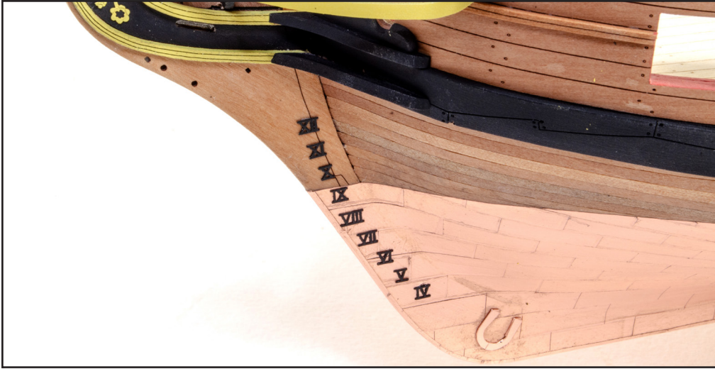
247. From the 0.2mm PE sheet, remove two sets of depth markings, paint black, and apply to the hull as shown. Marks are on the prow to assist with positioning.
