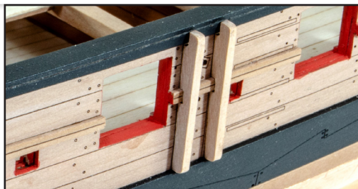
223. Glue these to the side of the hull, in the vertical engraved areas.
