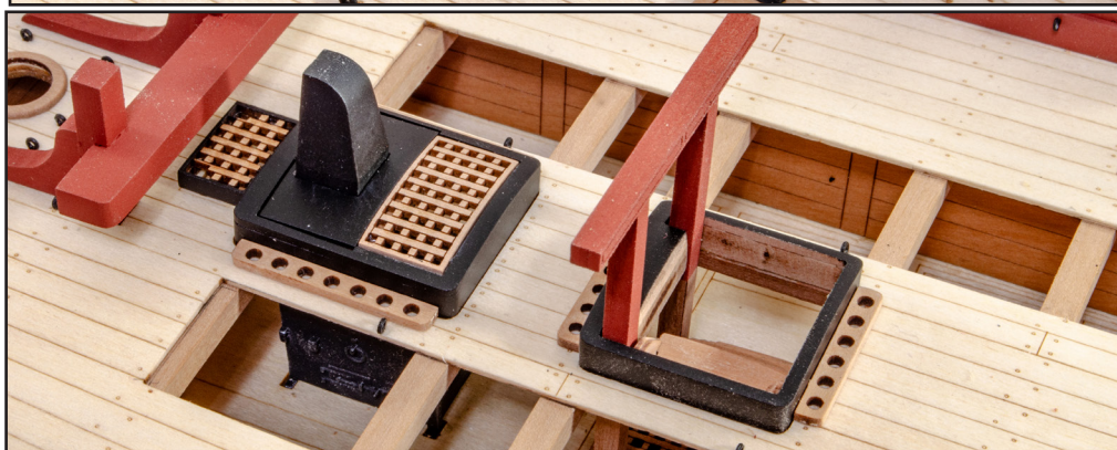
376. On the 1.5mm wood sheet, you will find a series of shot garlands which are specific to their deck locations, adjacent to the various black coamings. Remove these from the sheet and place into positions shown on the plan.
