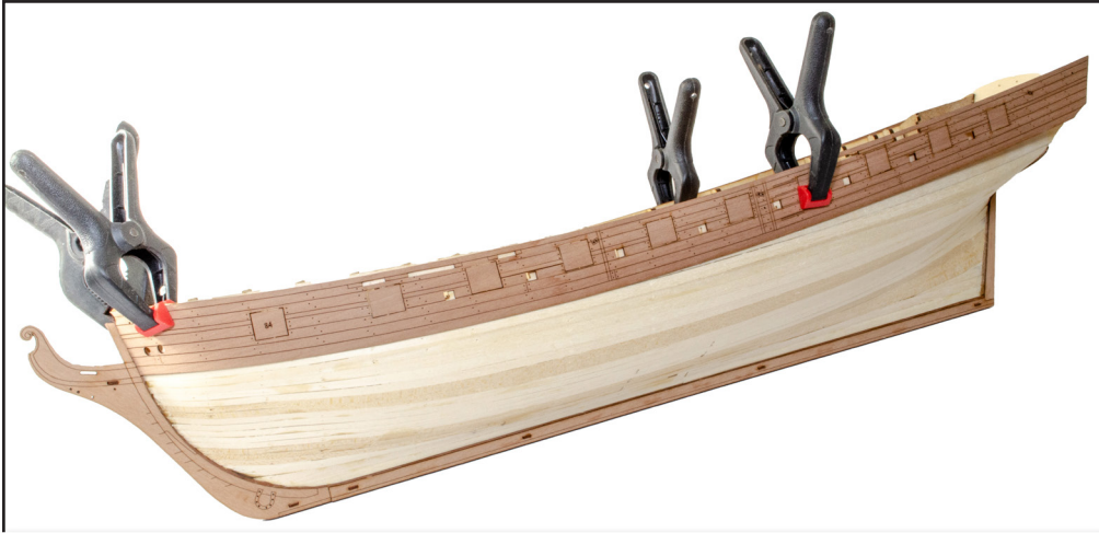
136. If you wish, you can soak the forward portion of each of these parts and leave them on the hull to dry so that retain a curve at the bow. If you do soak these, remember that you MUST leave the parts around 24hrs to thoroughly dry out as pear expands quite a lot when wet.
