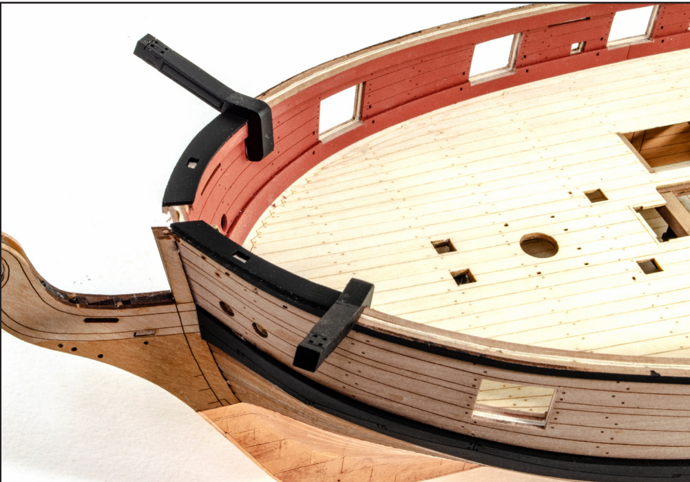
204. Glue both catheads into position. NOTE: Assembly from parts 256 and 257 is to be glued to the starboard side, and assembly from 258 and 259 is to be glued to the port side.
