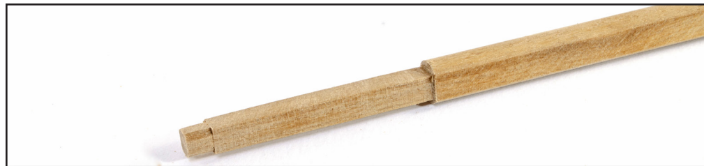
434. The upper part of this area now needs to be shaped as per plan, so it will allow the mast top to be slid comfortably over it, but not too loose.
