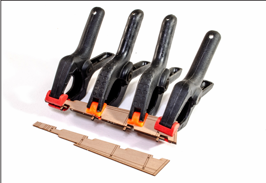
191. Glue the outer engraved parts to the inner core, clamping as you go to prevent any curling.
