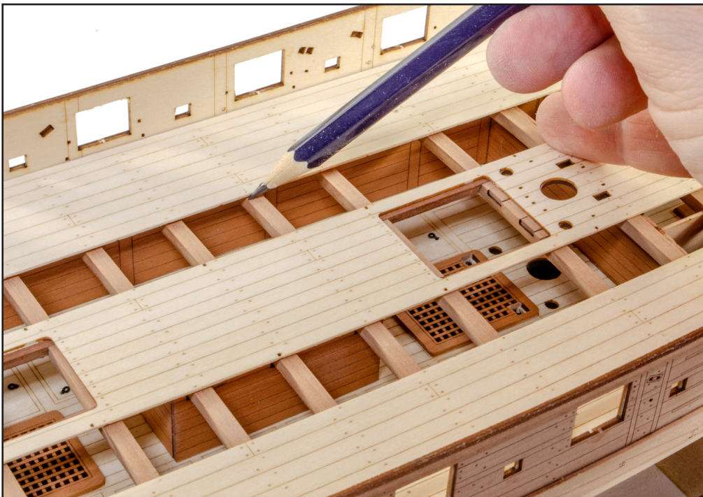
152. Trial fit the deck into the hull but carefully flexing it. If any material needs removing from the deck, do this carefully until the deck sits flat down onto the ply sub deck. When in place (no glue), use a pencil to draw around the open areas of the deck. These lines will be used as a guide NOT to add glue into those areas!
