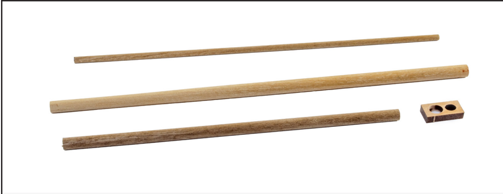
412. It's now time to build the bowsprit. Use your plan to cut the three dowel sections needed for this assembly. You will also need part M35 from the 4mm wood sheet.
