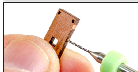
379. On the sides of parts 231, you will see an engraved slot. Using a 0.8mm drill bit, drill a hole in the middle of that slot, a couple of millimetres deep.
