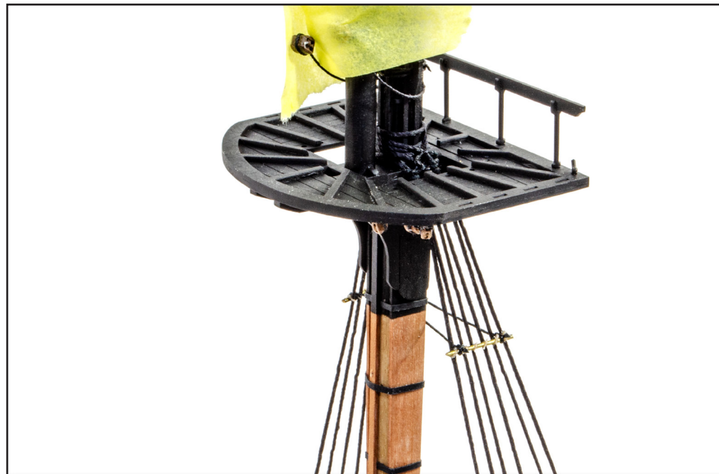
474. As per the same plan sheet, you now need to use brass rod and thread to add the catharpins to both main and fore mast shrouds. These provide stability to the shrouds and stop them from being pulled out of shape.
