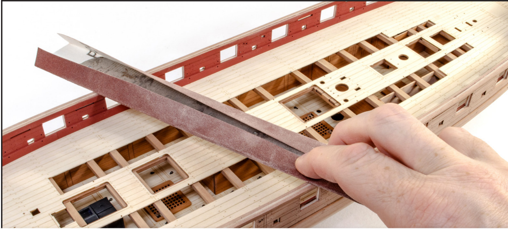
181. Take a 12-inch steel rule, or similar, and wrap it in sandpaper. Now even draw this across the tops of the bulwarks, equally levelling them.
