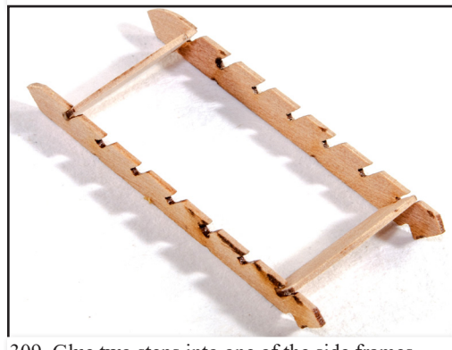
309. Glue two steps into one of the side frames, leave to dry and then glue the other side frame into place, making sure everything is 'square'.
