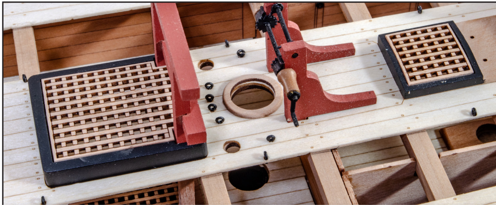
355. From the 1mm wood sheet, remove part 131 and fit to the main mast base as shown. You can use wood dowel here to ensure perfect alignment. (Again, please ignore the orientation of that winch!)
