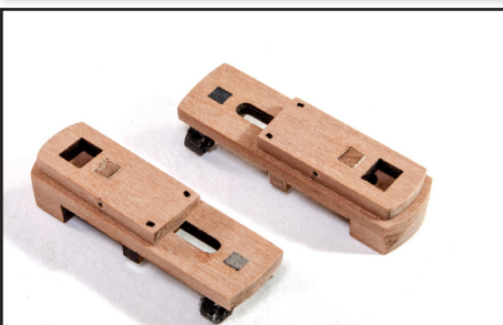
383. Fit the carronade bed to the upper side of the carronade carts, as shown here.
