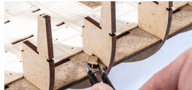
26. Push the parts through the bulkheads as shown here. This will lock the deck section in position. DO NOT GLUE!
