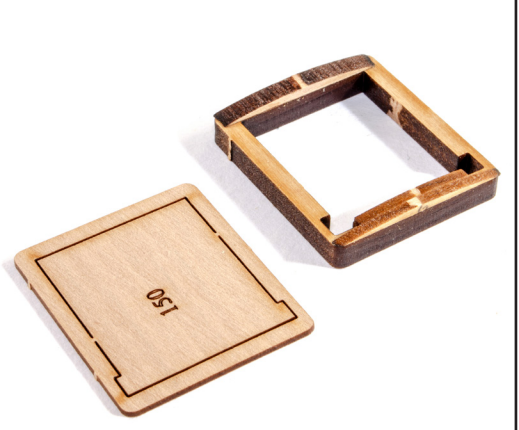
287. From the 1mm wood sheet, remove part 150, but don't fit quite yet. Also leave the infill in place for the moment.
