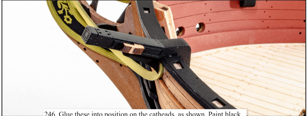
246. Glue these into position on the catheads, as shown. Paint black.
