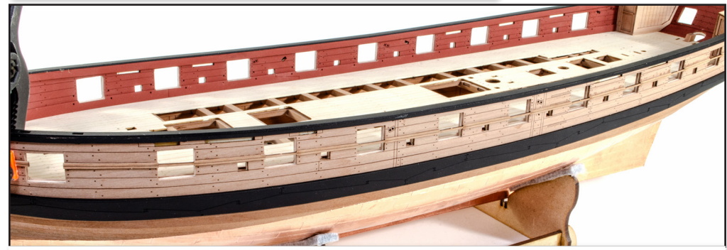
208. Now glue part 99 into place as shown. The narrow sections are designed to span the gun port openings.
