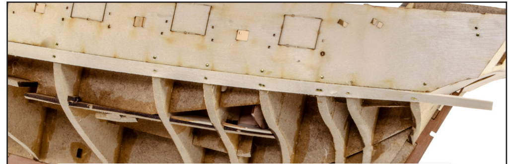
119. Here you can see the plank at the stern. The excess can be trimmed off later.
