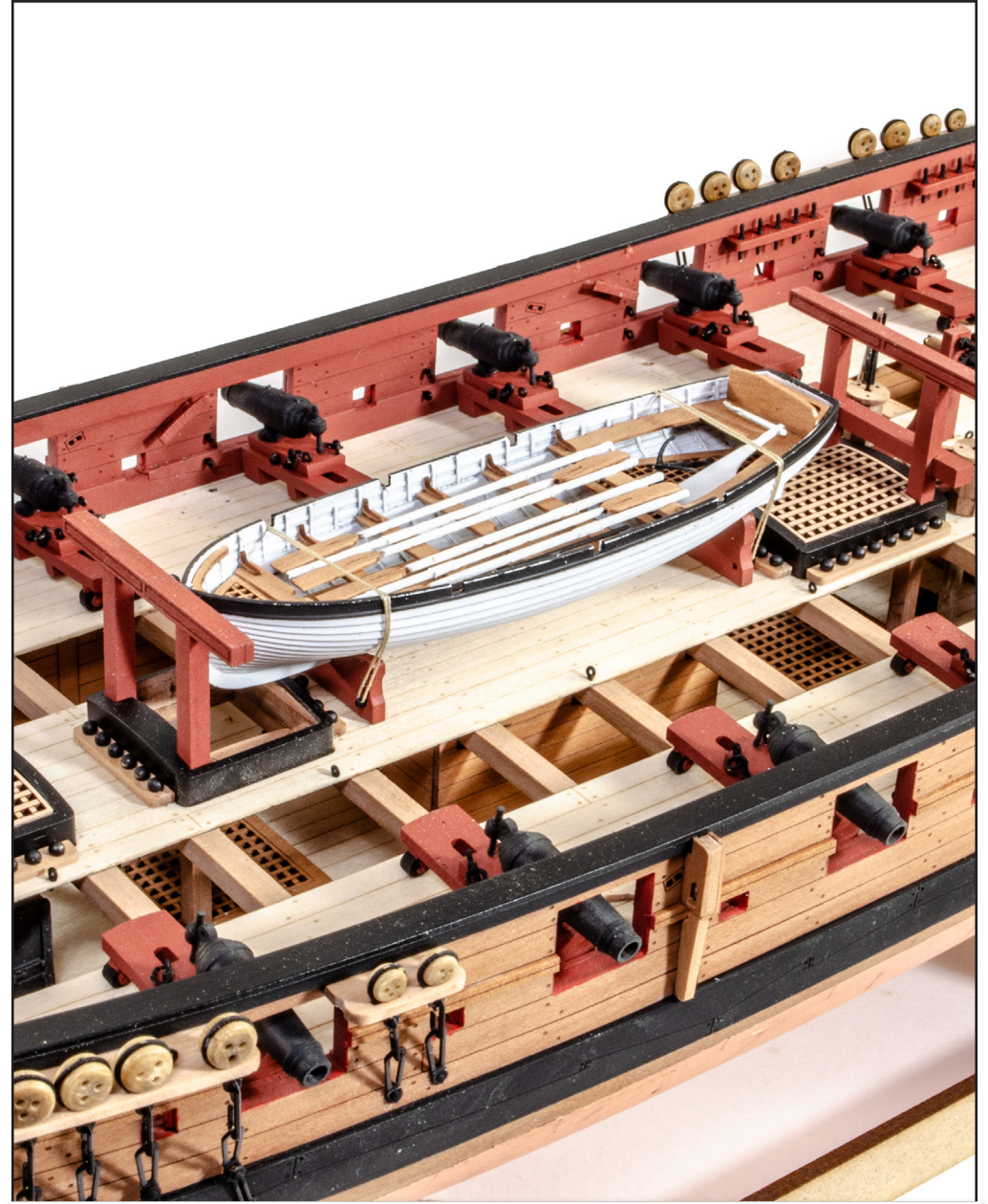
410. After building your 22ft Cutter as shown on the plan, you can then add this to the deck using the cradle parts 262 and 262, found on the 2mm wood sheet. You will also need some eyelets PE-14, found on the 0.4mm PE sheet. Use 0.25mm natural thread to lash the boat to the cradles.
