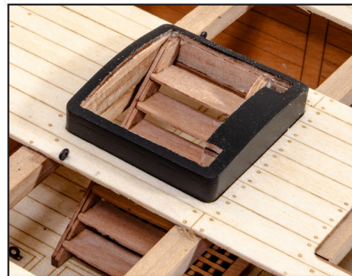
311. The ladder can now be fitted to the ladderway, noting orientation.
