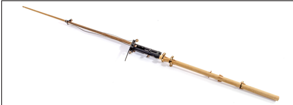
421. Paint the section in black as shown and then finally add the various rigging blocks and deadeyes to complete this assembly.
