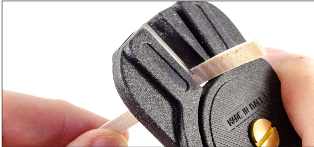
117. Again, if you feel the need to slightly curve the planks, whether at the bow or stern, nipping them on the inside is a nice and easy way to do this.
