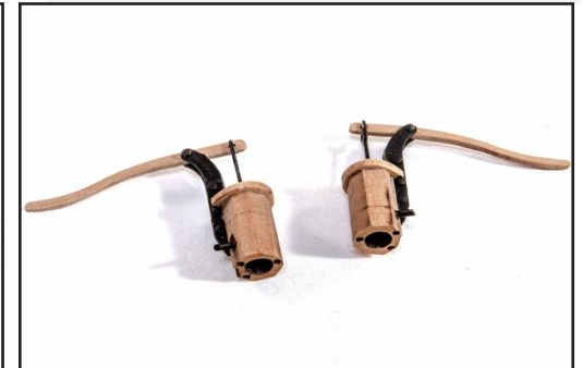
363. Drill a small hole near the base of each pump and attach a small length of 0.8mm brass rod. This is the drain spout.
