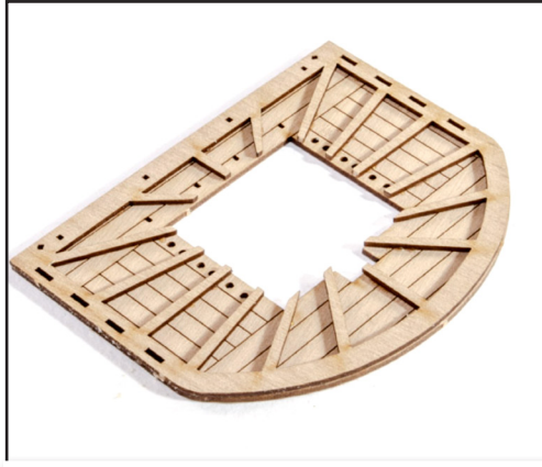
425. Glue together as shown, clamping until set. This is the fore mast's 'mast top'.
