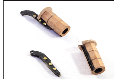
360. Cut the brass pins short and glue the metal assemblies to the pump bodies as shown. The metal assemblies have a shoulder on the back. This is what will lean on the top of the pump cap.
