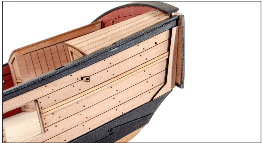
220. Parts 100 can now be glued into place, sitting flush with the rail. NOTE: It's a good idea to paint the forward edge of these parts so you don't mark the hull.
