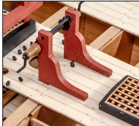
332. NOW...I always talk about orientation, and here I took the photo with it the wrong way around. Work smart, not like me! When you fit this assembly, make sure it points in the opposite direction. I've included an amended photo so you can see how it looks.
