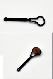
89. From the 0.4mm PE sheet, remove parts PE-5. Slightly prise open the loop, sit a 3.5mm deadeye within the loop, and then close the loop again. 8 are required.
