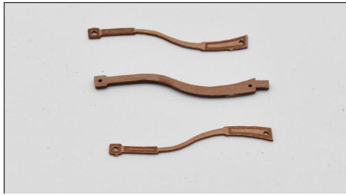
91. Make up the tiller arm with the core (66) the left outer (34L) and right outer (34R). You can use brass pins to help with alignment, and the edges of the tiller arm can be rounded off slightly. Using PVA wood glue, slot the tiller arm into the slot in the rudder head.
