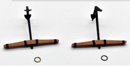
Paint the anchor black and then glue it into the stock. Finally, remove the anchor rings PE-7 from the 0.4mm PE sheet. Twist these slightly to open them, then slide into the hole in the anchor before twisting the part closed again.
