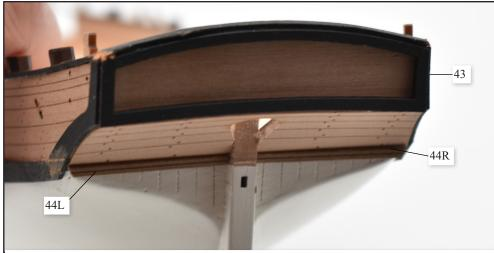
Parts 43, 44 L and R in place. Note the small amount of filler used to completely seal any joins. Do not be afraid to use filler for this purpose, as dealing with minor gaps as you go will enhance the overal look of the completed model. Once the filler is hard, sand smooth and paint over.
