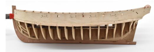
The first plank successfully pinned and glued in place.
