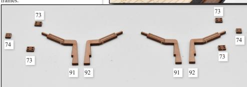
77. Catheads - Remove the cathead patterns (91 and 92) from the 1.5mm wood sheet, and the sheaves (73) and end caps (74) from the 1mm wood sheet.
