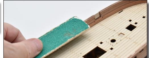
63. Above - Sand the top edge of the three bulwark layers flat, so that the gunwale seats perfectly flush with the top edge when fitted.
