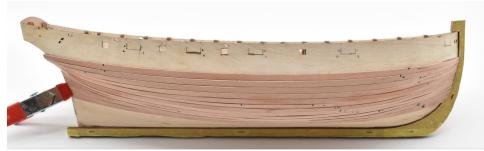
Planking progress with 12 planks per side done. Some stern planking is clamped to ensure they are fully adhered to the hull.
