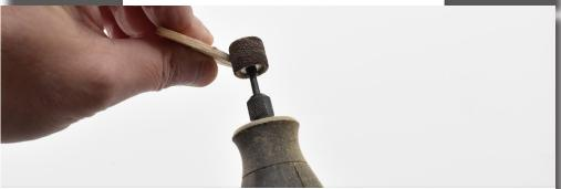
2. Bulkheads 1-4 and 13-17 can be pre-bevelled at this stage. Only put a slight bevel on these bulkheads, as they will be sanded to the correct angle one all are in place at a later stage.
