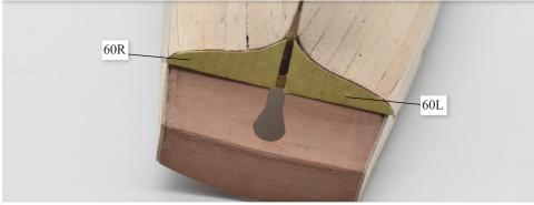
34. The stern planking patterns can be covered with masking tape, to help avoid any scratches when second planking is laid. Using PVA wood glue, fix 60R to the right side, and 60L to the left. Once fully cured, carefully file/sand the edges so they are completely flush with the edges of the hull sides.
