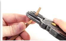
This plank bending tool is the ideal boat modeller's tool for the bending strips to the desired curvature. Used for perfect and precise bending of all wooden strips, such as planking on model boats up to 2mm thickness. For bending at an angle, change the cutting angle and the plank will 'spiral'. The more cuts produced the tighter the bend. Includes a plastic blade stopper.
