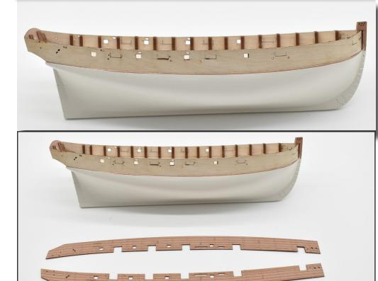
47. Now that all of the 'messy' work has been done, the outer bulwark patterns can now be glued into place. No pins were used, just claps. As with almost all wood to wood fixing, PVA wood glue was used. This was brushed onto the ply side, and the wood engraved bulwark placed and clamped in place, as shown.
