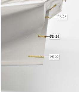
45. Hull painting almost finished. Before adding the last two or three coats, glue the rudder and rudder post hinges (PE-22 and PE-26) in place as shown using cyano glue.
