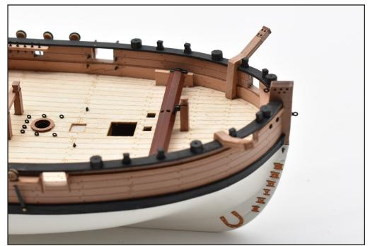
92. Add the Pawl Post so that the pawl touches the winch drum, as shown above and below. The bowsprit bitts assembly can now be glued in place, as shown below.
