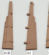
43. The main rudder assembly consists of three parts, the core (61), the right side (61R) and left (61L). 61R and 62L are glued to 61.
