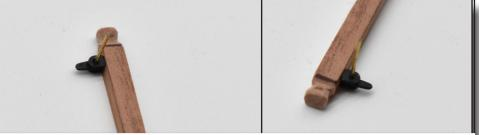
Glue the pawl brackets (PE-12) into each slot in 114. Insert the pawl (PE-13) and then lock it in place with a brass pin, which is then glued at the end and the excess snipped off.
