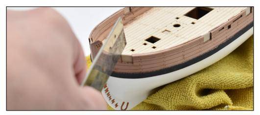
64. Above - using a Razor Saw, carefully cut away the ply gun port openings. Below - File the gun port openings so that all three layers are completely flush in the four inner edges, using a flat needle file. Take care not to damage the deck, perhaps add masking tape to the deck for protection in case you slip with the tool.
