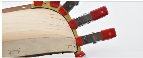
36. Glue the prow patterns in place, using parts 65 for perfect alignment, along with the outer keel sides (58). Use PVA wood glue, but take care to not allow too much glue to seep into the slot for the second planking
