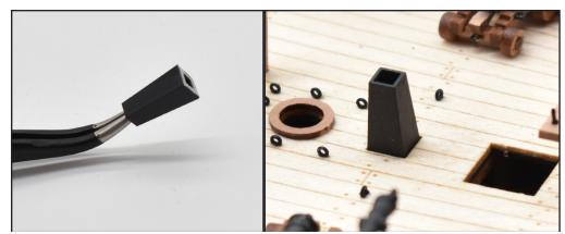
96. Paint the chimney (F3) black and glue in place as shown above using Cyano gel. The chimney coaming (96) can then be pushed over the chimney and down to the deck, as shown below.
