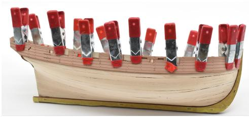
38. Parts 51L and 51R can be either glued into position at this time, or, as we have done here, just clamped into position. I decided to just clamp and not glue these so that I could just get the correct planking line for the 0.8x4mm planking strips, and then remove the engraved outer bulwark before painting the lower hull white, making sure no paint touches the engraved patterns.
