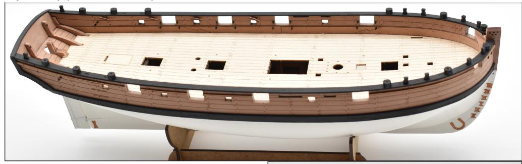
74. Remove the channels (89) from the 1.5mm wood sheet and glue in place. There are slots in the bulwarks so they can only be fitted one way. Use PVA wood glue. Each has a hole for an eyebolt (PE-1), which can also be painted black and glued into the channel at this point,
