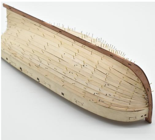
32. Once the planking is complete, remove every single pin from each of the planks. The hull can be sanded smooth using either abrasive paper or a small powered Mouse type sander.
