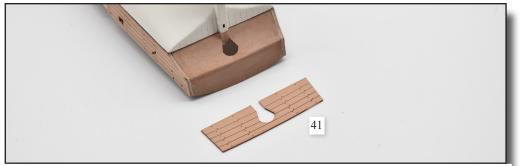
49. The outer lower stern counter can now be added (41) Brush glue watered down PVA wood glue to the cotact surface and clamp in pace as shown
