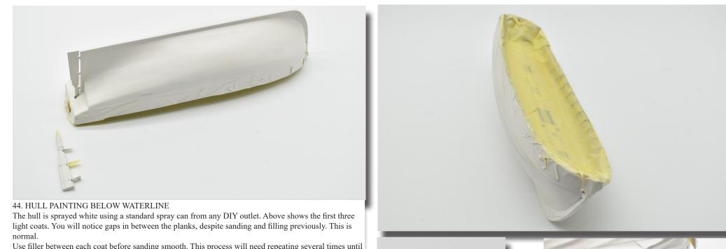
Use filler between each coat before sanding smooth. This process will need repeating several times until all gaps are eliminated.
