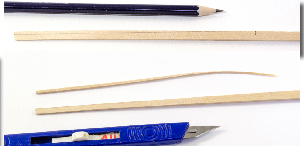
Below - Marking out the taper starting position at the stern.
