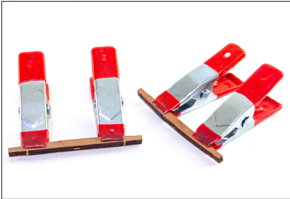
B. Before gluing the halves of the anchor stocks together, test fit the anchor shaft between them and if necessary, deepen the engraved area a little when the anchor sits comfortably within, remove the anchor and glue the stock halves together.
