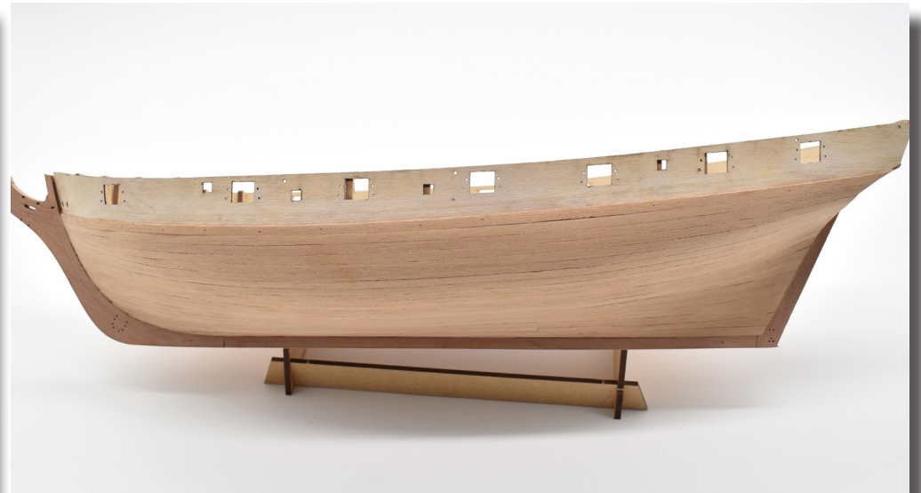
Progress of second planking at the stern. Note the planks are more or less flush with the edges of the rudder post.
