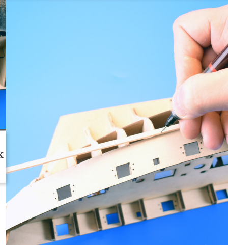
Below - Marking out the taper starting position at the stern.
