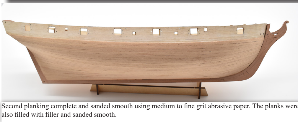
File/sand the edges of the planking so that it is flush with the stern counters.
