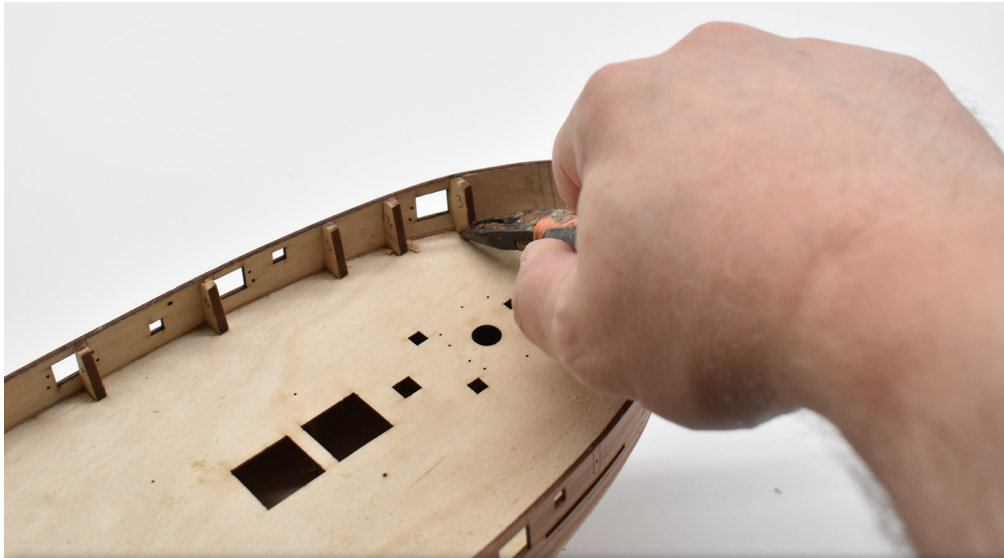
18 - Remove all bulkhead tabs above deck level by carefully bending and twisting with a pair of pliers or similar. Once removed, sand any remaining stubs flush with the deck.
