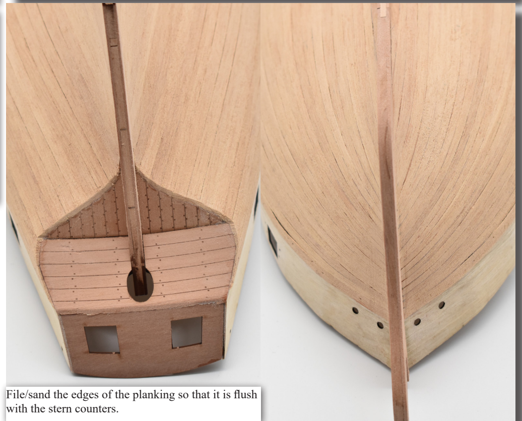
Second planking complete and sanded smooth using medium to fine grit abrasive paper. The planks were also filled with filler and sanded smooth.
