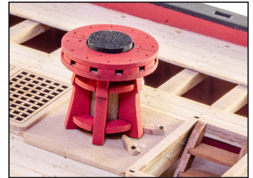
632. Paint the drum head black and sit on top of the dowel in the centre of capstan. Now glue the pawls to the coaming and insert two brass pins for the bolts. Paint the pins black.
