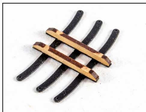
865. Assemble the cross trees like this, gluing the wooden parts to the underside of the PE.
