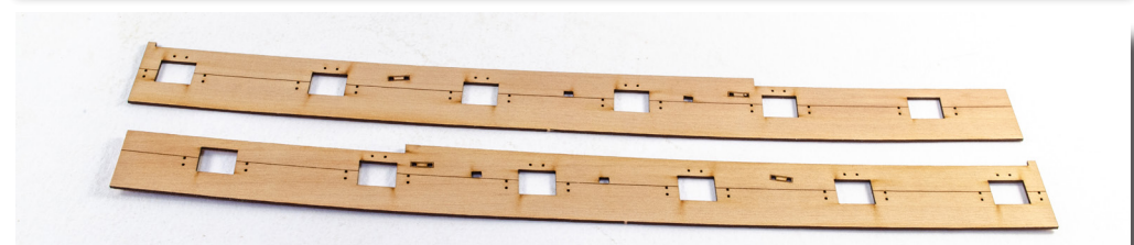
88. From the 1mm wood sheet, remove the Inner Gundeck Bulwark Pattern – Front Left (213), and the Inner Gundeck Bulwark Pattern – Front Right (215).
