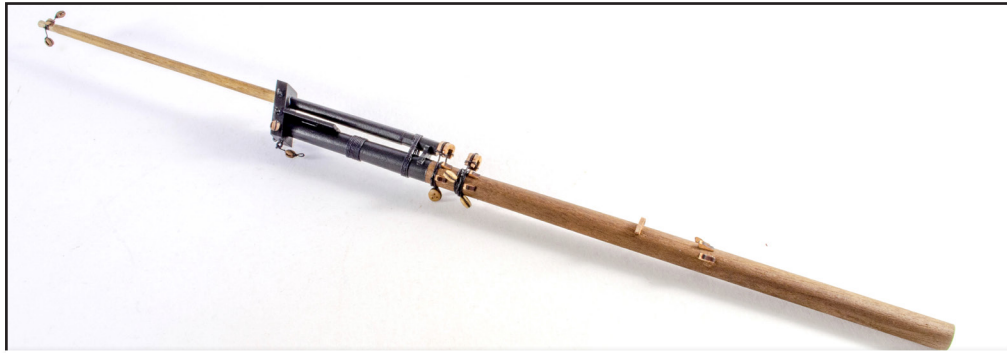
877. Paint and varnish the bowsprit as shown and then fit the correct rigging blocks to it, as per plan.
