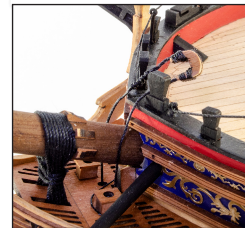
891. Slot the rigging cord through the round holes in the bow grate and then through the hole in the bow knee. You can seize both ends of this together (either above or below the grate, so the block is in the position shown on the plan. This can also be seen on Plan Sheet 21.
