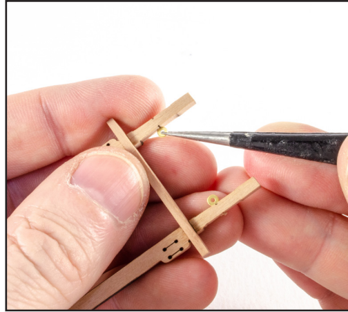
378. Insert the eyebolts on the inner sides of the assembly, and then paint black.
