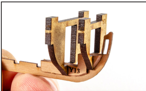
762. Sit parts Y13 into position as shown. Note that these parts sit in slots Y1 and Y2. Glue Y13 to the keel but NOT to the bulkheads. The upper edges will align with the keel.
