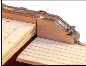
558. Glue the 1.5mm piece into place followed by the 0.6mm as seen here. You may need to bevel the underside on these to conform the gangway camber.
