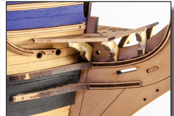
292. Glue the Bow Cheeks into position as shown. These will sit on top of the rails you recently fitted to the prow.
