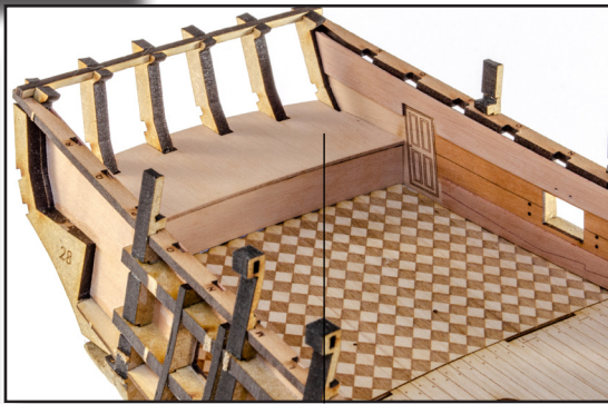
114. Now glue the Stern Cabin Seat Pattern (198) into position. You may need to trim this slightly to fit your model exactly, and we have allowed for these variations.
