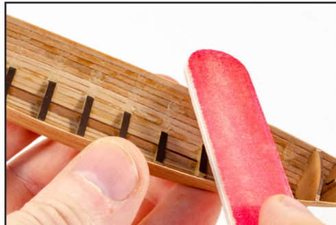
743. You can now use a sanding stick to draw over the upper edges of the bulwarks, to evenly level them.
