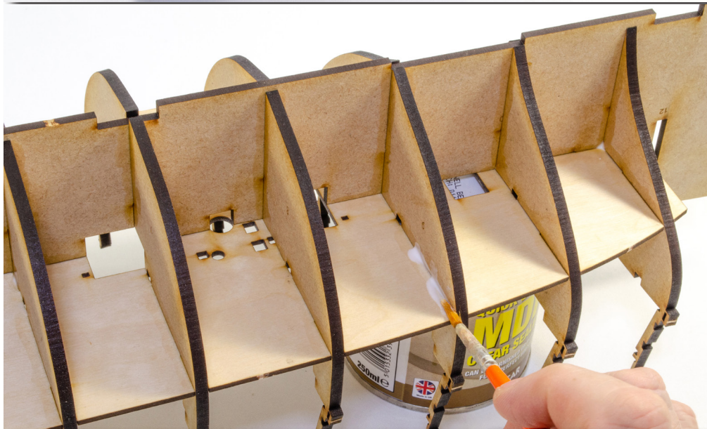
37. Turn the hull upside down and rest the lower deck on two items of similar size (paint tins etc). This will trip the bulkheads in position so you can paint wood glue into the joints between the deck, bulkheads, and keel. We find it's useful to slightly dilute the glue with water to make easier to apply with a brush. Leave the hull overnight to dry.
