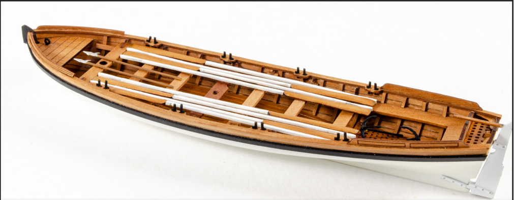
725. We suggest you fit the oars as we have here. You can stow the anchors at the back of the boat and for the boat hooks, we've sat them as shown, towards the front. Paint the handles in brown and the hook in silver.
