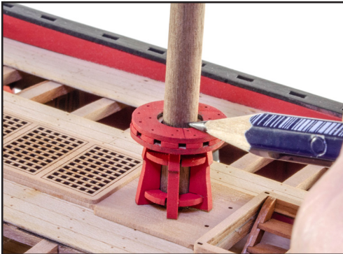
630. Push a length of 6mm dowel down into through the quarterdeck and into the gun deck capstan below. Slide the new capstan into place over this as shown. Use a pencil to mark where the dowel at the height of the capstan. Remove the dowel and cut to the length you marked. Now re-insert it with glue and glue the capstan into place.
