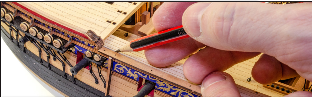
551. Trim the gunwale to the correct length (note that the two holes closest together go towards the front) and sit the gunwale over the gangway. Where they overlap, draw a line on the gangway.
