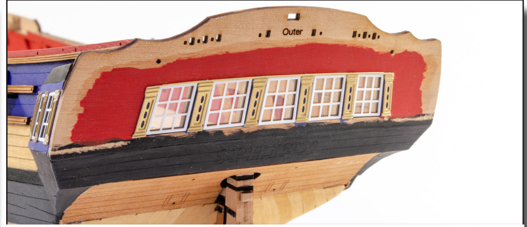
306. Glue the Stern Column Panel as shown here. This will sit directly above the window frames and the bottom of the columns will align with the bottom of window frames. We used CA gel to fit this as it allows some time to move the part. Now fit the Quarter Gallery Vertical Columns. Note these protrude evenly beyond the top and bottom of the window frames.
