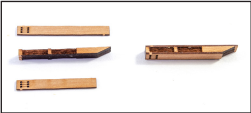
607. Glue the top and bottom patterns into place so the pattern holes are at the square end of the cathead.
