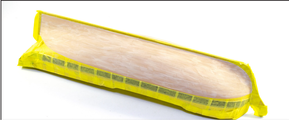
230. Carefully mask the waterline and ensure you have a good, sealed joint. Use a suitable filler (we suggest acrylic) and dilute the mixture before applying with a brush. When dry, sand the filler back to the wood and re-do this until you have a good surface with no cracks or holes.
