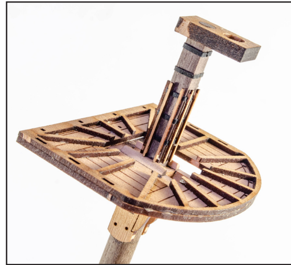
817. Now take the mast middle section (Mizzen Topmast) and shape as per plan. Drill the hole for the 'fid'.
