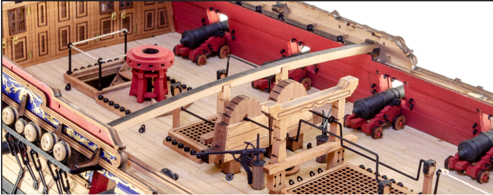
495. Glue Deck Beam 'A' into position. There are engraved marks on both the deck beam and location point which shows where each fit. Beam 'A' will also sit atop the two chain pump handle stanchions as shown.
