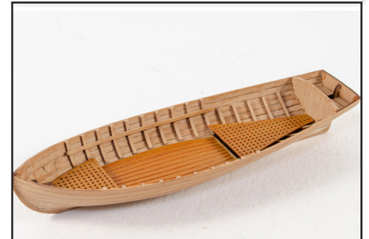
783. Use CA to fit the floor sections into position inside the hull. Also fit Y22 into position in the rear of the boat, as shown.
