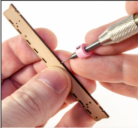
267. You'll notice a laser cut line on the edges. In the middle of this, drill a hole into the channels using a 0.6mm drill bit.
