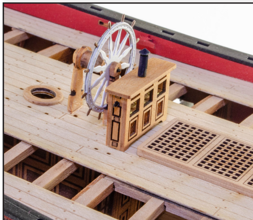
651. Glue the binnacle into place with the 'Towards Wheel' side.
