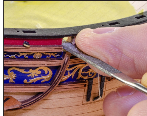
611. Test fit the cathead as you go. When complete, paint the catheads black and glue into position.
