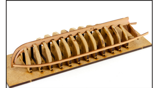
735. Lie the first of the hull planks (L29) from the 0.6mm wood sheet, in place as shown. This sits against the shoulders of the MDF bulkheads. We advise using wood glue for this instead of CA.
