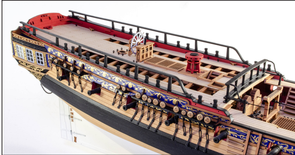
671. Glue the rails to the quarterdeck rail stanchions and make sure the forward moulding is glued to the gunwale.
