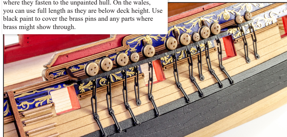
329. Before working on the deadeye assemblies, we suggest that you prime and paint black all the associated metalwork for constructing these. These are parts PE-48, PE-49, PE-50, PE-51, PE-52, PE-53, PE-54 and PE-55. Now take the 5mm Deadeye Stroops you just painted (PE-48) and the 3mm Deadeye Stroops (PE-53) and open each in turn with tweezers. Insert the correct deadeye and then close them up again to lock the deadeye into position. Do this for the correct number of 3mm and 5mm deadeye assemblies needed to fit to lower rig positions.
