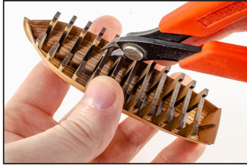
741. To remove the MDF bulkheads, first snip away the bridge on each one.
