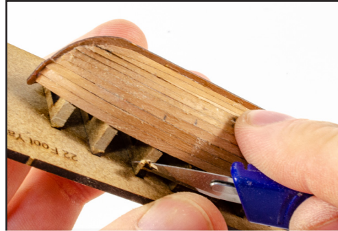
775. To help in sanding the hull, the protruding parts of the MDF bulkheads are cut away with a sharp knife.
