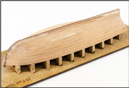
776. Sand the hull with around a 110 grade paper to begin with, using gradually finer grades to smooth the wood surface. Use an acrylic filler, slightly diluted, to fill any hollows or imperfections.
