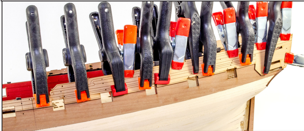
167. These can now be glued in position as shown, again applying glue to the hull instead of the patterns, to prevent curling. We also suggest a varied range of clamps so all the edges can be reached.
