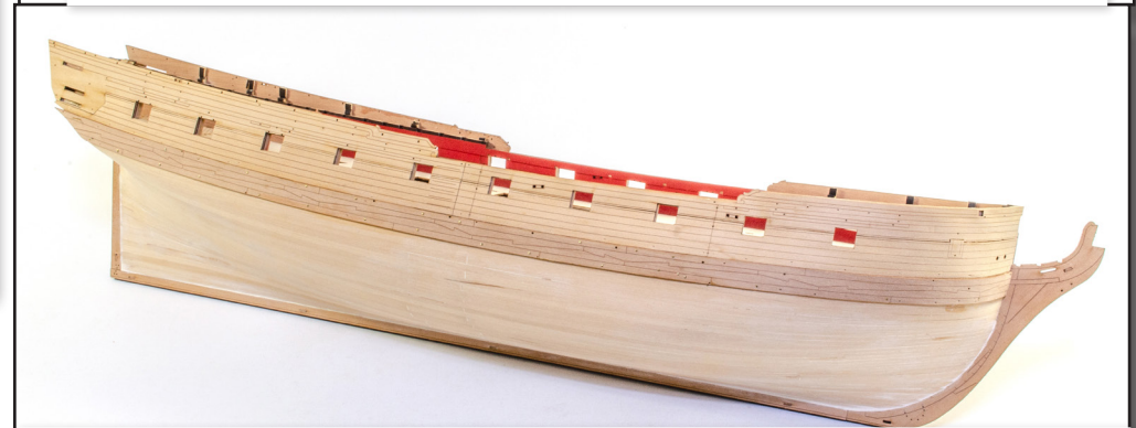
190. Both wales are now glued to the model. We used PVA for this and pinned where appropriate. There are small nail holes in the wales (NOT the larger scupper holes!), that you can use to pin. Also feel free to pin wherever you feel it necessary.
