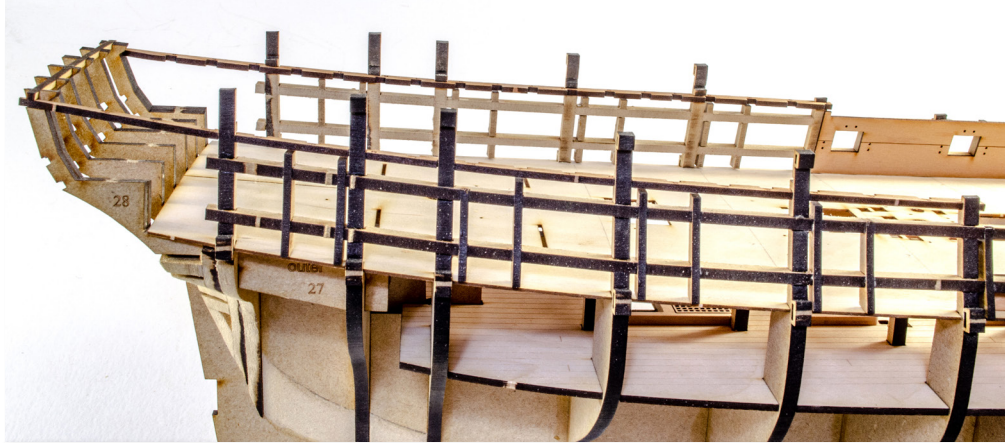
94. This photo shows how the rear of 409 and 410 slot into the timbers at the top of the stern.
