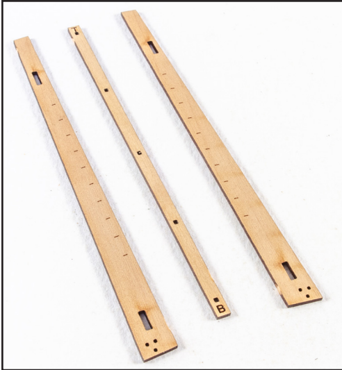
159. From the 1mm wood sheet, remove the two Rudder Post Outer Patterns (188, 189), and also the Rudder Post End Pattern (196)
