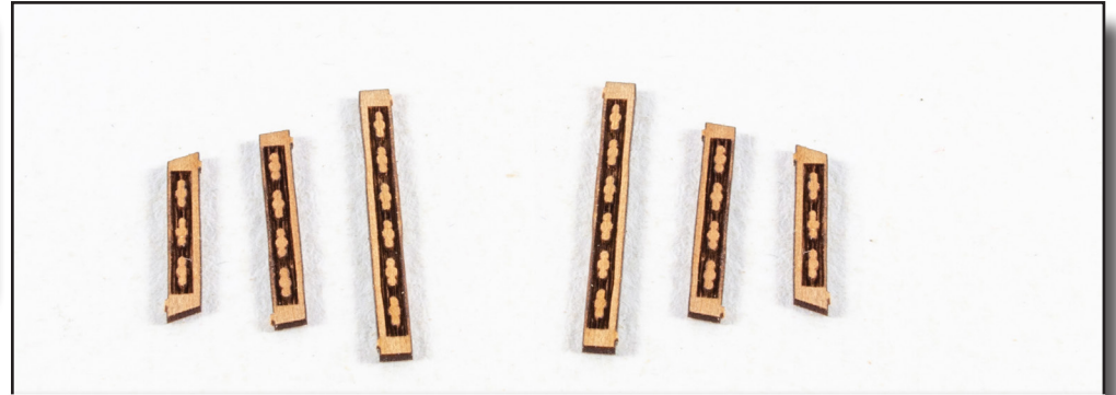
299. From the 0.6mm wood sheet, remove the V-Shaped Head Rail Pattern parts (81, 82, 83). You will need two of each for this task. There are also a spare set of parts in case you need a spare.
