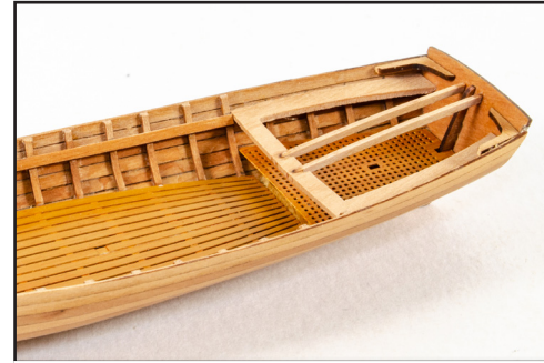
748. Glue seat L27, Knees L24 and the bow bracket L28 into position as shown.
