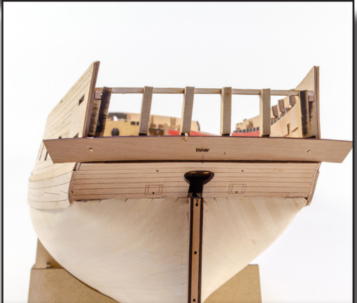
195. Glue the upper counter in position directly above the stern counter. Take some measurements of the hull and part to make sure it's placed centrally. The overhang at either side should be identical. Use pins to hold until dry.
