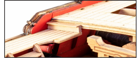
578. Fit these as seen here. You will need to bevel the inner edge to match bulwark. You may also need to trim them to the correct width, so they end at the gangway edge.
