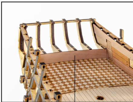
113. Glue the Stern Cabin Bulkhead Pattern into place as shown. You may need to slightly adjust the curve to the deck with sandpaper.
