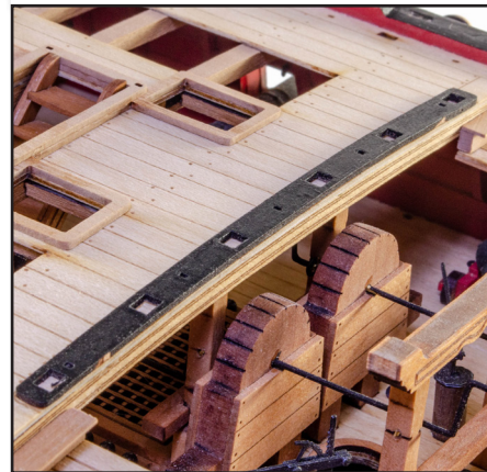
653. Glue the lower rail into position at the edge of the quarterdeck. This fits within the engraved area.
