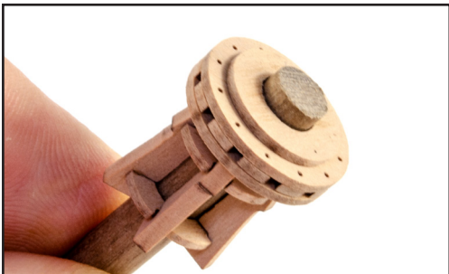
468. Lastly, glue the Capstan Top Drum Head – Gun Deck (254) in place. You can now withdraw the dowel.
