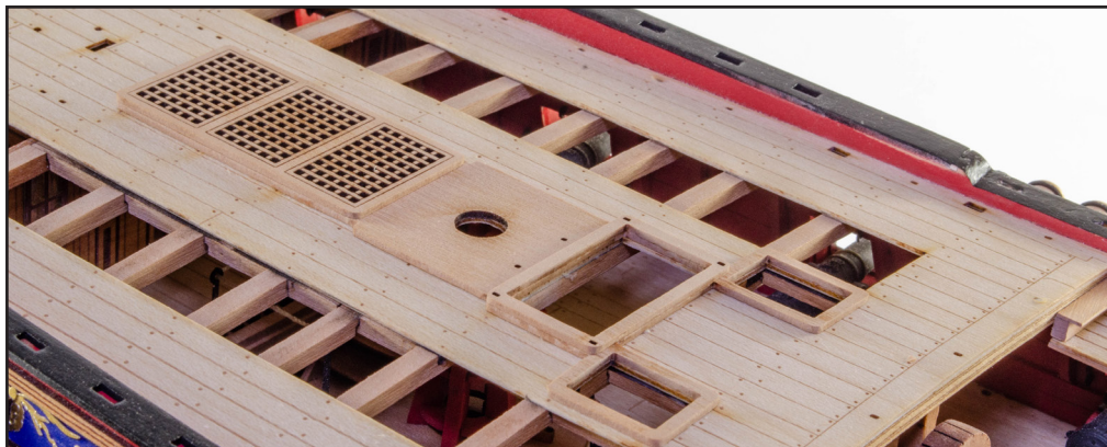
615. We now turn attention to the quarterdeck. Glue the remaining grating assembly into position as shown.
