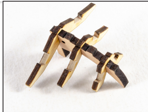
278. Glue the V-brackets to the Gammoning Knee, with the V-bracket bevels pointing forward.
