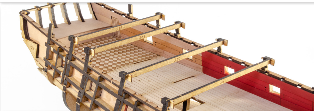
127. Lastly, from the 2mm MDF sheet, remove parts J-9, J-10, J-11, and J-12. To fit these to the appropriate bulkheads, you'll need the small keys J-0 on the 0.8mm ply sheet. As with the other jig parts, you'll find J-9 will fit to bulkhead #9 etc. Please don't glue these to the model either.
