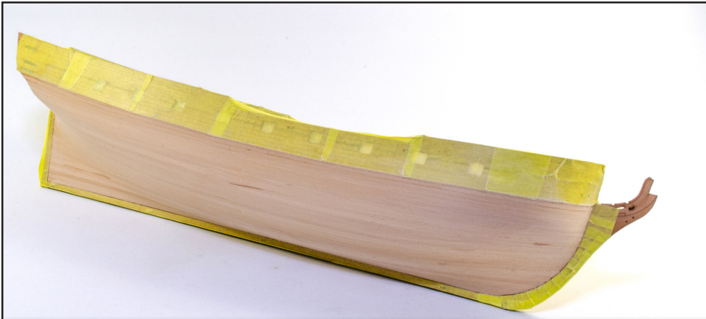
185. Before sanding, use masking tape to cover all areas that are laser engraved. The prototype was sanded with 110 grit paper.
