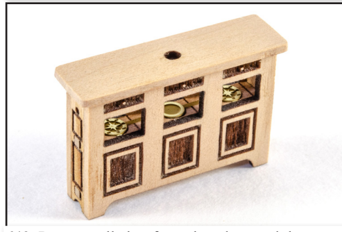
649. Remove all char from the edges and then glue the binnacle canopy into place.
