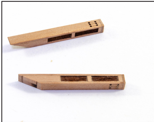
609. Remove all char and sand the top and bottom patterns so they blend into the rear cathead angle. Make two catheads.
