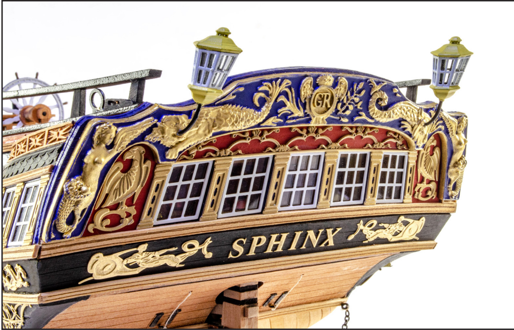
804. Shape the brass rod so it matches the profile on the plans. Drill the base of the lantern with a 0.8mm drill to insert the brass mounting rod. Fit both lanterns as shown, with their slight tilt inboard. These mount into the holes you previously drilled from the inner stern bulwark.
