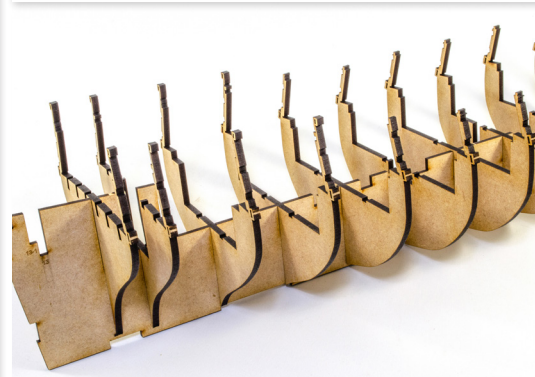
31. Lastly, slot (not glue) bulkheads 9, 10, 11 and 12 into their correct slots on the keel. If you wish, you can leave off bulkhead #12 at this stage and fit along with the bow and stern assemblies.
