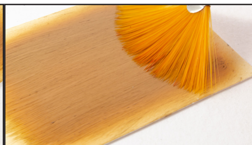
710. OPTIONAL: f. A fan brush can also be used to create knot effects and a more natural flow to the grain.
