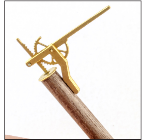
392. Now insert the side pip into the hole on the side of the dowel. Glue all assemblies.
