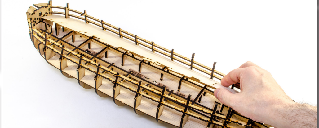
74. Slot Gun Deck Pattern (48) into position as shown. The outside edges of the deck locate into the slots at the bottom of the bulkhead ears, locking the edge in place. You will only need to pin this down towards the centre, with optional pins along the deck beams. You may apply glue first or paint it onto the underside once fitted.
