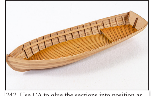
747. Use CA to glue the sections into position as shown.
