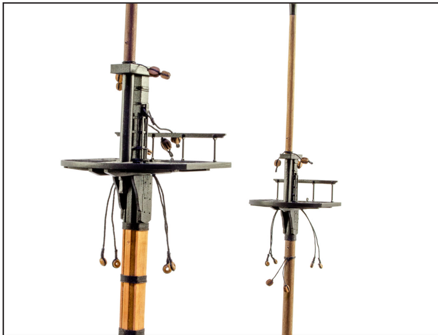
894. Before fitting the lower shroud lines, add the pendants to all three masts, using the thimbles. Check the plan for rope and thimble sizes as they vary between the fore/main to the mizzen.
