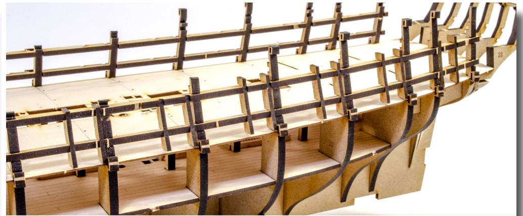
79. In this picture, ports 6, 7, 8, 9, 10, and 11 are clearly seen. Once the glue is set, fit the gun ports to the opposite side of the hull.
