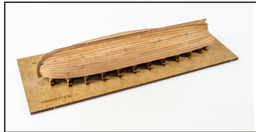
702. As you continue to plank, you will need to taper each one. The pencil marks here show where I tapered mine from. You will also need at some point, to taper downwards from the keel. Don't worry about using stealer planks to fill gaps.
