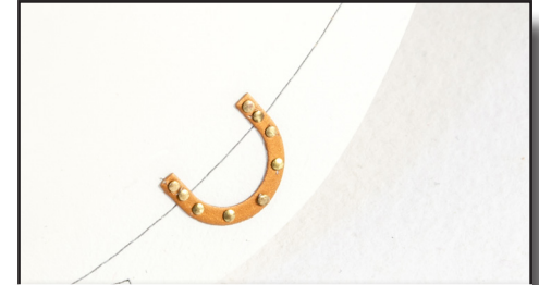
263. Prime and then paint the PE parts in copper paint. Fit the horseshoe parts as seen here. On our prototype, we use cut off brass pins on both sides as we did with the rudder. Paint the brass pins in copper also.
