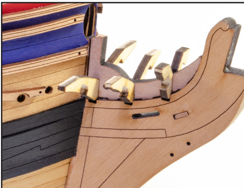
279. Sit (DO NOT GLUE) the assembly on the model. Note that the tops of the V-brackets are bevelled for contact with the gratings.
