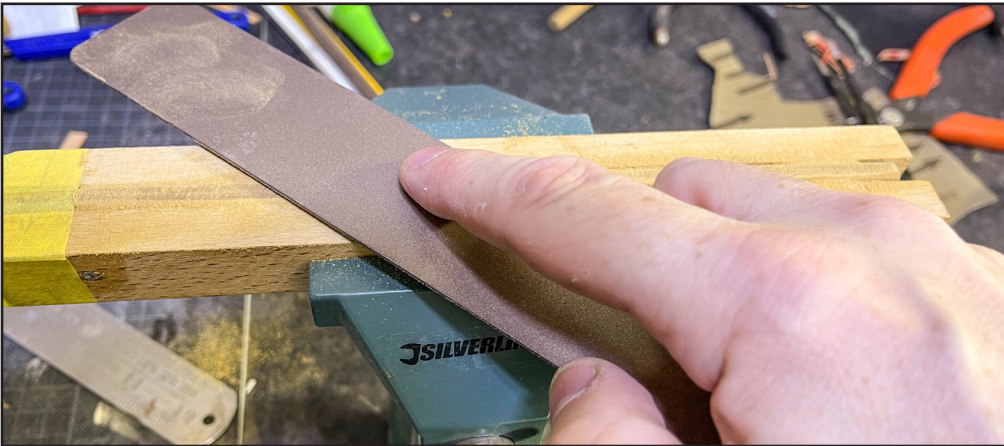
833. There are numerous ways to create the long flat sides on the lower mast section. Here is a jig that was built to do this. Two beams of birch are placed together, and two holes drilled through which are exactly 7mm from the top flat surfaces. Bolts are then inserted, being glued into one half.
