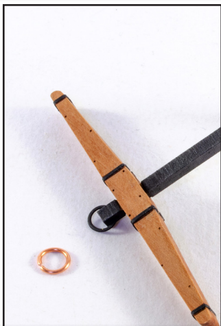
905. Use some brass wire to form the anchor hoops. Fit these to the anchors and paint black.
