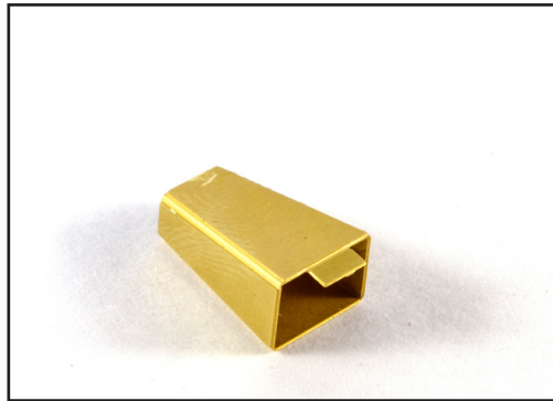
431. When complete, the flue will look like this. The small tab also bends down slightly, and you will need to test fit this to the stove to check the flue then sits flat.
