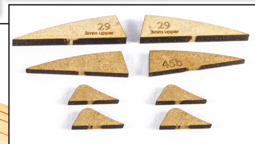
223. From the 3mm MDF sheet, remove the two Quarter Gallery Lower Finishing Patterns (29). From the 2mm MDF sheet, remove the two Quarter Gallery Patterns (45b), and the four small Lower Quarter Gallery Finishing Patterns (46).
