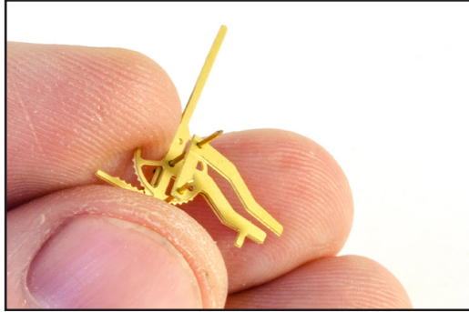
386. Use brass pins to locate a side bracket to each side of the main body. Use CA to glue.
