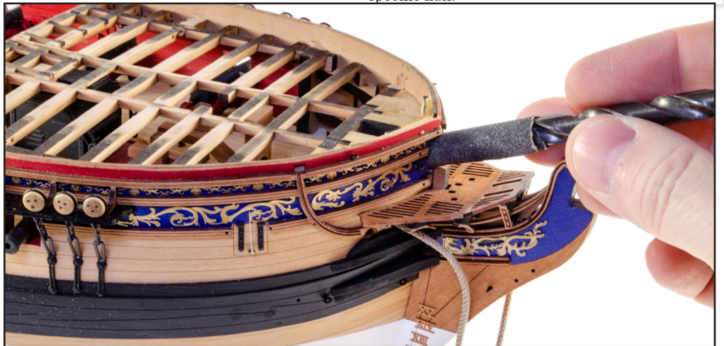
518. We can now prepare the bowsprit opening in the bow, to accept the 8mm dowel. To do this, take a drill bit around 6.5mm - 7.00mm and wrap some medium sandpaper around the shank end. Push this into the bow opening and turn the drill bit by hand as you go, opening up the hole slightly. Continue with the drill when you reach the bowsprit support, so you also elongate this too. Do this until you can slot an 8mm dowel through this and into the bowsprit support which is plugged into the gun deck.
