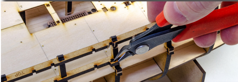
77. Before fitting the frames, snip away the 'safety gates' on the longitudinal gun port strips, as shown here.
