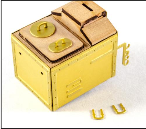
427. From the 0.4mm PE sheet, remove parts PE-76 and add these handles to the top rear of stove, as shown.
