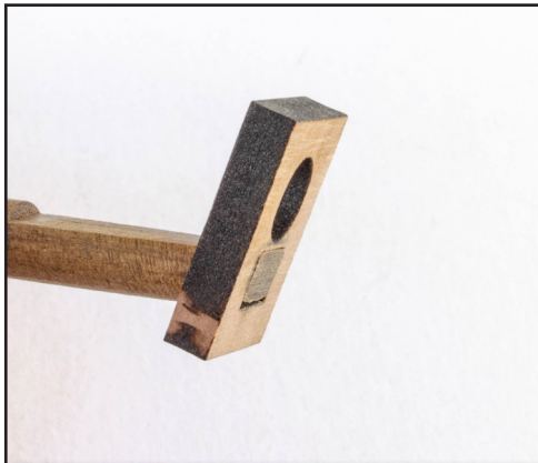
872. Test fit the cap to make sure of a good fit, and make sure the dowel is then sanded flush with the front of the cap.
