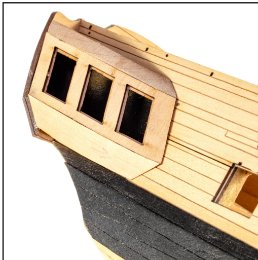
222. Glue these into position as shown here. You will need to trim these to suit your own model, and also bevel the upper inside edge so it meets the window area properly.
