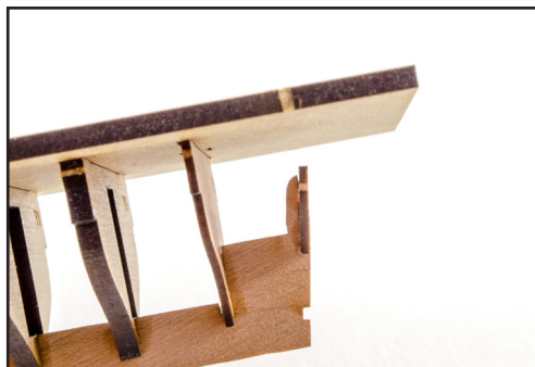
765. This photo clearly shows the stern board in position. Note that it must be fitted flush and at an angle with the rear of the keel.
