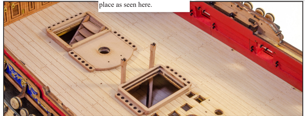
373. Bend the PE parts and sit on top of the stanchion. Now drill through the PE part into the stanchion (all the way through). Remove the PE part.
