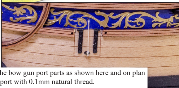
325. From the 0.4mm PE sheet, remove the Gun Port Hinge Lids (PE-111) and the Stern Port Lid Hinge (PE-111s). Also remove four of the Gun Port Lid Eyebolt (PE-109).
