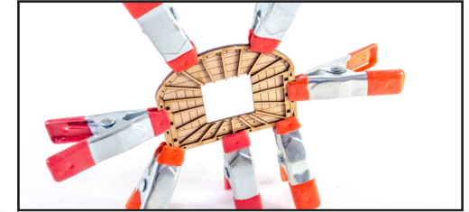
806. Glue the two parts together as shown, using clamps around the edges to ensure a perfect fit.
