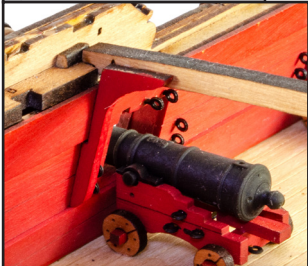
497. Here you see the knee installed for deck beam 'A'.
