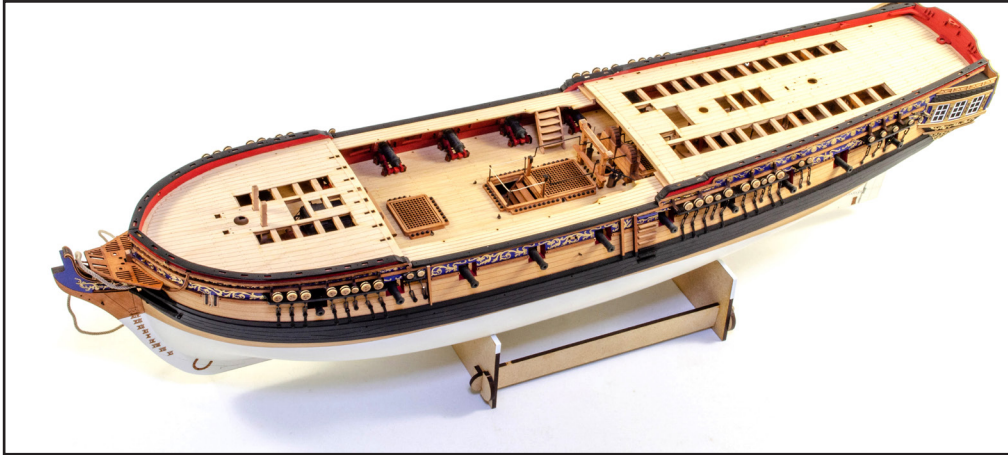
581. Glue the gunwales into position as shown. These should be more or less flush with the inner bulwarks with only the minimal of overhang.
