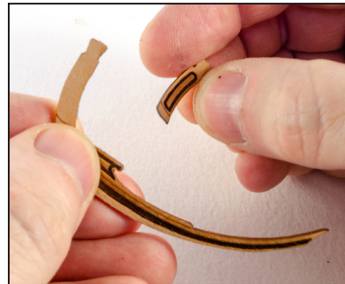
677. Glue the upper finishing patterns into place and clamp until dry.
