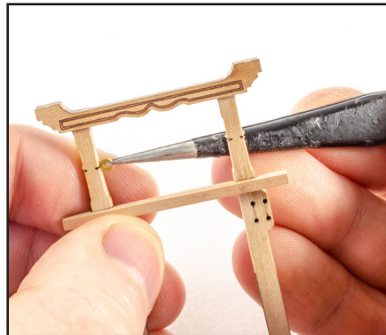
400. Glue the eyebolts into the assembly from the inside.
