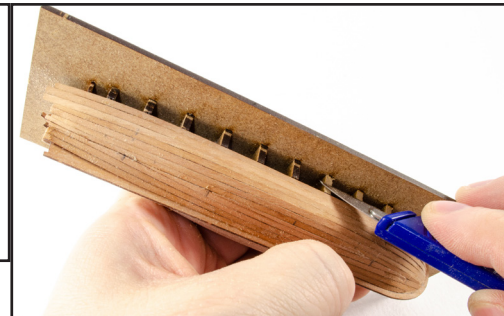
703. Trim back the shoulders of the MDF bulkheads as that will make it easier to sand the hull to shape.
