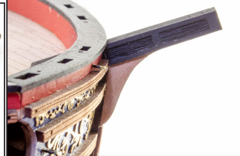
613. Glue these in position under the cathead as shown. You will need to cut back a little of the decorative trim. You will also need to slightly bevel the knees to suit the angles you have. When fitted, paint black.
