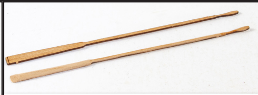
723. Sand the paddle to shape and slightly round the handle. To paint, we suggest white for the handle and just a plain varnished paddle. The paddle tip can be painted copper.
