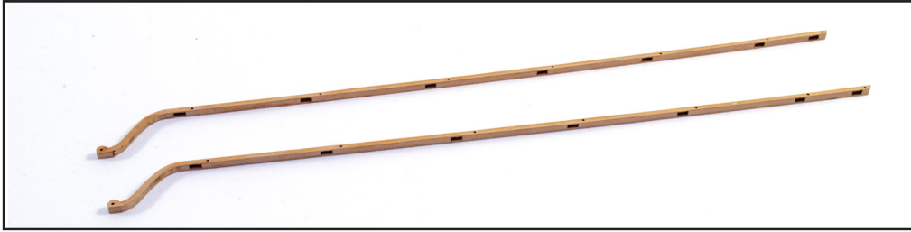
670. When dry, remove the pins and carefully sand to remove the char and make the surfaces even and level. Use filler in the pin holes and then paint the rails black.
