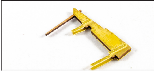
719. We recommend using CA gel to glue the PE parts to the wooden rudder as it gives time to allow for positioning.
