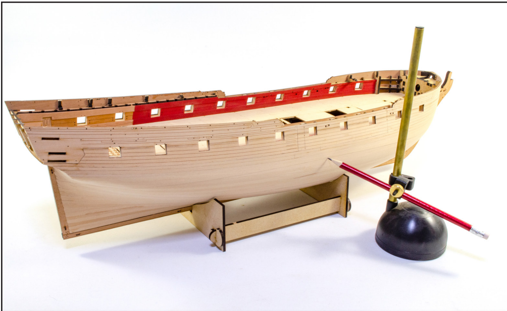
186. Check the waterline position both aft and stern (should be exactly the same!) and use a waterline tool to temporarily add a waterline mark. The reason for the waterline mark is so that the area below it can safely be filled prior to painting. We don't want any odd colour filler in the bare wood areas. For filling, we recommend an acrylic filler such as Ronseal's Multi-Purpose Wood Filler (Natural). This is first diluted with water and applied to the hull with a brush. When dry, it's sanded back and the process repeated until no gaps remain. Finish the hull with 320 grit paper, or similar. We won't paint this area just yet.
