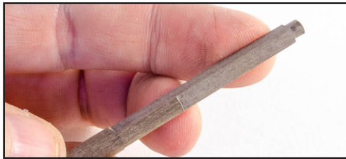
814. The upper section is then squared off on all sides and the top shaped to fit the cap block. You will need to reference the plans for the shaping of all mast sections for the sake of lengths and diameters. These photographs will just give you a general idea.
