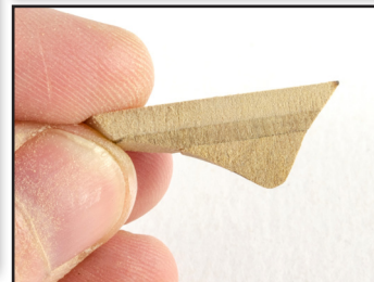
227. When shaped, the MDF will look like this. Note that whilst the front edge is tapered to a fine edge, the rear side is not.
