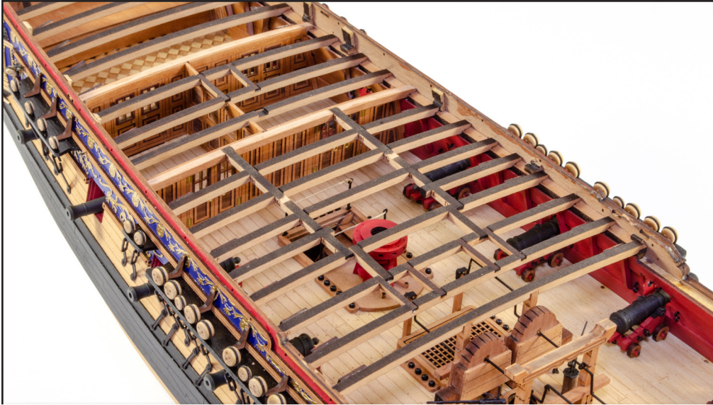
501. Glue all parts into position as seen here and on plan. Allow time to dry. Note that the parts 456 have lettering on them. Install these so the text faces away from the bulwarks.
