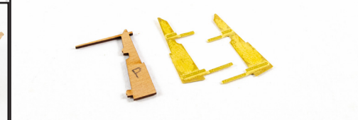
718. Cut the rudder (P17) from the 1mm pear wood sheet and also remove the rudder side patterns from the 0.4mm boats PE sheet. Note that all parts for the Pinnacle are in the same area, and that applies to the Launch and Yawl too.
