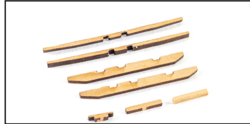
807. From the 2mm wood sheet, remove the two Mizzen Cross Trees (416) and the Mizzen Cross Tree Chock (417). From the 1.5mm wood sheet, remove the two Mizzen Cross Trees (385) and the two Mizzen Cross Trees Bolsters (385a).
