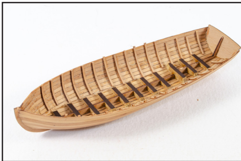
744. Carefully sand the inside of the hull to smooth things out and remove a remnant of glue. Cut the rib strips (L30) from the 0.6mm wood sheet and glue into place inside the hull, as shown. Space these 5 – 6mm apart.
