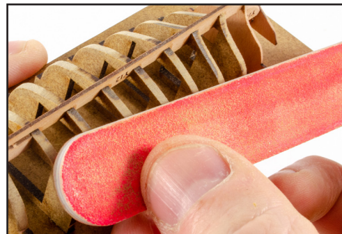
768. Sand/fair the hull using sandpaper or a sanding stick. Take a plank to make sure it lies smoothly across all bevelled bulkheads.
