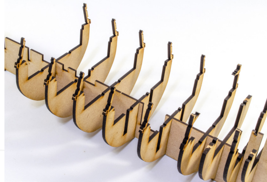
29. Slot bulkheads 1-1, 2, 2-2, 3 and 4 into position. Handle these gently as mishandling could damage the ears. Do NOT glue at this time.
