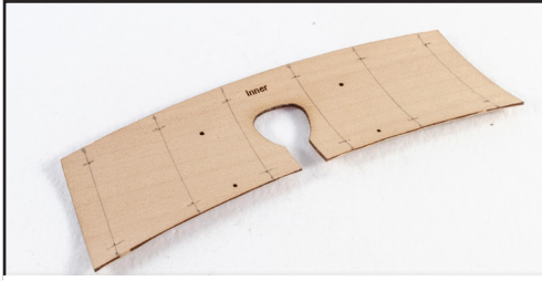
147. The counter will now look like this. The pencil lines are where I have marked the positions of the stern timbers it will sit on. I have also drilled some 0.5mm holes to make this easier to pin to the MDF underneath.
