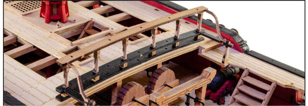
662. Using your plan as reference, mount the two stanchions on the gangways as shown and then fit the rail patterns by slotting over the stanchions and gluing to the mid breast rail. You may need to trim the latter to length. Now glue the upper rail pattern so it sits on the rail you just installed and up against the upper rail. Again, trim to fit. Paint all rails/stanchions in black.
