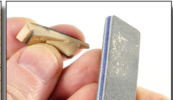
226. Remove the MDF parts from the hull and start to shape them. These will be more or less flush with the lower part of the gallery (continuing the angle of that part). Occasionally place the MDF back to the hull to test the fit.
