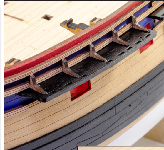
273. Fit the Channel Knees (380, 381) to the main channels. There are two sizes here for the two different rail connection points. If necessary, you can adjust the angle, so you achieve a good fit to the rail and the channel.
