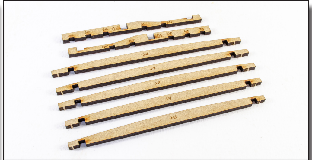
123. Before any external faces/planks are added, you'll need to get to grip with some jigs. These are designed to maintain the width between bulwarks whilst adding those external areas. From the 3mm MDF sheet, remove parts J-U, J-V, J-X, J-Y, and J-Z. Also remove parts #30. 'J' means that the parts are jigs, and these should NOT be glued to the model.
