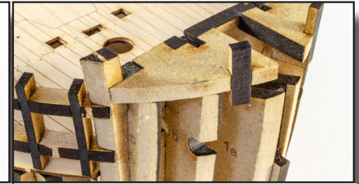
116. Glue parts #16 into position as shown into the slot on the edges of parts 18.
