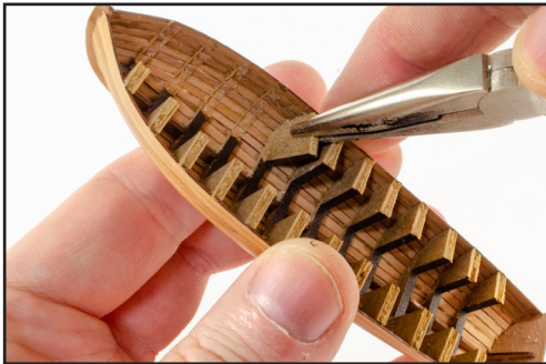
742. Use pliers to twist at each bulkhead to carefully remove them.
