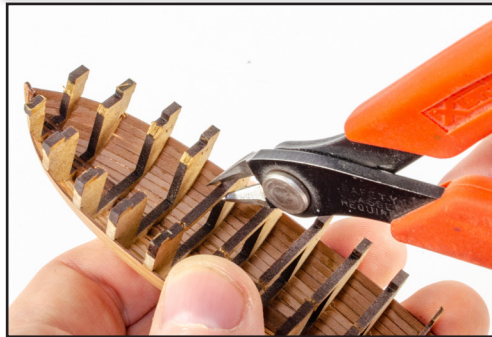
778. To remove the MDF bulkheads, first snip away the small bridge on each part.
