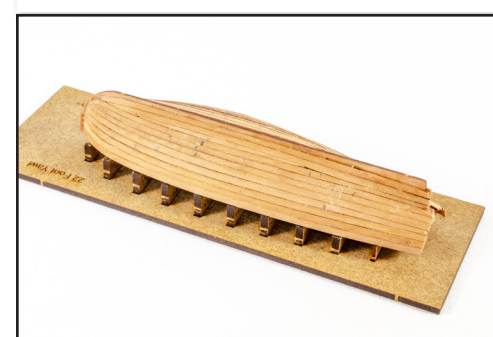
773. You may need to fit infill planks or 'stealers' as you progress. We aim to make such fillers as low as possible in the hull so the paint will cover them. You may of course wish to use a tick-strip method to plank, whichever suits you.
