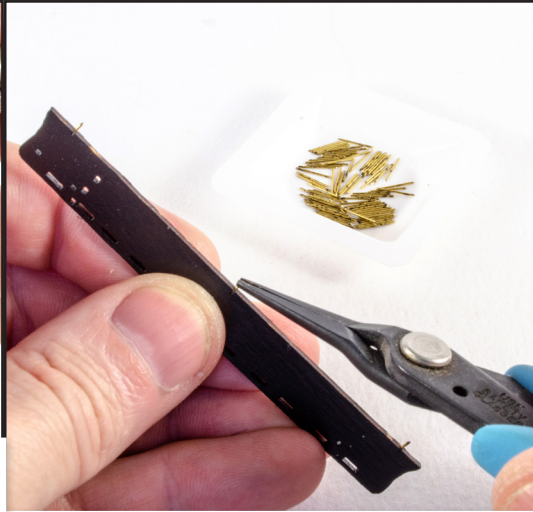
268. Paint the channels in black and now take a number of the cut-off pin lengths from your previous stages and cut to length and glue into the holes. The pointed end should stick out around 2mm, as a guide.
