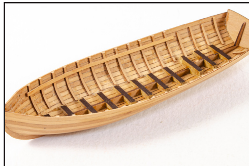
745. Use a pencil to make a mark on the ribs which is about 3mm down from the edge of the bulwark. Remove the seat support strips (L31) from the 0.6mm wood sheet, and glue underneath these pencil marks.
