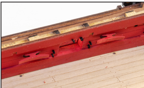
473. Glue these into position as shown on here and on the plans.
