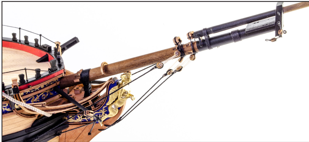
879. Rig the bowsprit shrouds and stays as per plan. You can also rig the boomkins at this stage while things are accessible.
