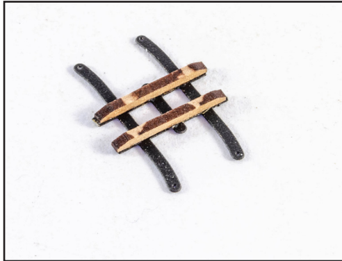
821. Glue the trestle trees into position on the underside (the surface with no details) using CA glue.
