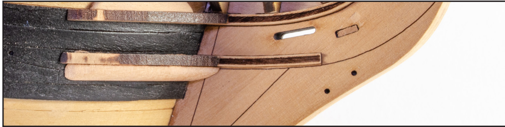
296. Glue the parts into position as shown. All of these newly added bow parts can now be painted black.
