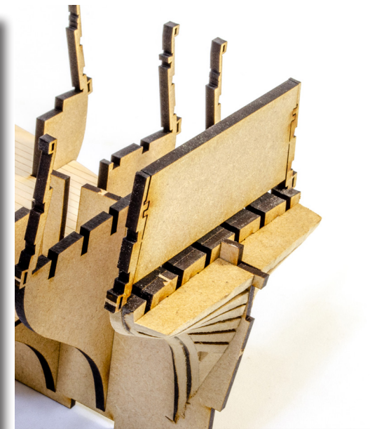
39. Now fit and glue the stern assembly into position on keel slots 13/13-1. If you previously left bulkhead #12 off the hull, you can now fit and glue this into place too.
