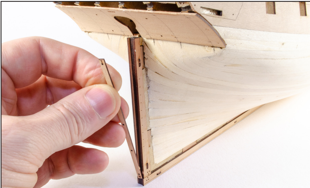
161. Now glue the rudder end post pattern into position. Note that the 'T' denotes TOP, whilst the 'B' denotes BOTTOM.
