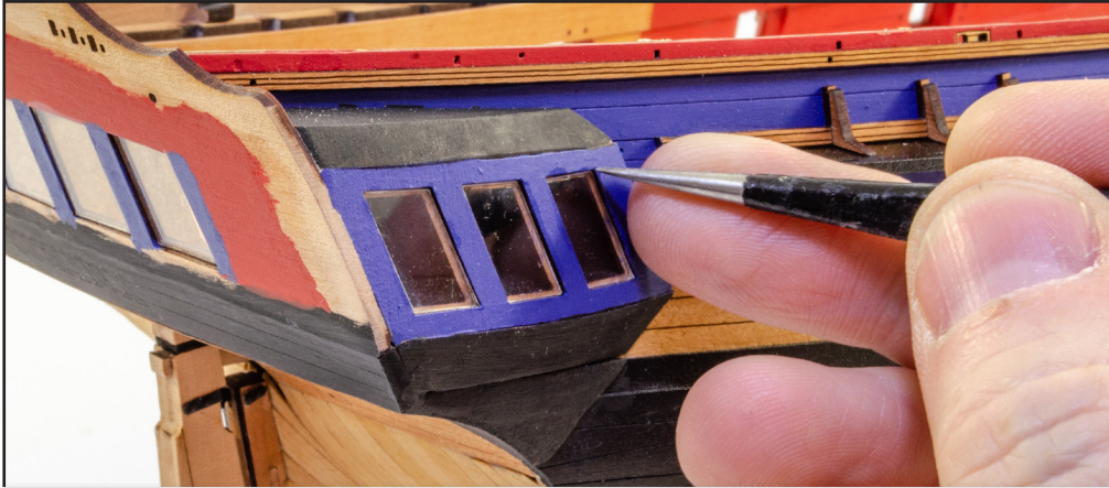
302. Test fit and glue the windows into the recesses on the quarter galleries and stern, using the numbering on your plans. You may need to file these a little to make them fit. Clear acrylic varnish was used to glue these into position as CA can fog the transparencies.
