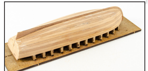
739. Sand the hull smooth using 110 grade abrasive paper to start with and then finishing with finer grades. We suggest any imperfections are filled with an acrylic filler, diluted with water.
