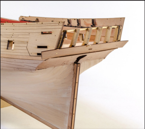
195. Glue the upper counter in position directly above the stern counter. Take some measurements of the hull and part to make sure it's placed centrally. The overhang at either side should be identical. Use pins to hold until dry.
