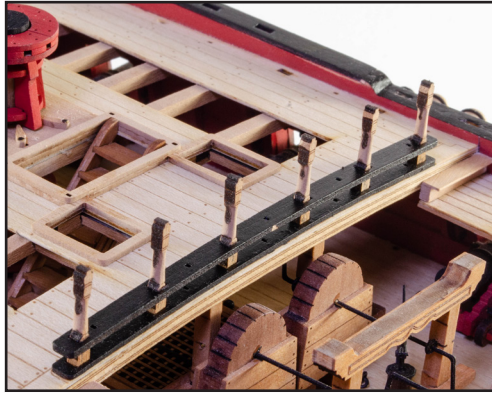
657. Slide into position and glue the middle rail. This will sit on the lower stanchion shoulders.
