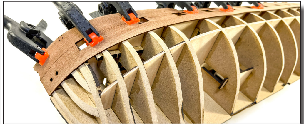
133. You will note that if you faired the hull properly, these parts will lie flat against all bulkheads, with no ripple or gaps. If you do find gaps, you'll have some time to correct this before we finally fit these parts.
