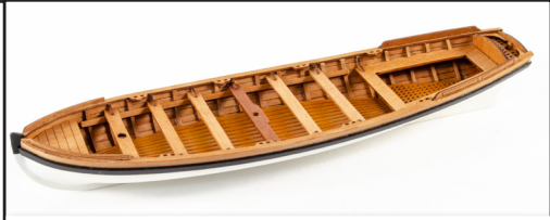
720. Paint the hull white and the wales (from the planking strips) in black. Glue the wales into position as shown. The wales will simply follow the path of the second plank down, on each side.
