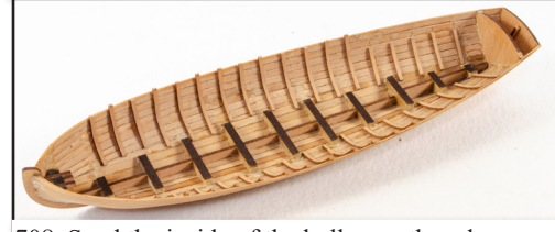
708. Sand the inside of the hull smooth and remove any glue remnants. Remove the rib strips (P31) from the 0.6mm wood sheet and fit as seen here. Space them around 5 – 6mm apart.
