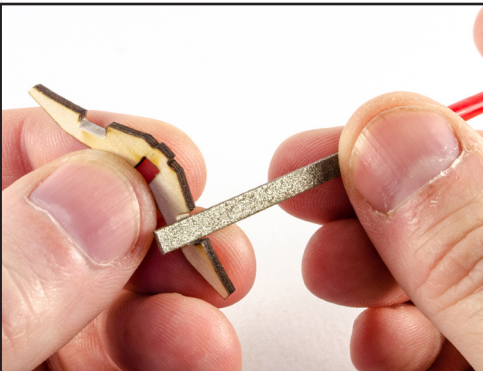
277. Using a file, bevel one side of the slots on each V-bracket, as shown. On the prototype, we angled these about 45 degrees.
