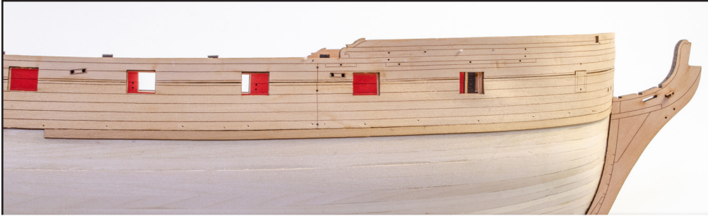
176. Glue the front upper pattern in place as seen here. You can use whichever glue you choose, but we do recommend CA gel as it no pinning is required, and the parts can be quickly fitted.
