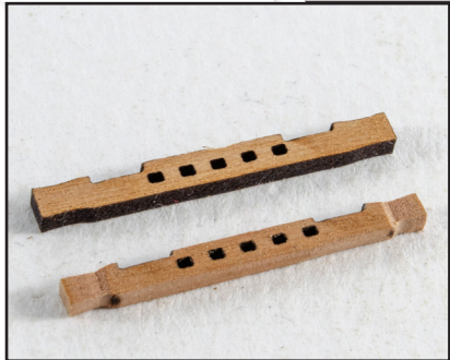
584. From the 2mm wood sheet, remove the Fore Bitts Cross Beams (426). Remove the char and slightly shape the ends as seen here.
