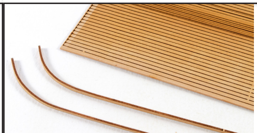
699. If you want to bend the first 0.6mm hull planks (P30), you can soak them but make sure they are thoroughly dry before fitting them.
