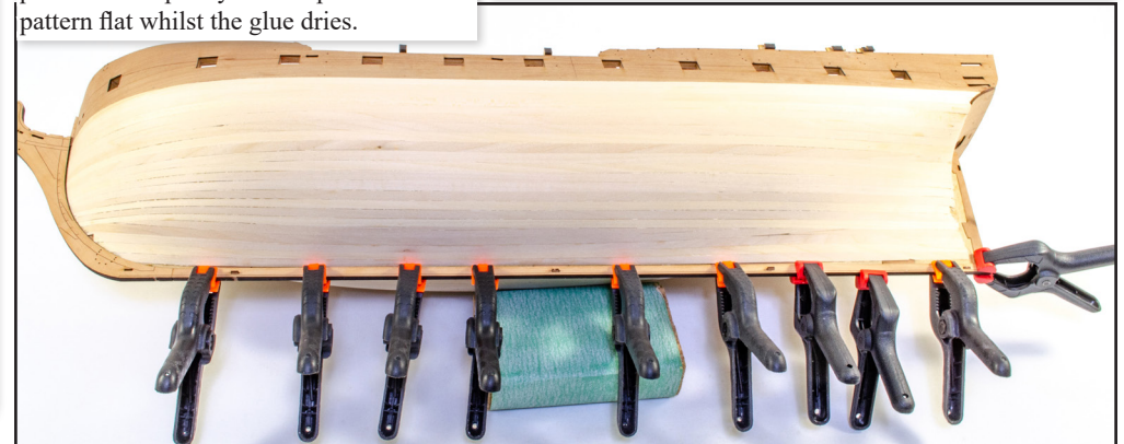
157. The prow outer patterns can now be glued into position, with the pegs helping with alignment. TIP: apply glue to the prow instead of the thin pattern. This will prevent the pattern from curling while you align it. Use clamps to secure in position until set. Do this for both sides.
