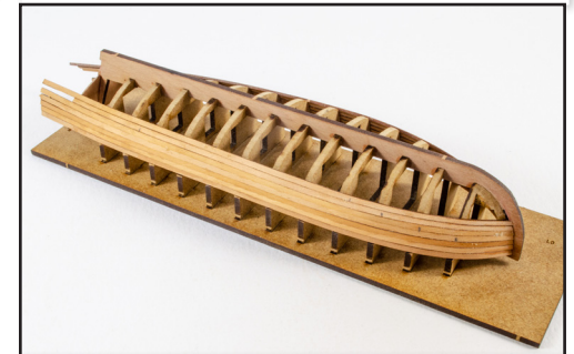
737. Using more 0.6mm planks, continue to plank upwards towards the keel. To get maximum contact to the bulkheads, you will need to taper the planks. The pencil marks seen here are where these were tapered from. Edge-bevelling the planks will allow them to sit snugly together too. You will probably find it necessary to start planking from the keel at some point and meet up with the previous planking.
