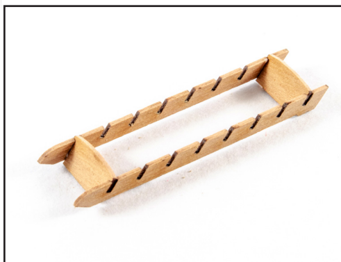
618. When dry, glue the other ladder side into place.
