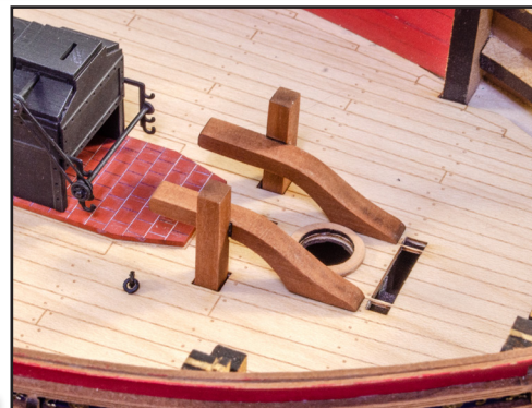
460. Glue into position as seen here, making sure the post supports are on the inside of the posts.
