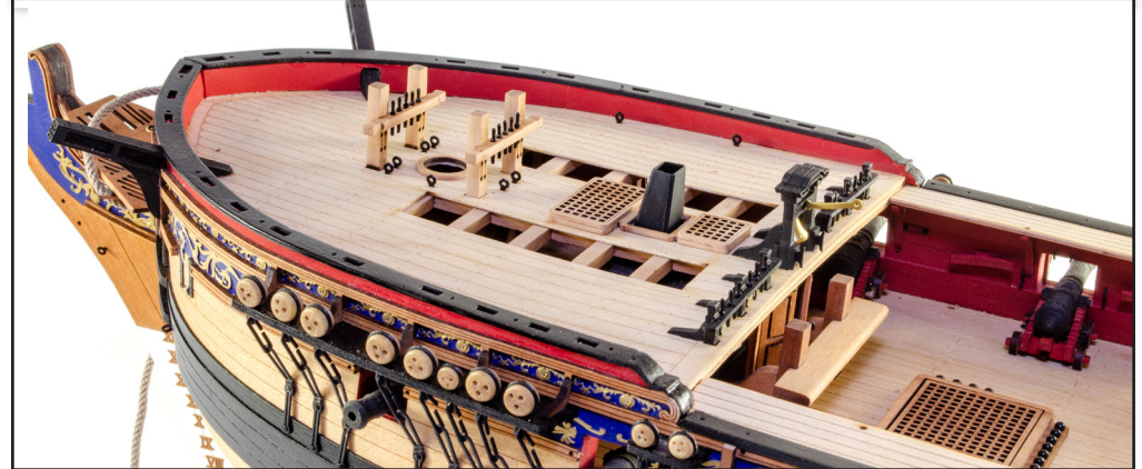
663. Using your plans as reference, fit all deck eyelets (PE-106) and deck cleats (398). Next to the binnacle, fit four eyelets (PE-81). Paint all eyelets black. On the forecandle deck, install the Belaying Pins (PE-152) from the 0.6mm PE sheet. Paint black.
