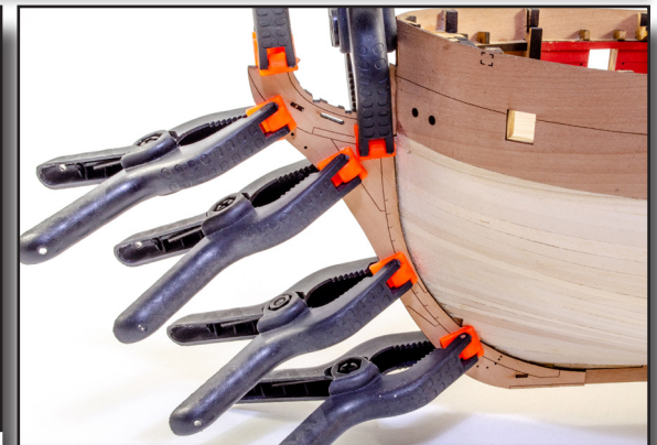
157. The prow outer patterns can now be glued into position, with the pegs helping with alignment. TIP: apply glue to the prow instead of the thin pattern. This will prevent the pattern from curling while you align it. Use clamps to secure in position until set. Do this for both sides.
