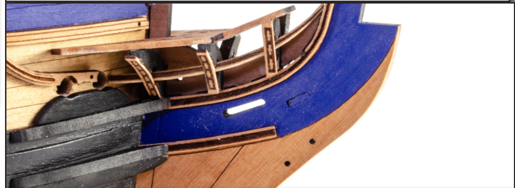
300. Glue the V-shaped head rail patterns into place on the edges of the V-brackets as seen here, trapping the lower rail. You may need to trim the patterns to suit.
