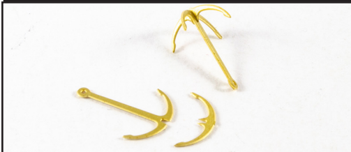
722. Glue the anchor parts together as shown, using CA. You can either paint these black or use a blackening solution.
