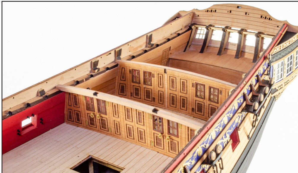
346. Now fit the forward Bulkhead Screen into position. Quarterdeck Beam 458I sits in front of the screen, so the screen can sit flat against it. You can also glue that beam into place at this time.
