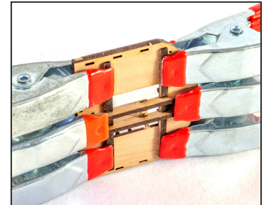
810. Glue the Cross Trees in place underneath the mizzen top platform and clamp until thoroughly set. Check plan for placement.
