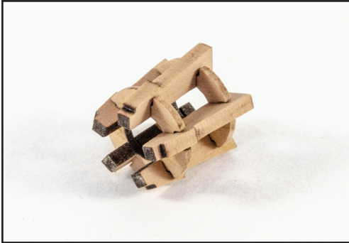
625. Glue the whelps to the checks to create a drum.
