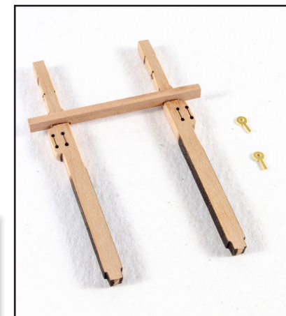
376. Remove char (at least above deck level) and then glue the wooden parts as shown. From the 0.4mm PE sheet, remove two Chain Pump Handle Eyebolts (PE-143).
