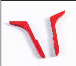
495. Glue Deck Beam 'A' into position. There are engraved marks on both the deck beam and location point which shows where each fit. Beam 'A' will also sit atop the two chain pump handle stanchions as shown.
