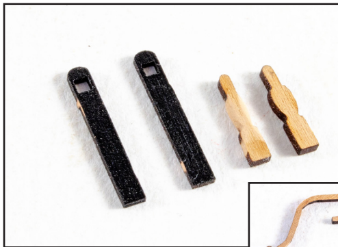
660. From the 1.5mm wood sheet, remove the two Quarterdeck Breast Rail Stanchions – Gangway (407) and sand the curved area to represent a pillar. From the 1mm wood sheet, remove the two Quarterdeck Waist Rail Patterns (153). You can paint these black now if you wish.
