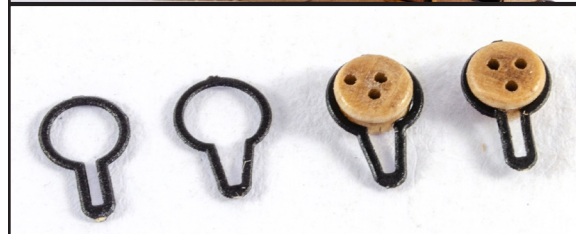
330. Follow the plans and fit the deadeye and chainplate assemblies. If you find a particular part is too long or short for a specific point, try to use another size of the same part. There are no real rules here as long as the result closely resembles what you have on your plan. Use brass pins to hold things into position. You will need to cut these shorter where they fasten to the unpainted hull. On the wales, you can use full length as they are below deck height. Use black paint to cover the brass pins and any parts where brass might show through.
