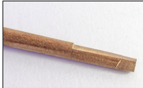
871. Carefully shape the dowel so that the bee will sit flush with the top of the dowel. Shape the front of the dowel at an angle to fit the cap.
