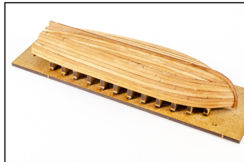
738. Here you can see the completed planking. It's perfectly ok to use infill planks (stealers) to close up any gaps, as these won't be seen below the paint layer. You can see the infill planks in this picture.
