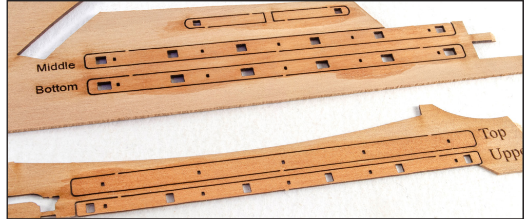
652. Locate the Quarterdeck Breast Beams – Lower/Middle (151/152) on the 1mm wood sheet, and also the Upper Breast Rails – Upper/Top (77/78) from the 0.6mm wood sheet. I have left these in the sheets to help identify during assembly. You can also pre-paint them at this stage for ease but remember the 0.6mm parts only need paint on one side, and the same for the bottom rail.
