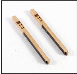
582. From the 3mm wood sheet, remove the two Fore Topsail Sheet Bitts (468). Remove the char.
