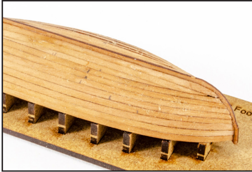
774. Here's another view of the planked hull. Again, you can see the various taper marks and stealers that I fitted.
