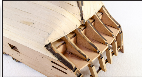
148. Before fitting the lower counter pattern, you can trim the ends of the ply bulwarks, so they are flush with the end stern timbers. Lightly sand the stern, remembering that this area is curved.
