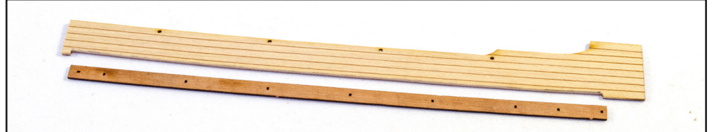
553. Remove the area on the gangway with a knife/sanding paper and test fit the gunwale to it to make sure it fits along the length. Also test fit the two parts to the hull to make sure they go together properly.
