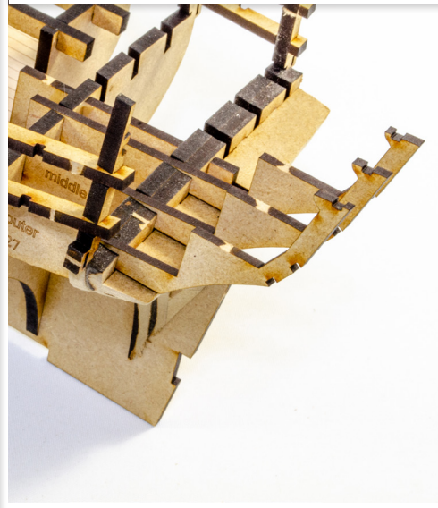
69. Insert the Stern Counter Frame – Outer (27) to the bulkhead slots to the outside of the middle frame. Do this for both sides.
