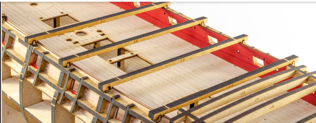
126. From the 4mm MDF sheet, remove parts J-4, J-5, J-6, and J-7. The clip across the top of each bulkhead with the same number (i.e., J-7 across bulkhead #7). Again, do NOT glue these.
