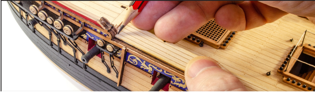
549. Sit the gangway in position (you may need to trim the length slightly) and mark the front and rear positions of where the adjoining gunwale will fit.
