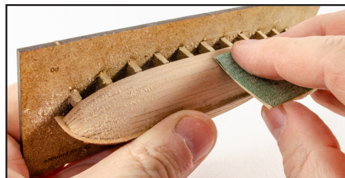
704. Sand the hull using 120 grade paper, finishing it with a finer grade to allow for a good paint finish.
