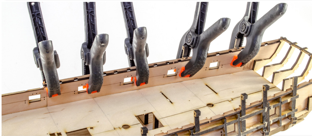
96. You will need to test fit these parts before gluing as some minor adjustment may be needed at the rear of the part, so it sits as shown here. This is part 216. We have left a little extra length here to allow for variation. Once you have the best fit, clamp and then paint in dilute wood glue from the reverse. Repeat with the opposite bulwark, 214.
