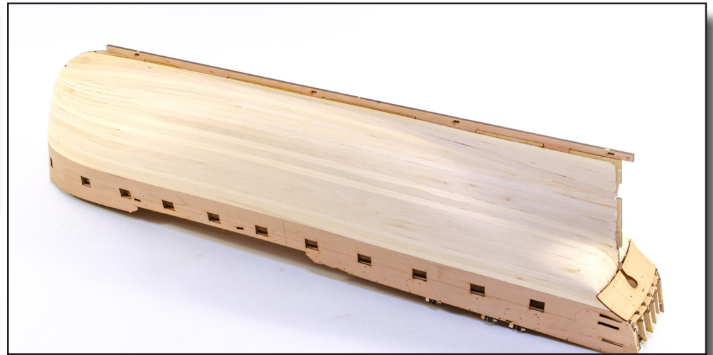
151. Using wood glue, glue the Keel Pattern into place on the underside of the hull. This can only fit one way around due to the tabs. Leave to set.
