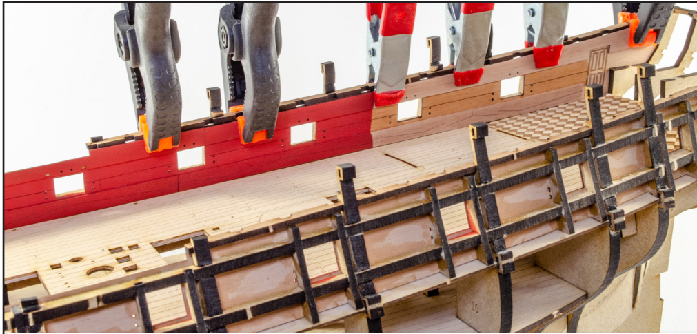
111. Now glue the Deck Clamp Pattern – Rear (111) into position as shown, again leaving the upper edge slightly higher than adjacent bulwark. The top edge of this will fall more or less directly under the quarterdeck beams that sit over the rear bulwarks.
