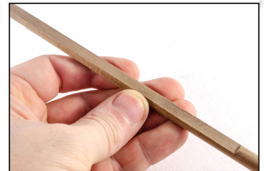
855. Create the flats on the lower mast section, taking dimensions from the plans. Also create a subtle flat running down the front of the mast, as shown on plan.
