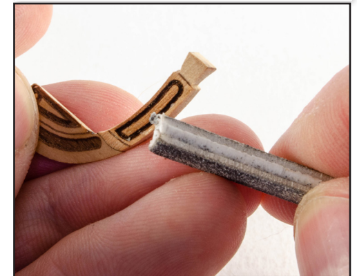
678. Carve/Sand the top of the rail timberhead as shown.
