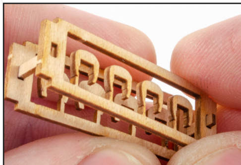
884. Take the sprue with no engravings. These parts are slightly smaller in size. Glue into position over the previous, using the keys to align.
