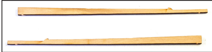
541. Glue and clamp in place as shown. We recommend you slightly bevel the rear edge, so it sits against the stern with no gap.
