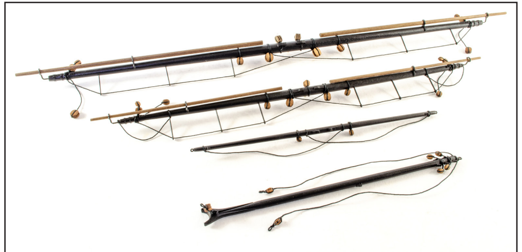
881. Paint all yards in black and fit them out with blocks etc. as shown on plans.
