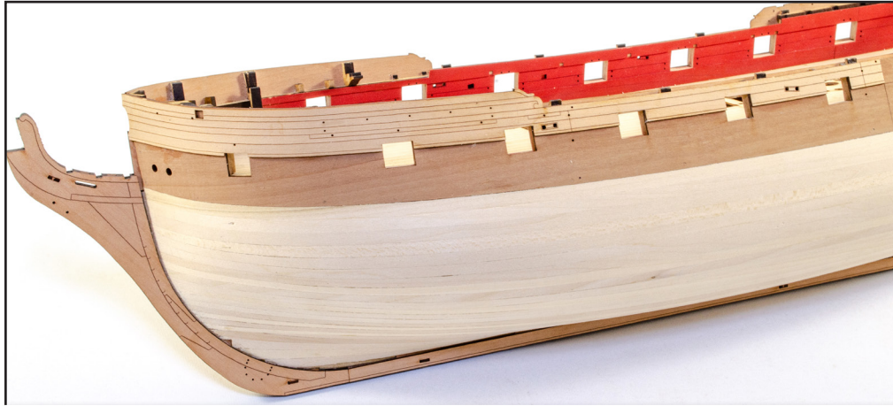
165. Both patterns can now be glued to the hull. TIP: We suggest using diluted white glue, applied to the hull and not the pattern. If applied to the pattern, you will find it curls, making it harder to fit. You may need to slightly adjust the pattern to fit your model by sanding a little from the front edge. Test fit to ensure best fit first.
