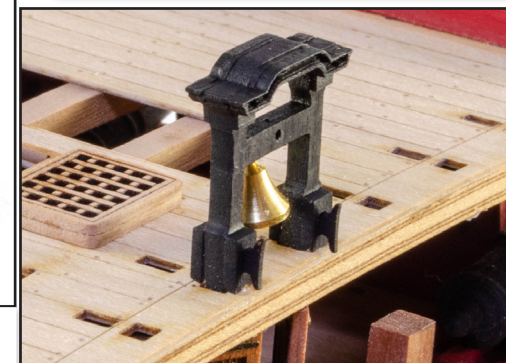
597. Mount the belfry to the forecastle deck as shown, with the cleats pointing aft.
