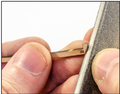
511. To fit deck beam 'RF', you will need to bevel the ends of the beam to fit within the curved bow.
