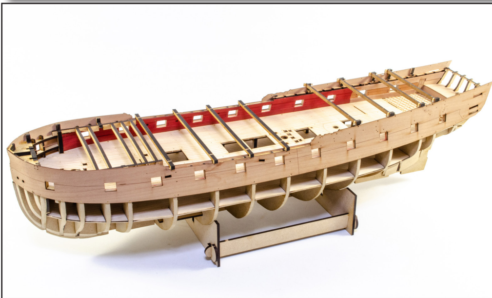
137. Once fitted, leave the parts to dry for a few hours. Notice the jigs are temporary fitted to maintain the width of the hull.
