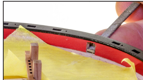
610. The holes in the bulwark are deliberately left smaller than required for alignment and part integrity when assembling. You will now need to open these up to fit the catheads. Use small files and a sharp, narrow blade to open these up to size. For an indication, the inner bulwark will have the hole cut down to deck height, and on the outside hull, the hole will extend up to the gunwale. Use tape to protect the deck whilst you work.
