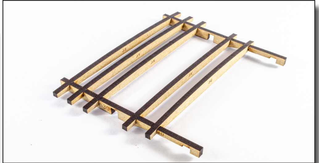
124. You can assemble and glue the jig using the parts you just removed though. Each slot in #30 is labelled for the appropriate jig part.
