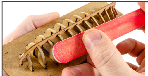
698. Use sandpaper or sanding sticks to sand/fair the bulkheads so that a plank will lie across them with maximum contact.
