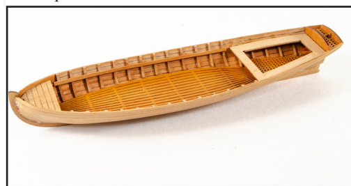
713. From the 1mm wood sheet, glue parts P16 and P24 into position in the bow and rear of the boat.
