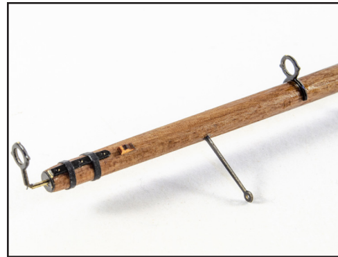
880. YARDS, GAFF etc: Make up all yards as per plans and don't forget the spritsail yards on the Mizzen/Bowsprit plan sheet. You can use either a cut-off brass pin to secure the yards to the masts, or brass wire. For the prototype, we have used the thicker wire option.
