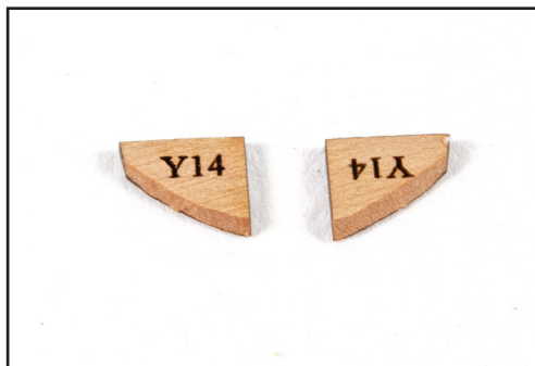
766. Cut both parts Y14 from the 1mm wood sheet and bevel the outer curved edge as shown here. This bevel is only a rough guide as it will be bevelled more soon.
