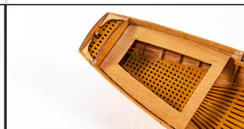
714. From the 1mm wood sheet, glue the knees P25 into place as shown.
