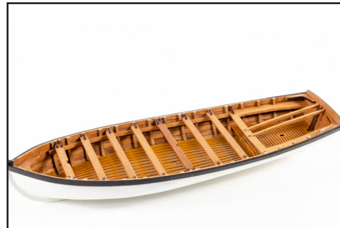
750. Mark a waterline on the hull and paint the lower area white. Take two planking strips and paint those black. Glue them into position so they are level with the upper bulwark. Bend and glue the mast support brackets into position and paint black. Also fit the eyebolt and paint black.
