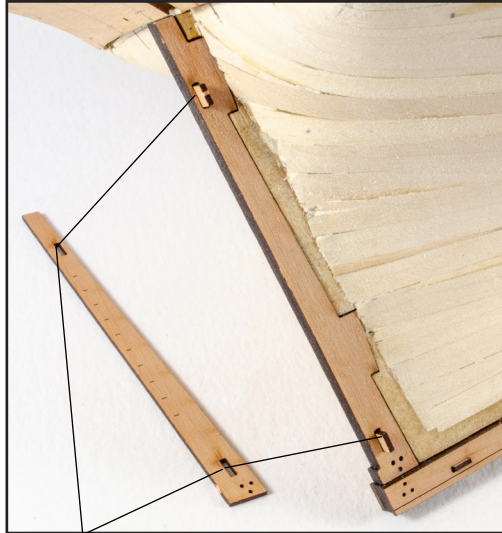
160. Using two more location pegs which are first slotted into the rudder post, glue the rudder post outer patterns into position. You will notice these will only fit one way. Clamp until dry.
