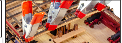
516. Glue this in place centrally on forecastle deck beam 'Z', so it's flush with the top of the beam. You may need to trim each end of this to fit your specific hull.
