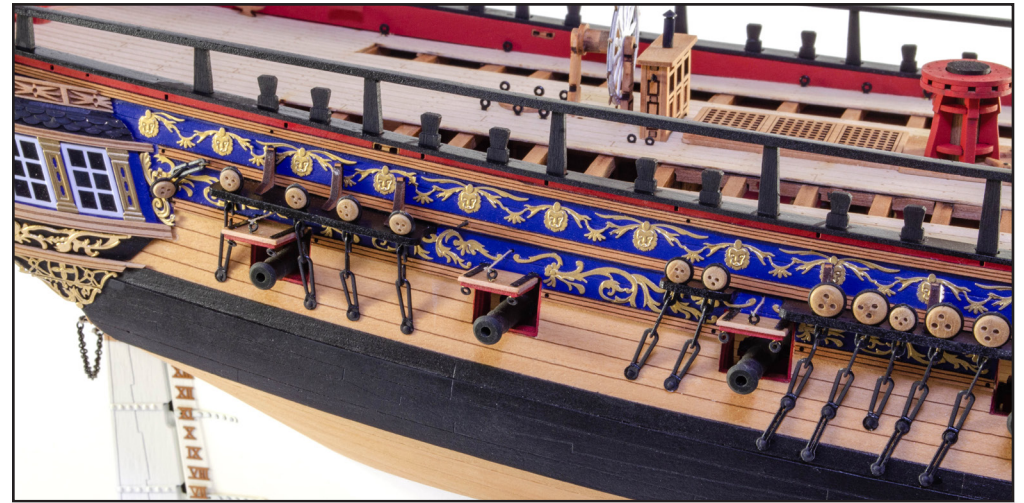
682. Add a short length of 0.1mm natural thread to the upper hole above each of the three rear gun ports. Glue the gun ports into place, checking that the lid is the correct one with the engraved planking patterns, and then tie the other end of the thread to the outside eyebolt. Seal the thread and cut off at eyebolt.
