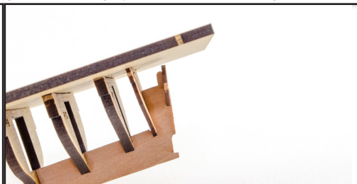
697. When P13 is glued into position, it should be at the same angle as the stern angle of the keel, and flush with it.
