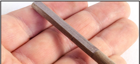
813. The mast sections will go through a number of shape changes to their cross section. Here you see the upper area of the lower section, squared-off on one side to fit the cross trees.
