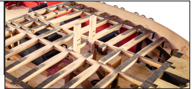
523. Slot and glue the Fore Jeer Bitts through the hole in the gun deck and down into the lower deck where it will plug. The engraved slots for the beam should face aft. NOTE: Early batches of Sphinx have a slot in the gun deck that will need opening a little wider so that it's the same width as the maple deck.
