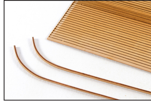
734. If you decide to soak the first planks to bend them, make sure you allow them to thoroughly dry before fitting them.
