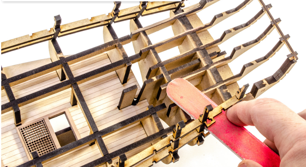
72. Before you attempt to fit the gun deck, sand the horizontal faces of the Stern Counter Frames you just fitted so they flow with the longitudinal deck beams.
