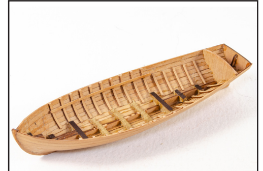
781. On the forward ribs, use a pencil to add a mark 3mm down from the top of the bulwark. Cut the seat support strips (Y29) from the 0.6mm wood sheet. Add a strip to both the internal sides of the hull, as shown.
