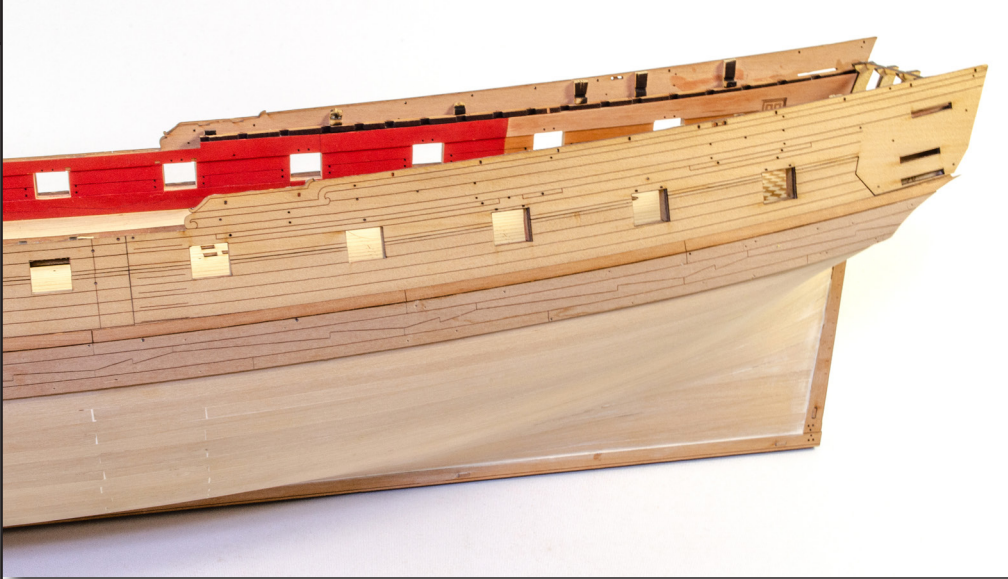
193. Now glue part 72 next to this, along the top of the main wale. When complete, glue parts 73 & 74 on the left side of the hull, in the same manner. Trim down the rear of these parts so they are flush with the stern counter curve.
