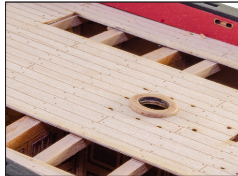
633. From the 1mm wood sheet, remove a Mizzen Mast Base. Sand the upper edges slightly round and glue into position. Note this hole is elongated for the mast rake, and that should run fore to aft.
