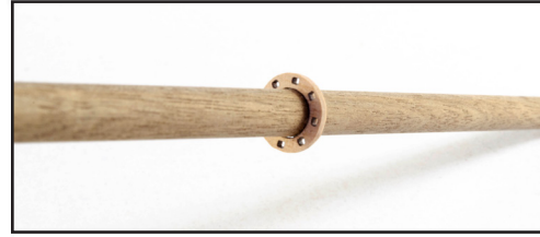
826. From the 1mm wood sheet, glue the Mizzen Belaying Pin Ring (246). You can now paint the belaying pins (PE-152) from the 0.4mm PE sheet, and fit them into the holes.
