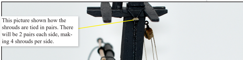
138. Using plan sheet 8 as reference, rig the shrouds as shown. Inset picture above shows the 3.5mm deadeye secured to the shroud
