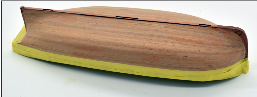
56. Second planking complete, sanded and filled. To get to this stage, several filling and sanding sessions were required. The filler used is a water based type, so it can be diluted and thinned, so it is able to flow into every gap. Before the sanding and filling process started, the engraved upper bulwark patterns were removed and the areas not to be painted white masked off, as can be seen.
