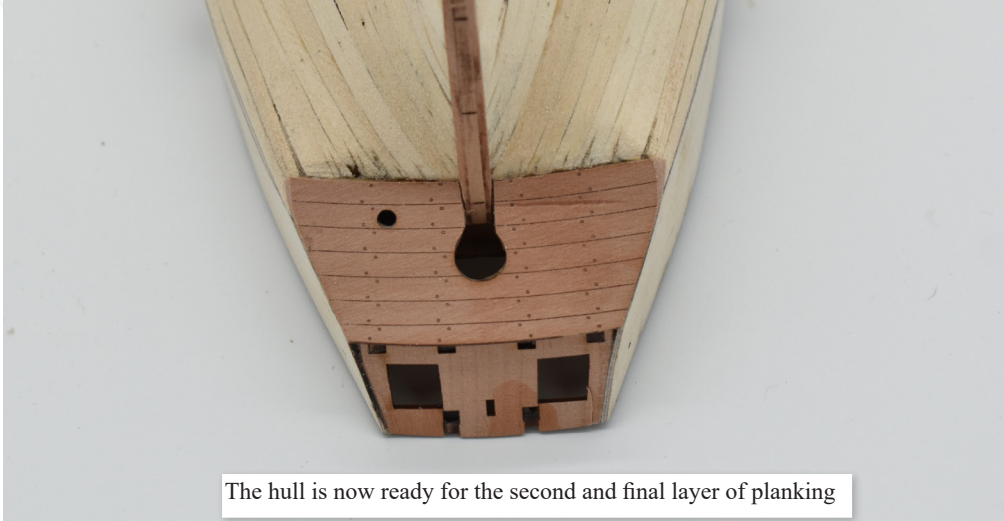
51. Once firmly fixed in place, sand the edges of the stern counter flush with the hull sides.
