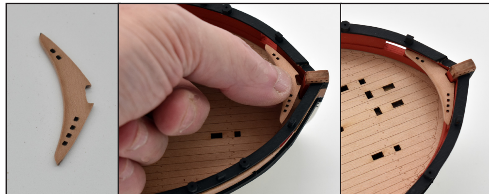
91. Remove part 37, the bow knee, from the 2mm wood sheet. Trial fit and file/sand as necessary so the contact edge sits as flush as possible to the inner bow. Note the orientation of the belaying pin holes, there are 2 on the left side, as the bowsprit covers the rest of the area, and 4 on the right side.
