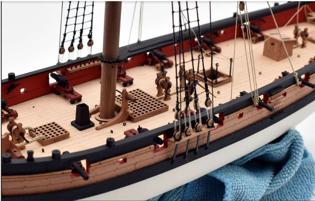
147. Two pictures showing the 2 breast backstays per side. The lower ends are secured around the first and last lower deadeye for the shrouds, and then taken up through the hole located near the end cross-trees and then tied to the topmast head, at the cleat positions.
