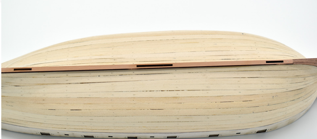
48. The main keel (33) can now be added. Pin as well as glue into position, making sure the slots for the drop keels line up with the slots in the hull
