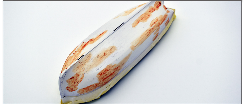
57. The hull is sprayed white using a standard spray can from any DIY outlet. Above shows the first three light coats. You will notice gaps in between the planks, despite sanding and filling previously. This is normal. Below shows another covering of filler, before sanding smooth. This process will need repeating several times until all gaps are eliminated. (Pre-cut holes in keel were blocked off using brass pins during this process)
