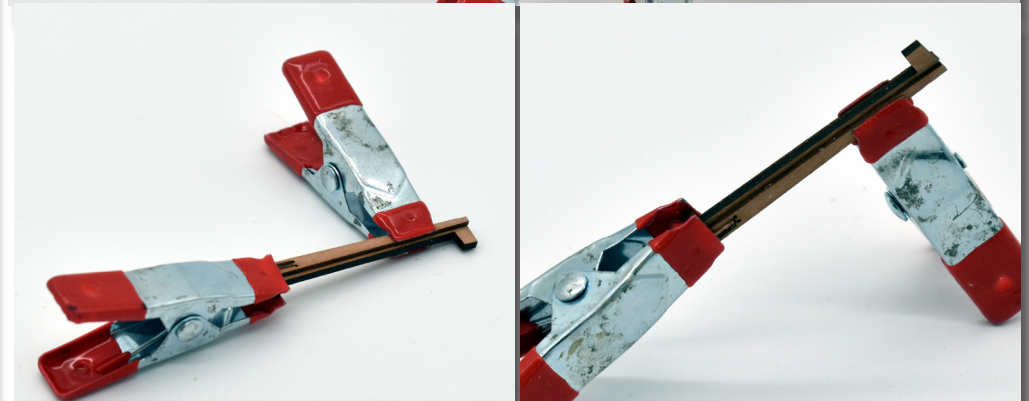
47. Make up the stern/rudder post assembly using part 32 at the core, and parts 95 for the outer rabbit parts. Glue and peg using K-3 the parts together and clamp until set, as shown.
