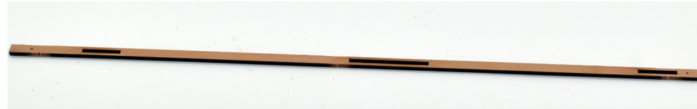
48. The main keel (33) can now be added. Pin as well as glue into position, making sure the slots for the drop keels line up with the slots in the hull
