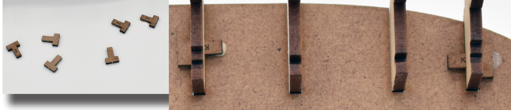
15. Remove the lower deck securing keys (K-2) and slot and glue into place on bulkheads 3, 6 and 9. These will ensure the lower deck is locked into place.
