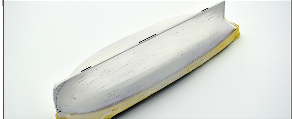
57. The hull is sprayed white using a standard spray can from any DIY outlet. Above shows the first three light coats. You will notice gaps in between the planks, despite sanding and filling previously. This is normal. Below shows another covering of filler, before sanding smooth. This process will need repeating several times until all gaps are eliminated. (Pre-cut holes in keel were blocked off using brass pins during this process)
