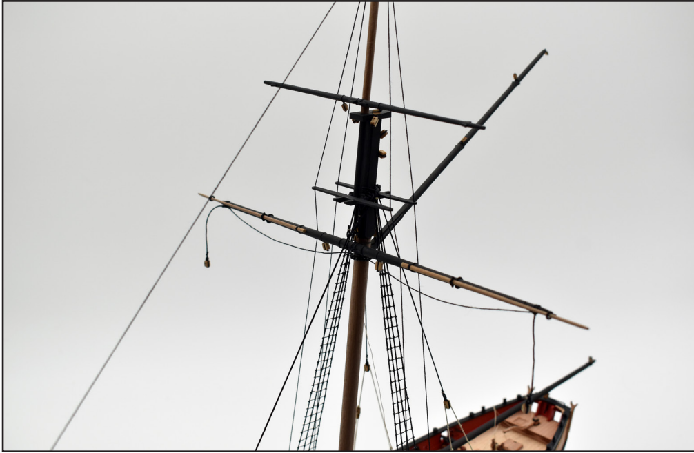
147. Two pictures showing the 2 breast backstays per side. The lower ends are secured around the first and last lower deadeye for the shrouds, and then taken up through the hole located near the end cross-trees and then tied to the topmast head, at the cleat positions.
