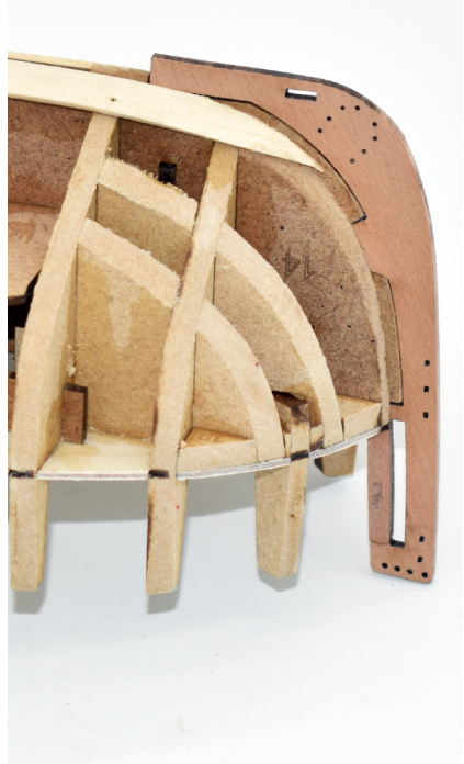
42. Glue the prow in place using PVA wood glue
