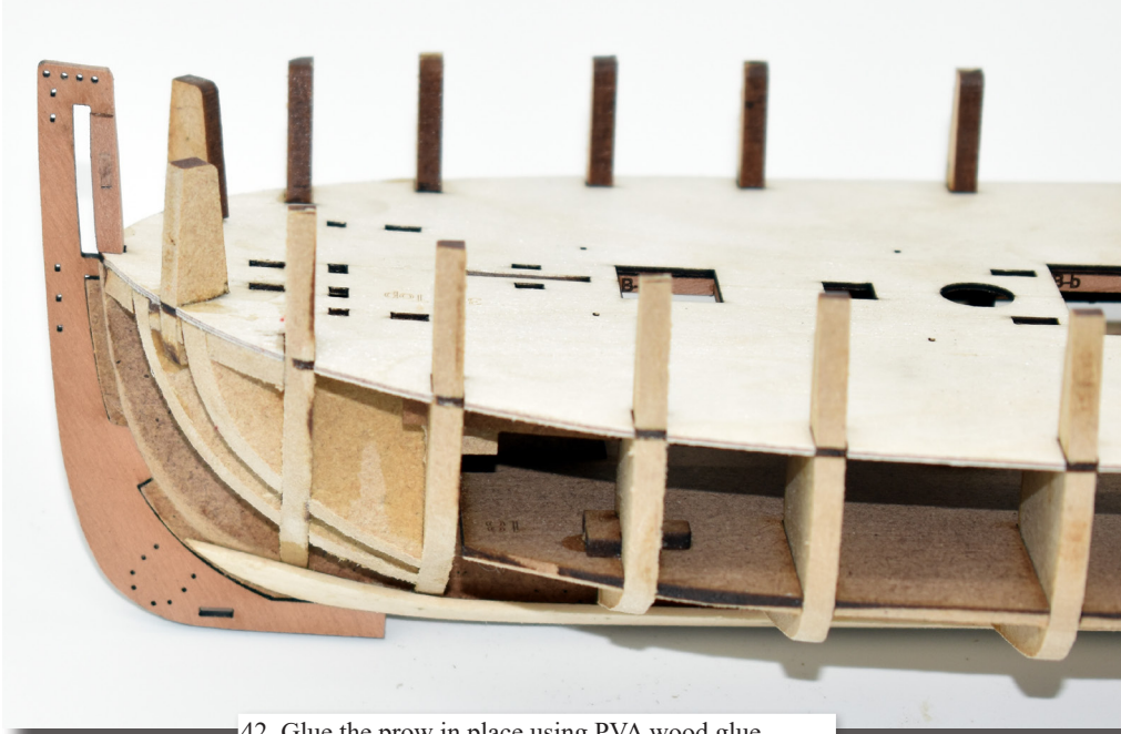
42. Glue the prow in place using PVA wood glue
