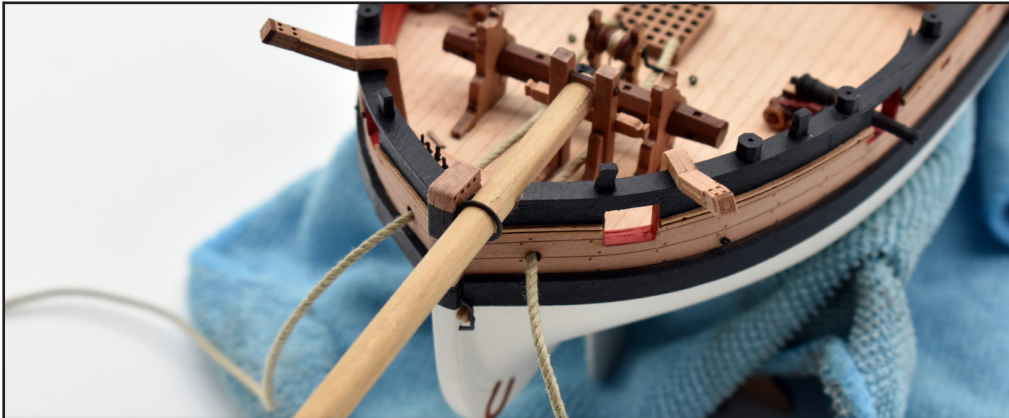
130. Once the bowsprit has been shaped as per the plan, you can now slot and insert into place. the very end fits in between the bowsprit bits.
