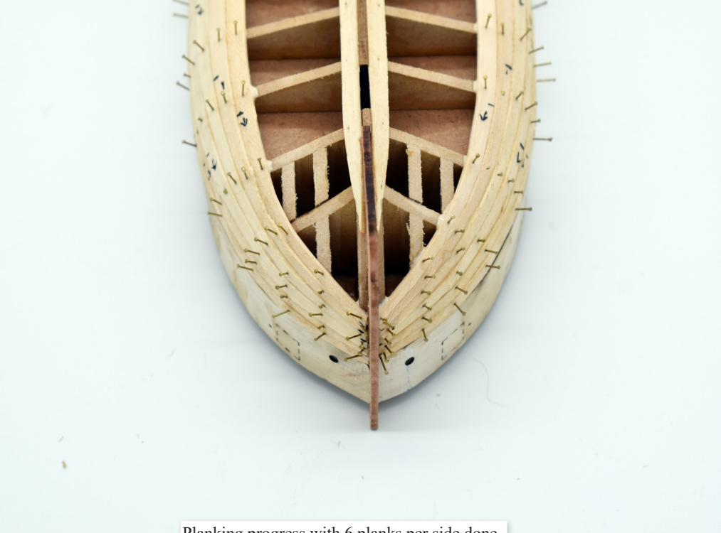
Planking progress with 6 planks per side done
