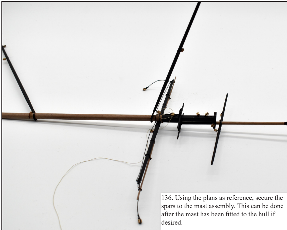
Add the parrel beads to both main and driver boom jaws, ready to be secured to the mast.
