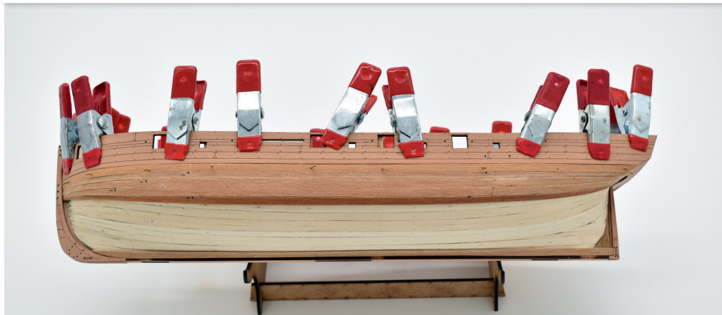
As with the first planking, the planks require tapering at the front (as shown above) Below - The first 4 planks laid.
