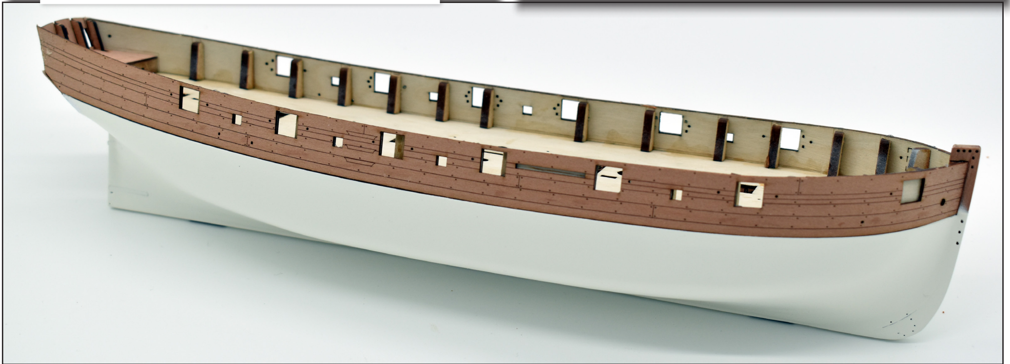
61. After 24 hours, remove the clamps. The bulwarks should now be firmly in place
