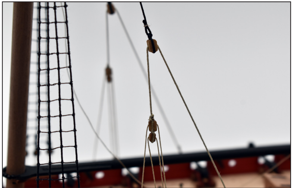
142 - These 2 pictures show the back stay rigging detail
