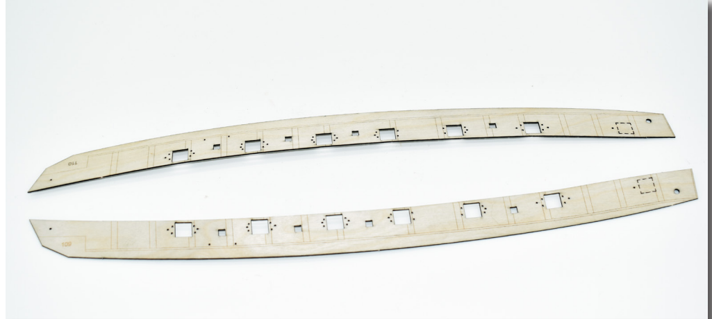
44. The two bulwark 0.8mm ply patterns can now be added (49 - left/port and 50 - right/starboard). The engraved vertical lines should follow quite closely the bulkhead positions, and the lowest horizontal line should be placed at the top edge of the false deck position. We recommend that these parts are dry fitted several times to ensure correct positioning. Each engraved line may not be a perfect match to each bulkhead tab due to slight variations in the sanding of the bulkheads process. However, if they more or less match from front to back, this will be fine. Always watch for the lower deck line along the deck edges.
