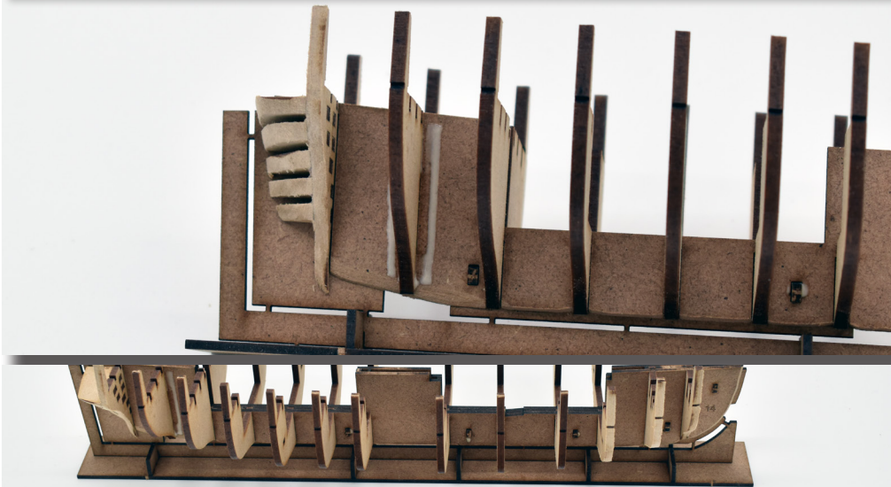
12. The final bulkheads can now be fitted. Remove both halves of bulkhead 12 and add glue as shown. Do not add glue to the slot, as there is a chance some glue will entre the slot for the drop keel.
