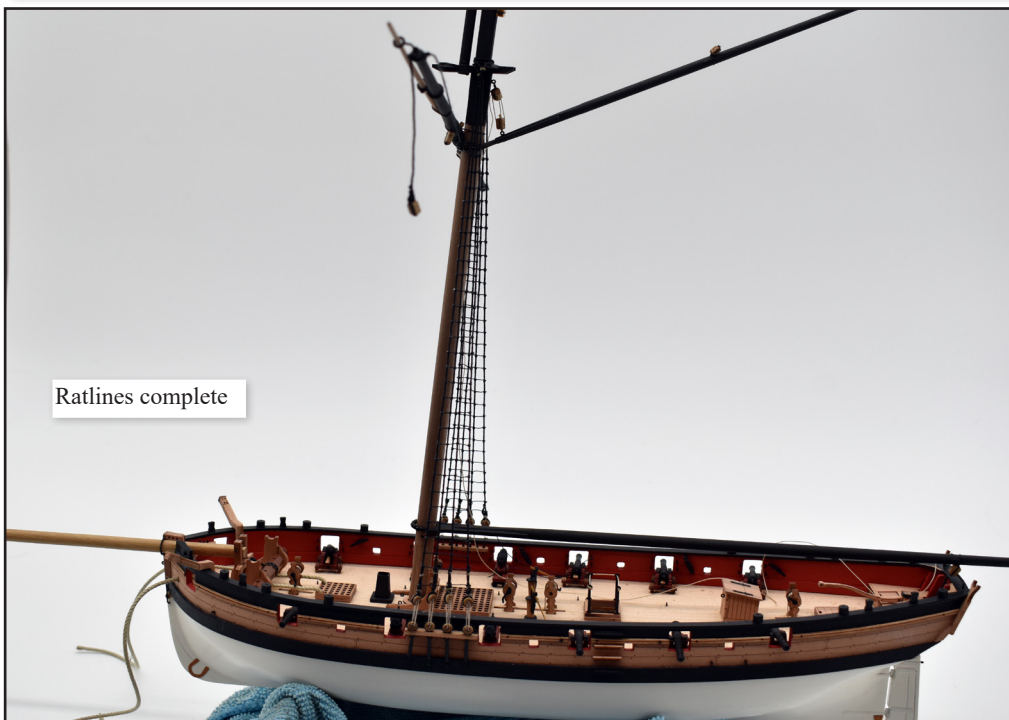
140. Once the ratline are complete, use some good quality cutters to snip the extra cord from each ratline.
