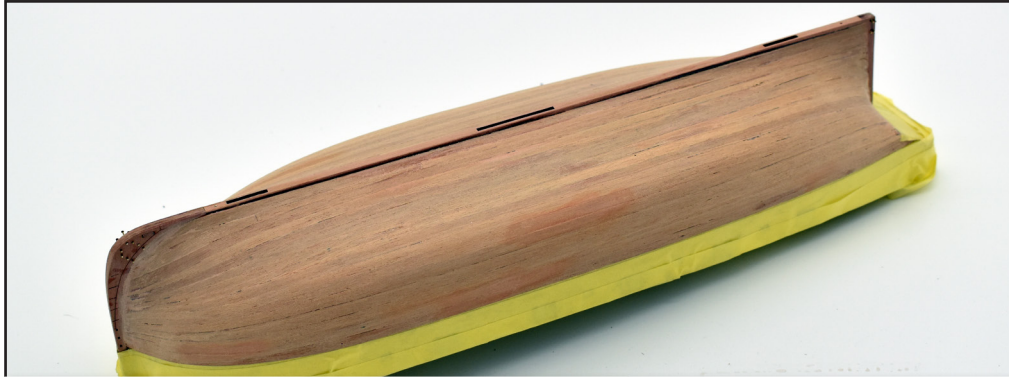
56. Second planking complete, sanded and filled. To get to this stage, several filling and sanding sessions were required. The filler used is a water based type, so it can be diluted and thinned, so it is able to flow into every gap. Before the sanding and filling process started, the engraved upper bulwark patterns were removed and the areas not to be painted white masked off, as can be seen.
