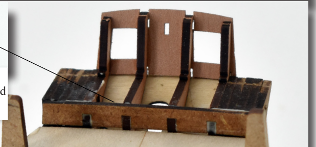
36. To further strengthen the hull assembly, you can brush on watered down PVA wood glue under the lower and upper decks.
